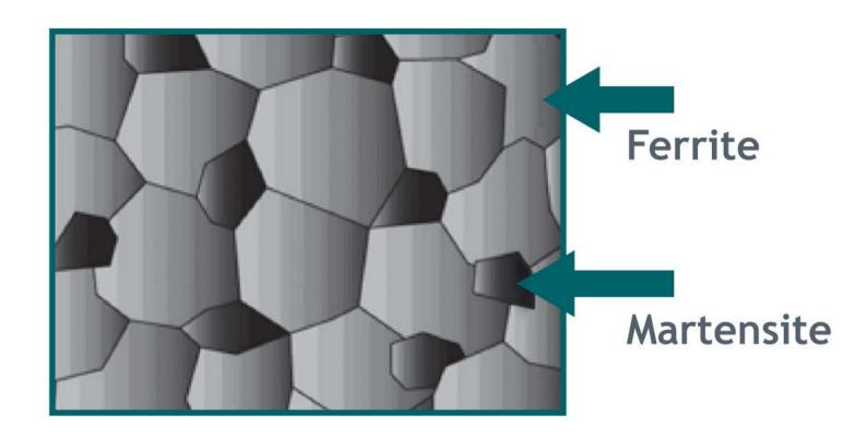
Example of a microstructure of a dual phase steel, showing the martensite (dark) and ferrite (light) phases
