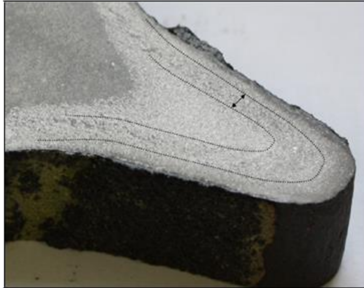
Figure 7. Carbide enriched layer with ribbon containing less carbide.
