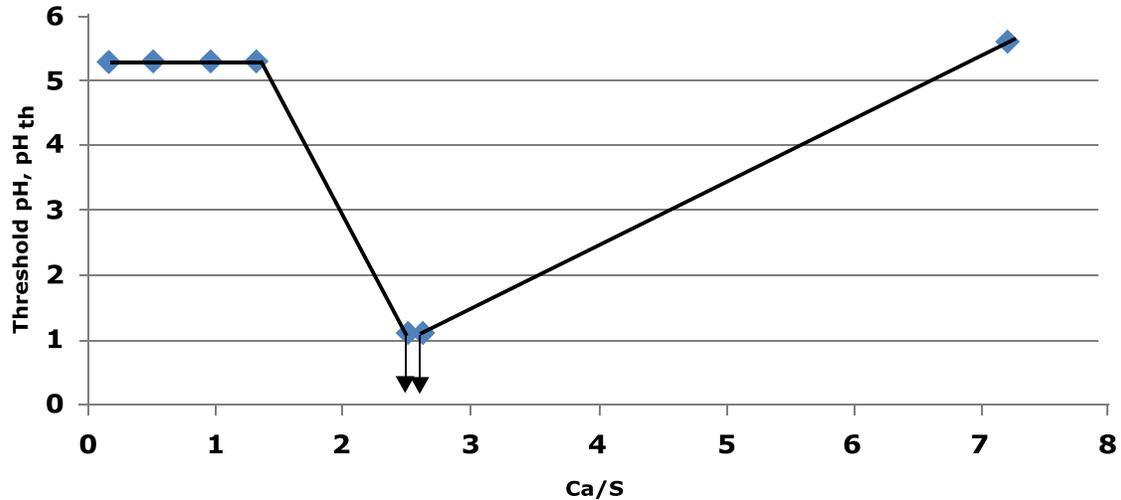
Figure 7. Correlation between threshold pH and Ca/S ratio.
