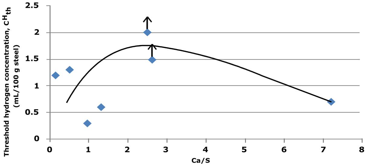
Figure 6. Correlation between threshold hydrogen concentration and Ca/S ratio.
