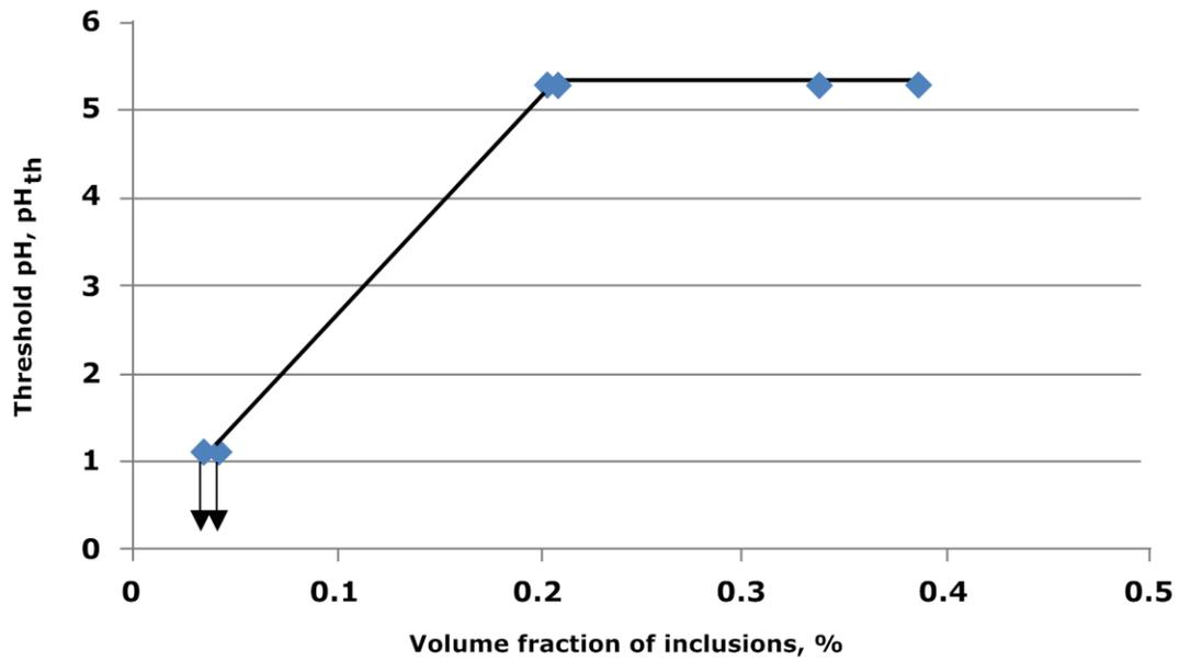
Figure 4. Correlation between threshold pH and volume fraction of inclusions. Arrows pointing downward identify steels that did not crack under the most aggressive conditions of this study, ie. pH 1.1, so that  $pH_{th} < 1.1$  for these steels.
