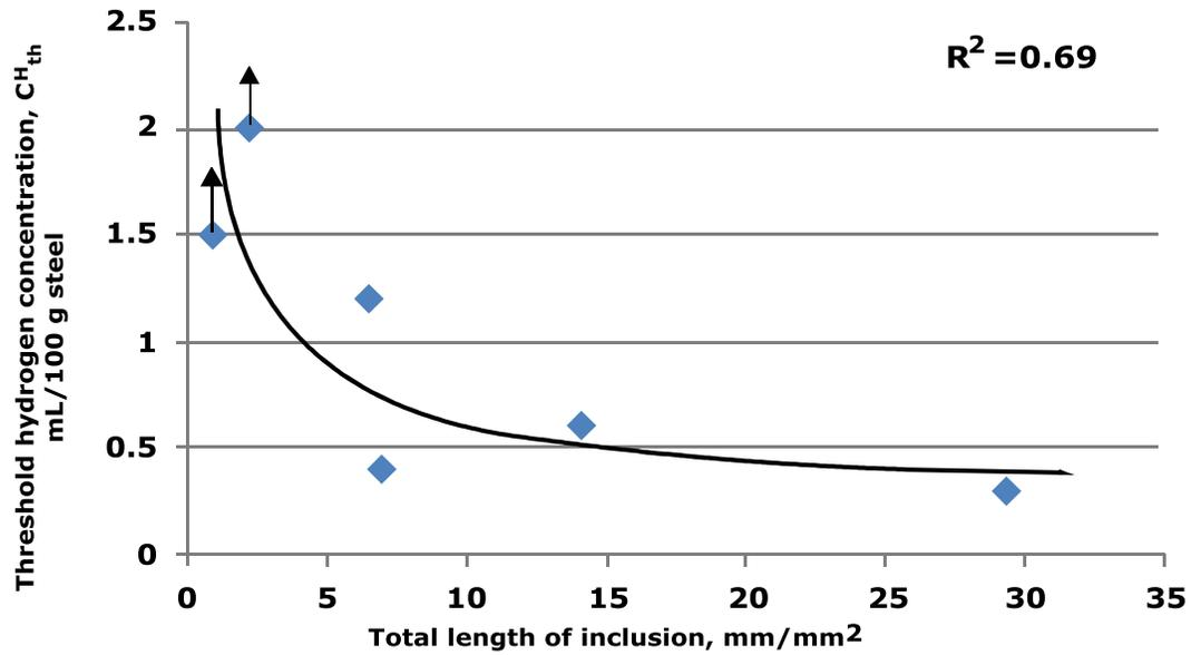
Figure 3. Correlation between threshold hydrogen concentration and total length of inclusions.
