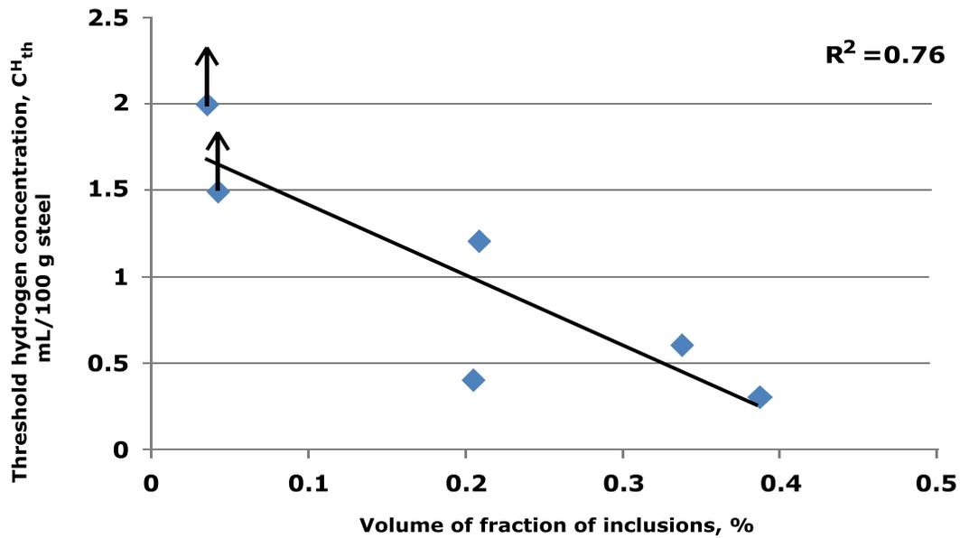
Figure 2. Correlation between threshold hydrogen concentration and volume fraction of inclusions. Arrows pointing upward identify steels that did not crack at the highest quantity of  $C^{\text{H}}$  that was measured; i.e.  $C_{\text{th}}^{\text{H}}$  for these steels exceeded these values.
