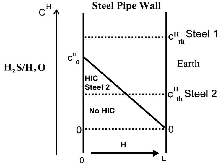
Figure 1. Model indicating significant parameters in occurrence of HIC and criterion for HIC.
