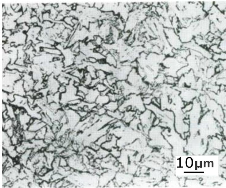
Figure 9. Photomicrograph of steel CTR-2 showing uniform microstructure [9].
