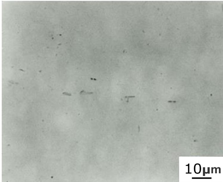
Figure 10. Photomicrograph of steel CTR-1, showing Nb-rich precipitates [9].
