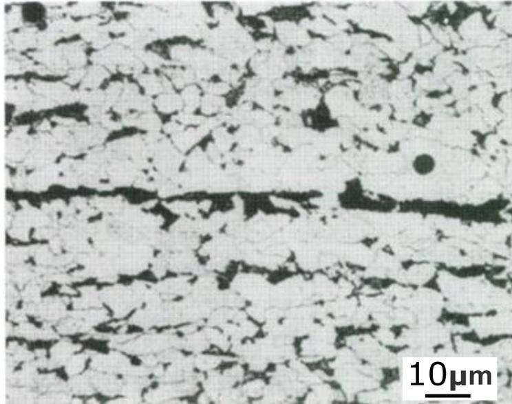
Figure 8. Photomicrograph of steel CTR-1 showing banded microstructure [9].
