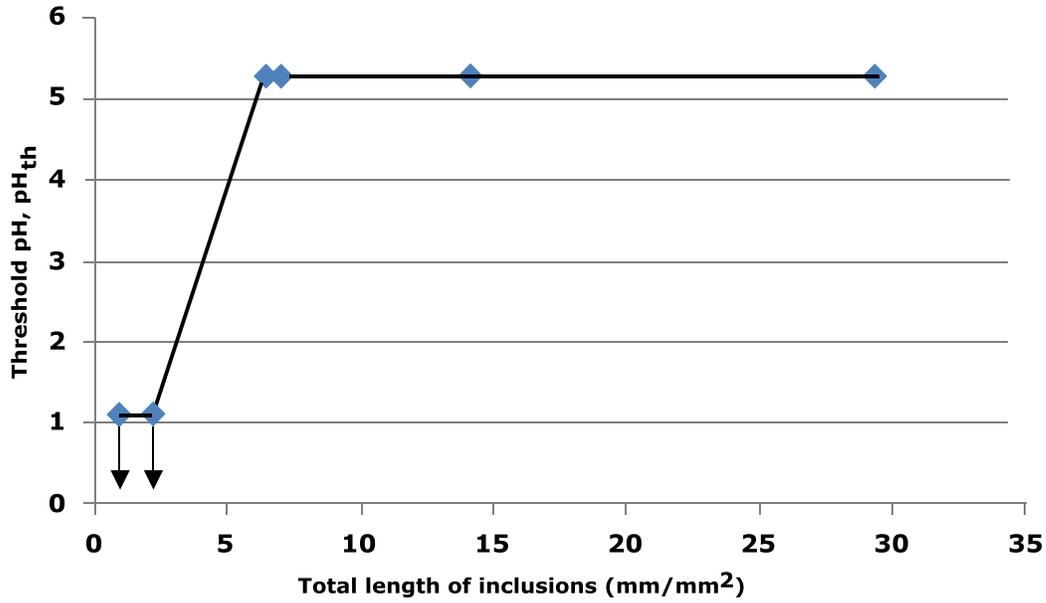
Figure 5. Correlation between threshold pH and total length of inclusions.
