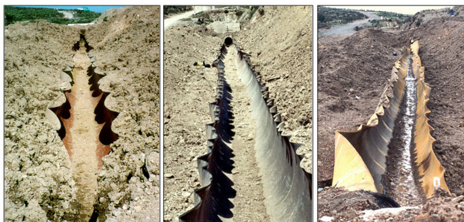
Figure 5. CSM's full-scale tests on X100 lines. View of the fractured lines.
