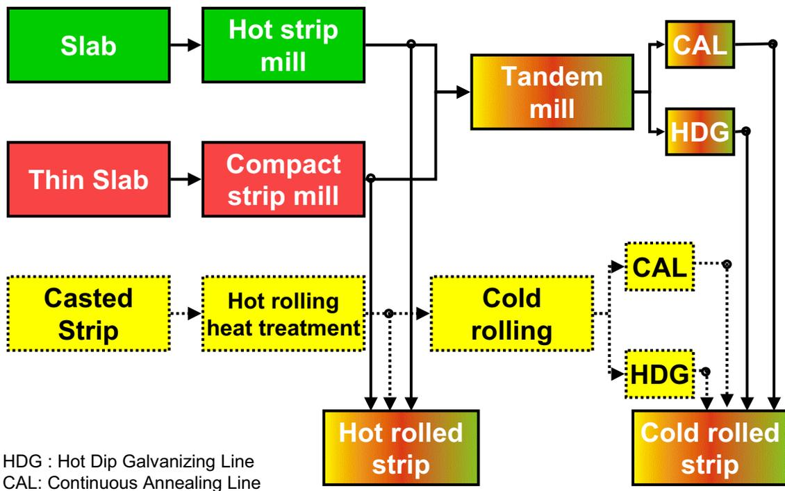
Figure 14. Process routes for hot and cold rolled steels.
