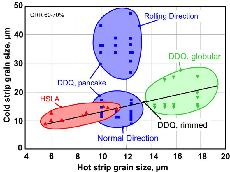
Figure 12. Relationship of hot strip and cold strip grain sizes for batch annealed steels.
