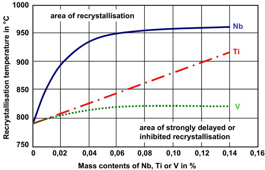
Figure 6. Influence of Nb, Ti and V on the threshold temperature of austenite recrystallization.
