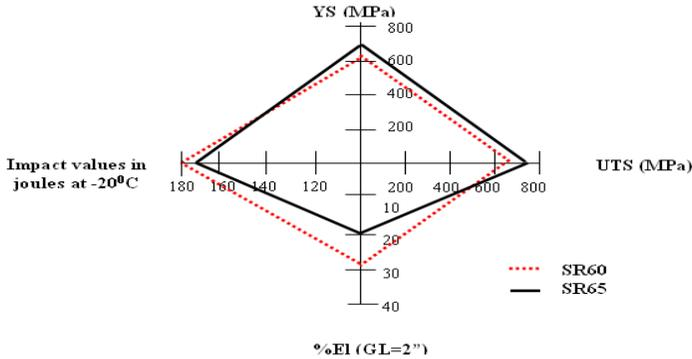
Figure 5. Comparison of typical mechanical properties of SR60 and SR65 grade steel.
