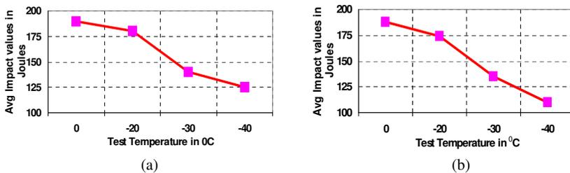
Figure 7. Impact energy transition curve for a) SR60 and b) SR65.
