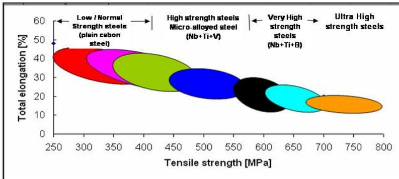
Figure 1. Overall view of hot rolled steel grade made at Essar in different strength level
