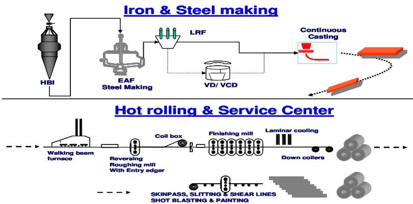
Figure 2. Process flow chart at Essar Steel
