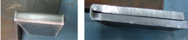
Figure 6. Close bend specimen in grade SR65.
