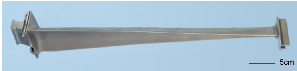
Figure 2. A photograph of a large low pressure turbine blade that is being qualified for a next generation commercial aero engine. After many programs and extensive alloy and process development by many companies and organizations, this alloy class is now seeing applications within several aero engines.
