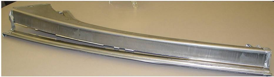
Figure 2. DP800 stamping exhibiting shear fracture.
