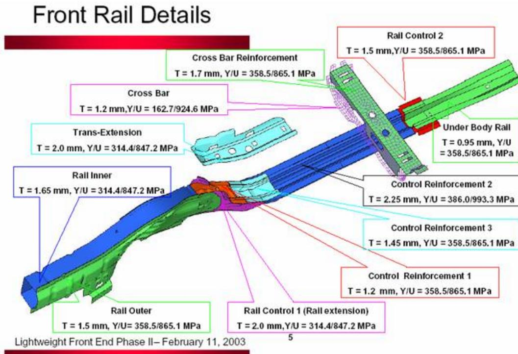
Figure 1. Front rail design from Auto Steel Partnership Lightweight Front End Structure Project – All components are Dual Phase steel. Target mechanical properties shown.
