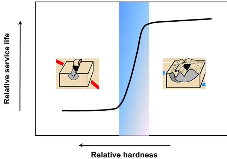
Figure 5. Prevailing wear regimes with respect to the relative hardness.
