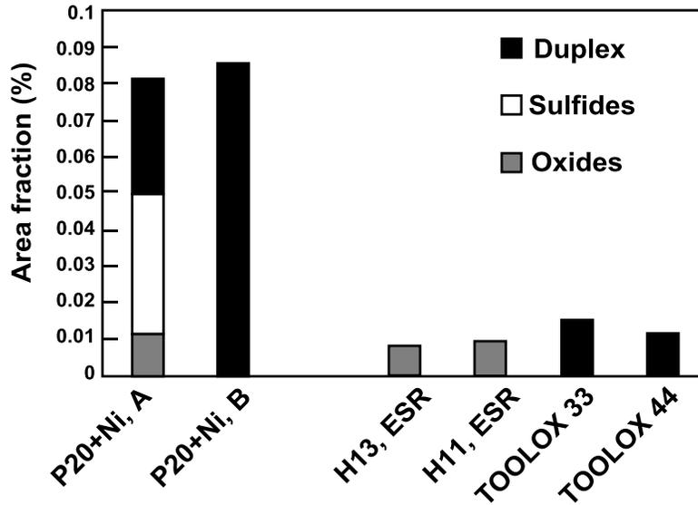
Figure 3. Steel inclusion contents, plate centre position.
