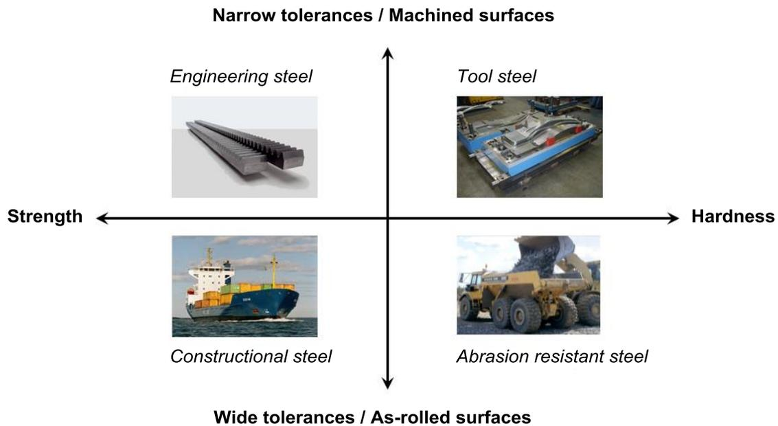
Figure 1. Common steel grade application areas.
