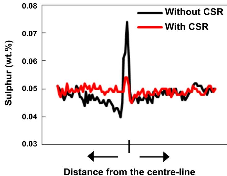
Figure 2. Sulphur segregation at slab centreline.
