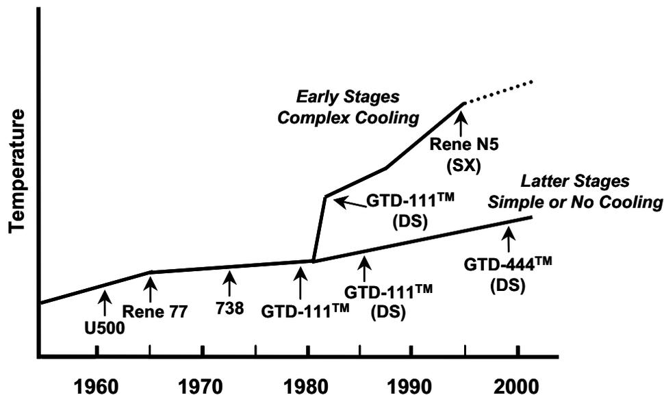
Figure 1. IGT bucket alloy evolution showing increase in temperature capability.
