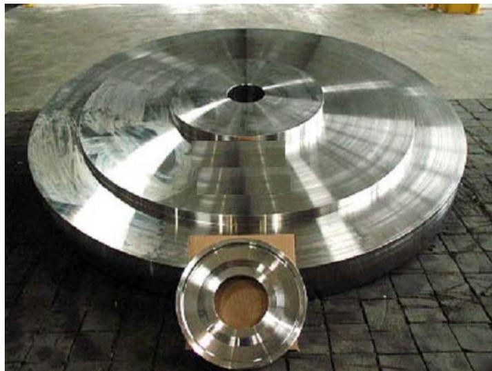
Figure 5. Size comparison of an IGT first stage wheel forging (machined to sonic inspection shape) with a typical aircraft engine turbine disk forging.
