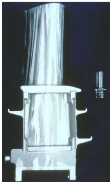
Figure 2. Size comparison of an IGT first stage bucket with a typical aircraft engine turbine blade.
