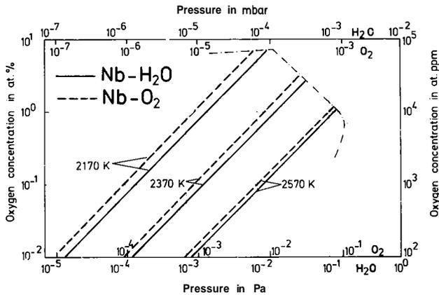
Figure 3 - Steady states for niobium in O<sub>2</sub> and H<sub>2</sub>O atmospheres.
