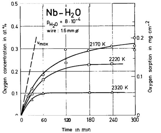
Figure 2 - Increase of O concentration with time for niobium in H<sub>2</sub>O atmosphere.
