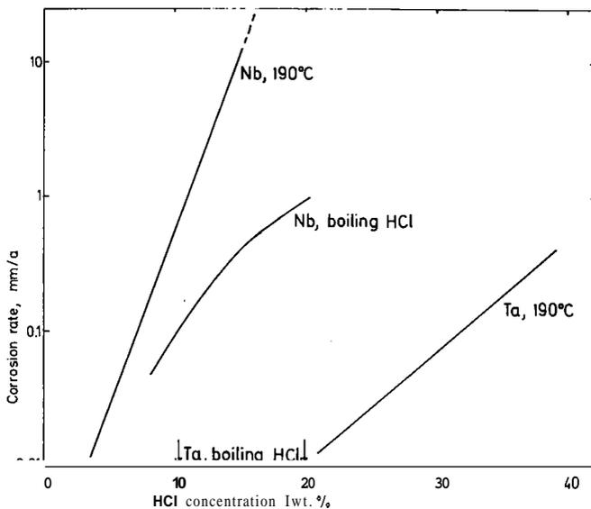
Figure 9 - Corrosion rates of niobium and tantalum in HCl (41).
