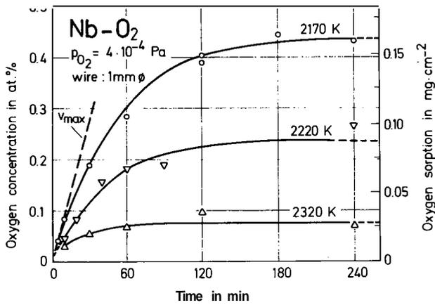
Figure 1 - Increase of O concentration with time for niobium in O<sub>2</sub> atmosphere.
