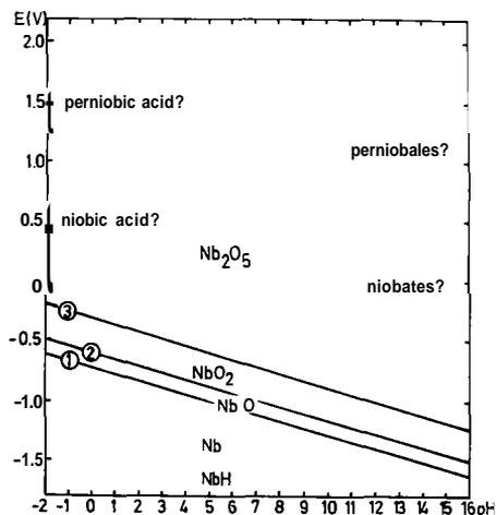
Figure 4 - Potential - pH diagram for the system niobium - water at 25 C (26, 27).
