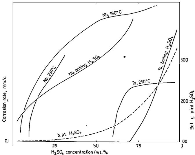
Figure 5 - Corrosion rates of niobium and tantalum in  $H_2SO_4$  (41).
