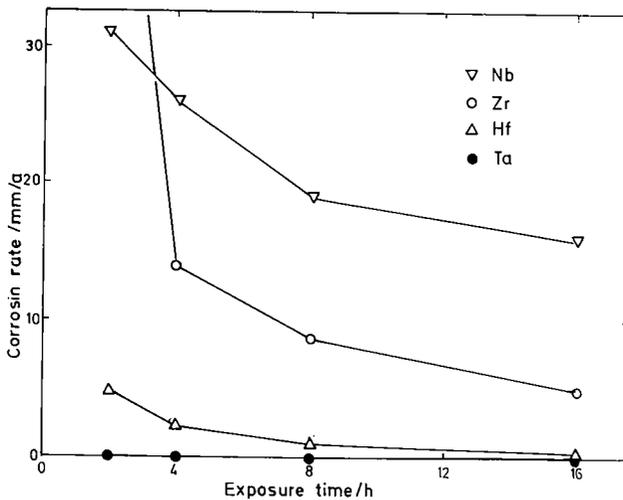
Figure 6 - Corrosion rates of niobium, zirconium, hafnium and tantalum in boiling 75 %  $H_2SO_4$  (185°C) (42, 43).
