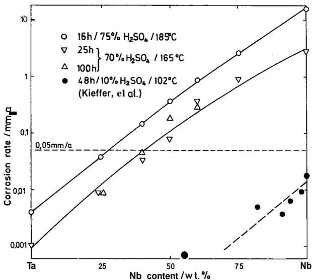
Figure 8 - Corrosion rates of Nb-Ta alloys in boiling  $H_2SO_4$  (37, 42, 43).
