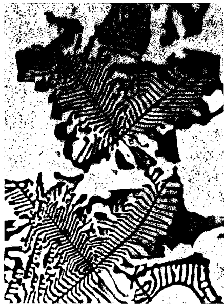
Figure 2(b). "Fish bone" eutectic Optical micrograph, Murakami etch, X 1000.
