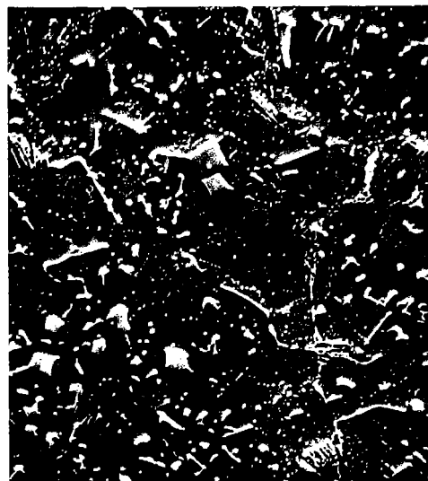
Figure 3(b). 2 W, 4 Nb, 5 Mo, 4 Cr, 1 V steel M_6C eutectic eutectic, finely-dispersed M_6C carbides and primary NbC. Scanning Electron Micrograph X 500.
