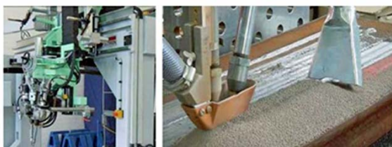
Figure 3. Submerged arc welding system.
