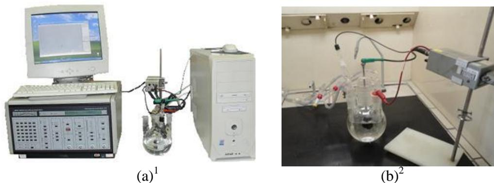
Figure 2. Electrochemical test; (a) Potentiostat PAR 273A, (b) Electrochemical cell.
