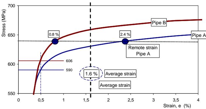
Figure 3. Comparison of average and remote strains.
