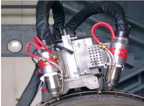
Figure 3. Tandem welding head.
