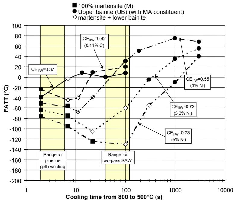
Figure 3. Correlation between FATT and the cooling time  $t_{8/5}$  for different steel compositions and microstructures occurring in the CGHAZ (acc. [2,3])
