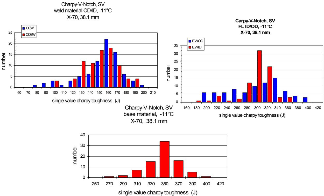
Figure 8. Charpy toughness Values (single values) for WM, HAZ (FL) and BM
