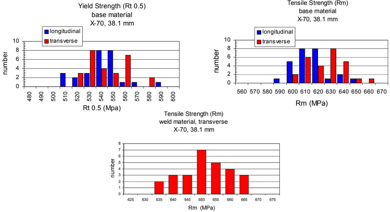
Figure 7. Strength distributions from orders with 38 mm wall thickness in X-70
