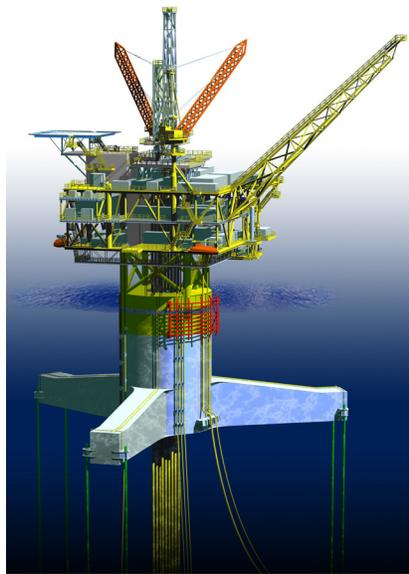
Figure 1. Principle of a TLP (the Atlantia Offshore Sea Star Design)
