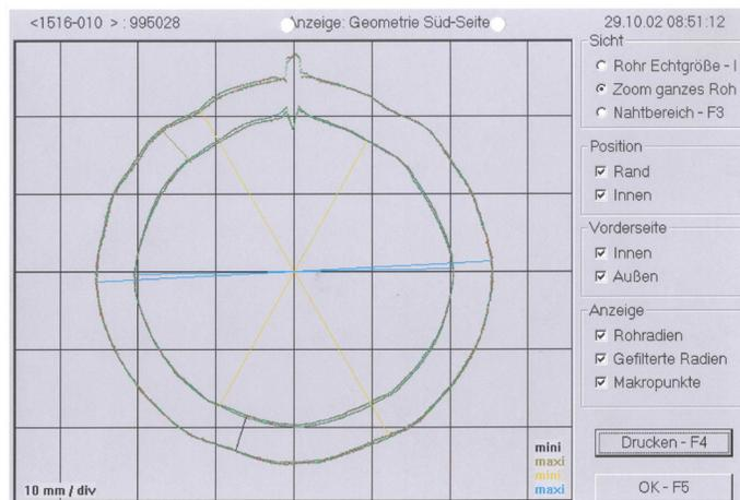
Figure 13. Characteristic shape of a pipe end
