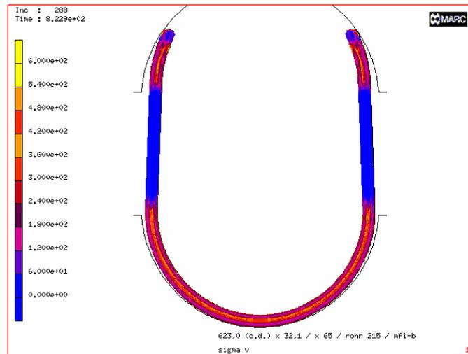
Figure 6. FEA Simulation of the O-ing Process
