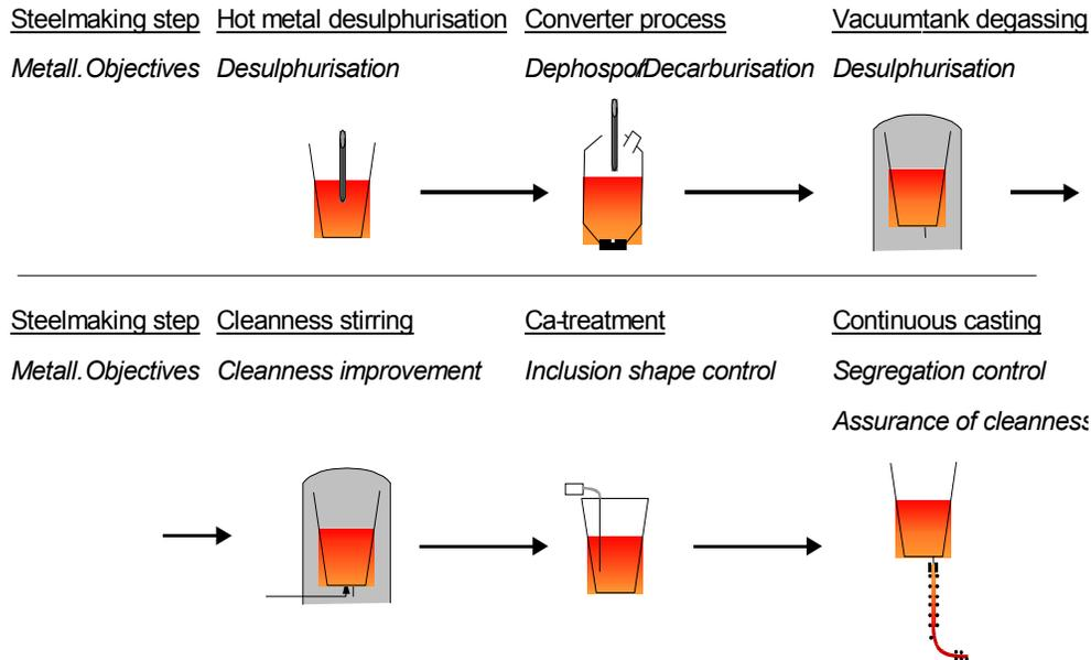
Figure 5. Steel making process, toughness optimized
