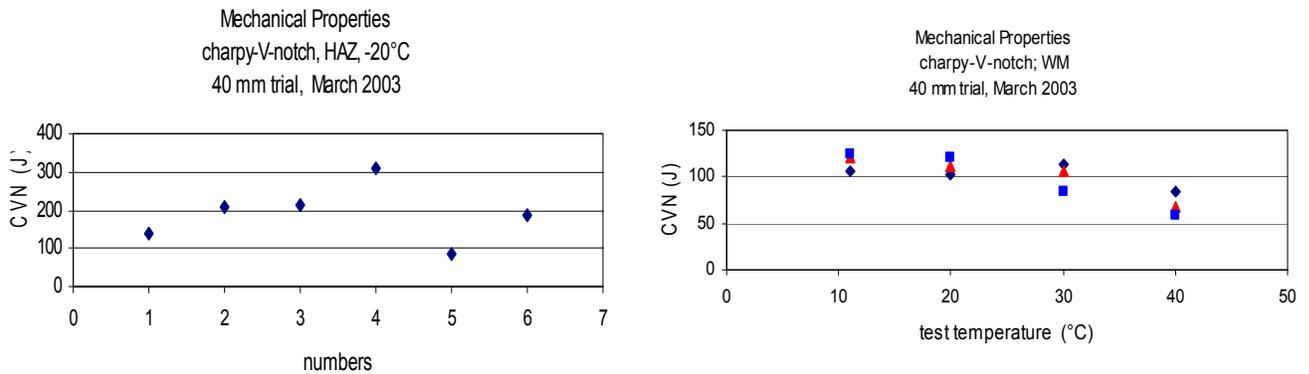
Figure 9. Charpy toughness Values (single values) for WM, HAZ (FL) for 40 mm wall
