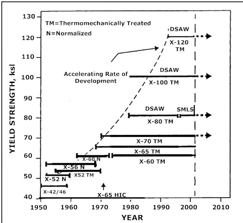
Figure 1. Development and application of pipe grades after J. M. Gray [5].
