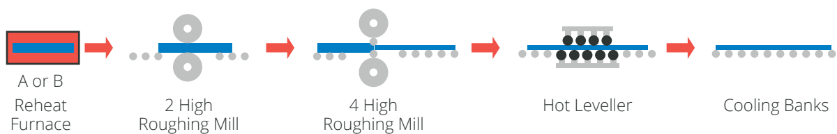
Figure 2a. Plate mill rolling. (Adapted from Corus-Namtec) [1].
