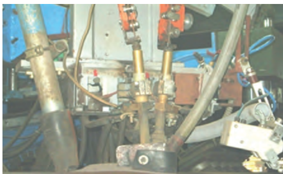
Figure 3b. Helical Submerged Arc Welding. (Image courtesy of Welspun Corp).
