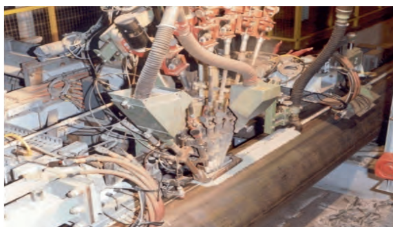
Figure 3a. Longitudinal Submerged Arc Welding (LSAW) of High Strength Low Alloy (HSLA) pipe. (Image courtesy of Tata Steel).
