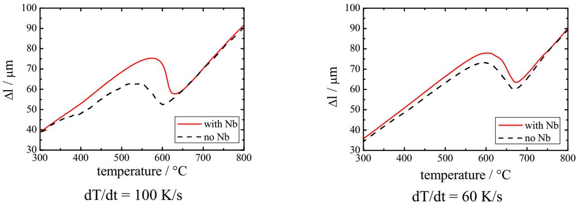
Figure 24. Measured length change as a function of the temperature for DP 600 alloys without and with Nb.
