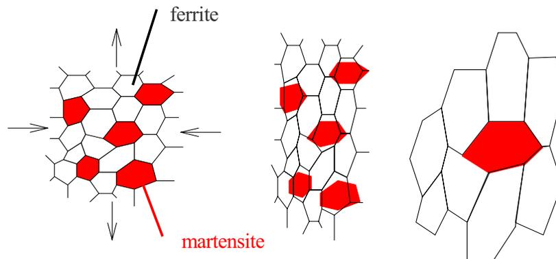
Figure 8. Schematic microstructure of a DP grade.
