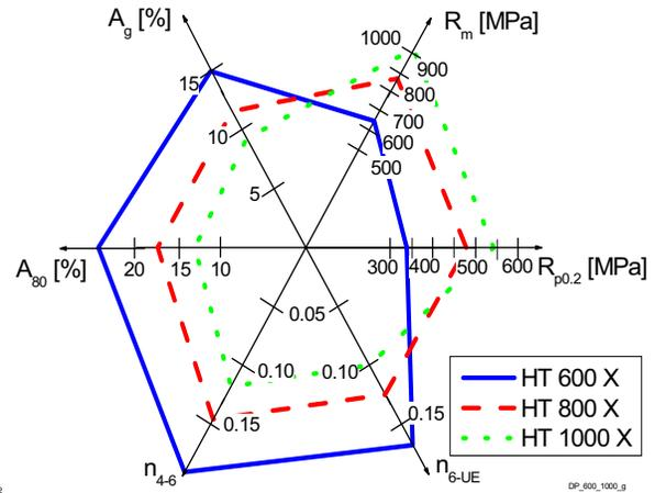
Figure 12. Typical mechanical properties of the DP grades HT600X, HT800X and HT1000X.
