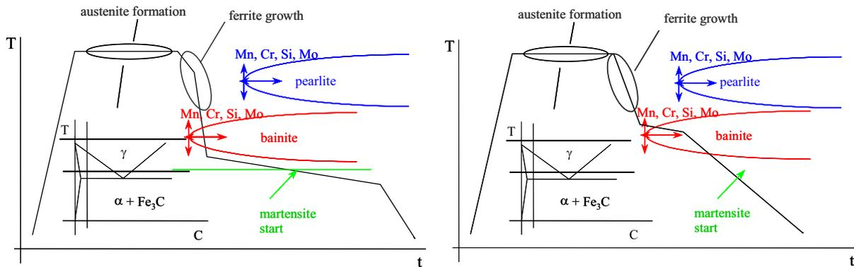
Figure 15. Schematic representation of the phase transformations of PM steel grades during heat-treatment.
