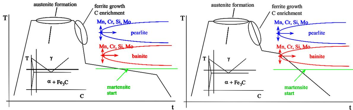
Figure 9. Schematic representation of the phase transformations of DP steel grades during heat treatment.
