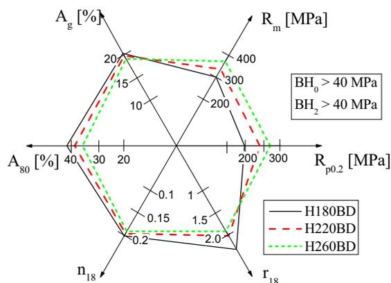
Figure 6. Mechanical properties in the transversal direction of partially stabilized Nb ULC grades produced via HDG (the BH values are measured in transversal direction, too).
