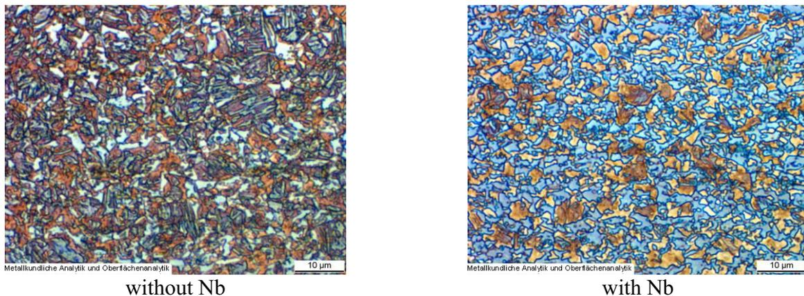
Figure 27. Microstructure of DP 800 alloys without and with Nb after annealing at 850 °C / 60 s and cooling with 40 K/s.
