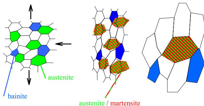
Figure 19. Schematic microstructure of a TRIP grade.
