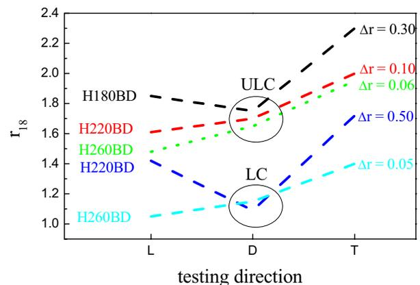
Figure 7.  $r$ -value in the longitudinal (L), diagonal (D) and transversal (T) direction of partially with Nb stabilized ULC BH grades and LC BH grades produced via HDG.
