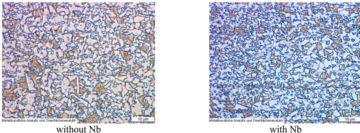
Figure 25. Microstructure of DP 600 alloys without and with Nb after annealing at 850 °C / 60 s and cooling with 80 K/s.
