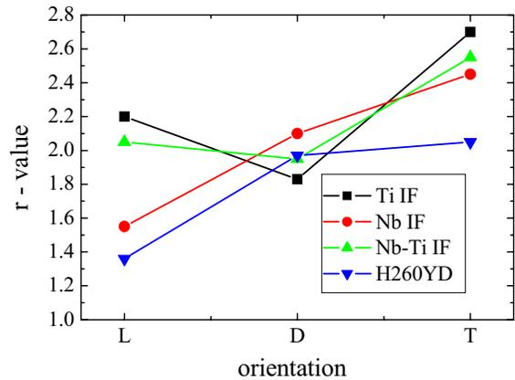
Figure 2.  $r$ -value in the longitudinal (L), diagonal (D) and transversal (T) direction for a soft Ti-IF, a soft Nb-IF, a soft Nb + Ti-IF and a high strength Nb + Ti-IF-grade with a minimum yield strength of 260 MPa (H260YD).
