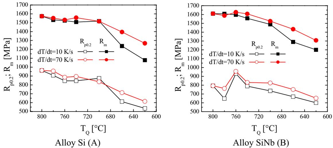
Figure 31. Yield and tensile strength of alloys A and B as a function of the quenching temperature ( $T_{IC} = 800^\circ\text{C}$ , cooling rate from intercritical annealing to the quenching temperature  $dT/dt = 10^\circ\text{K/s}$ ).
