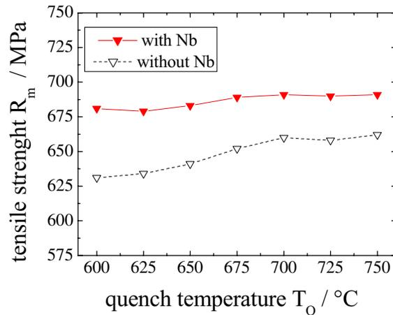
Figure 28. Mechanical properties as a function of the quenching temperature  $T_Q$  for DP 600 with and without Nb after simulating an annealing cycle according to the continuous annealing line of *voestalpine*
