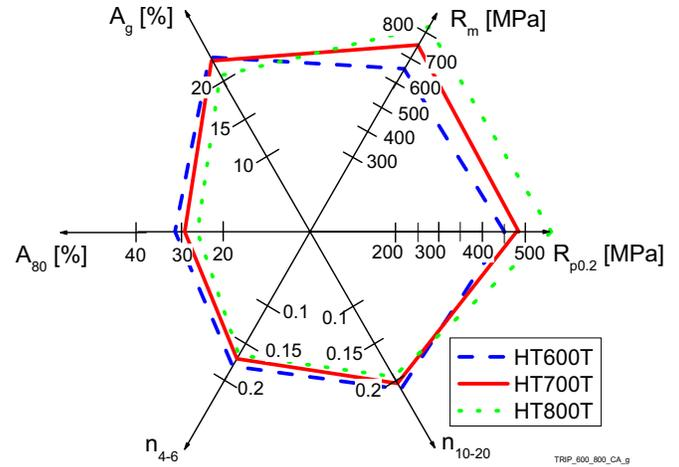
Figure 23. Mechanical properties of TRIP grades with minimum tensile strength of 600 MPa (HT600T), 700 MPa (HT700T) and 800 MPa (HT800T).
