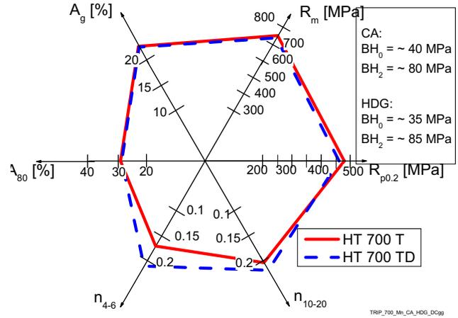
Figure 21. Mechanical properties of a continuously annealed (HT700T) and a hot-dip galvanized (HT700TD) TRIP grade.
