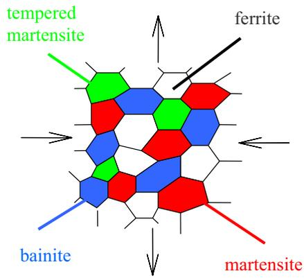
Figure 13. Schematic microstructure of a PM grade.
