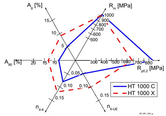
Figure 18. Comparison of the mechanical properties of the DP grade HT1000X and the PM grade HT1000C.
