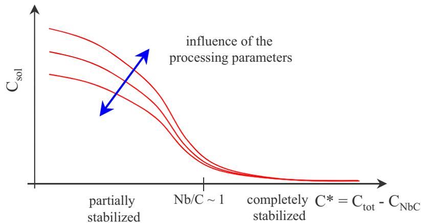
Figure 5. Impact of the carbon and Nb content on the carbon content in solid solution.
