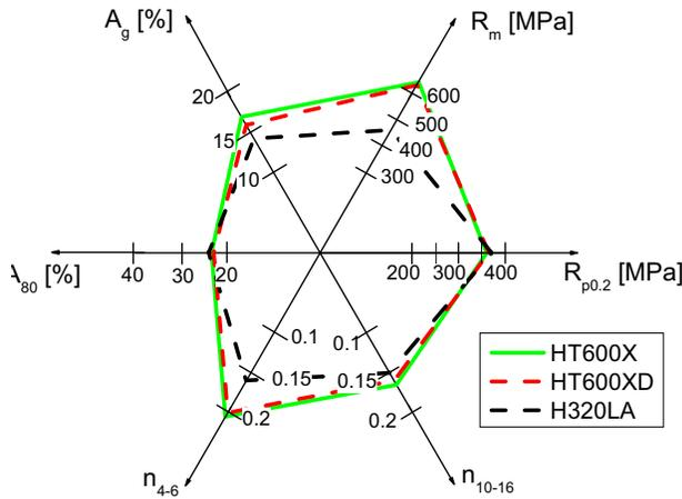
Figure 11. Comparison between the mechanical properties of the DP grades HT600X, HT600XD and the micro-alloyed grade H320LA.
