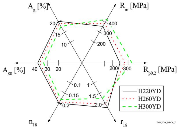
Figure 4. Mechanical properties in the transversal direction for HDG high-strength IF grades with minimum yield strengths of 220 (THM 220 IF), 260 (THM 260 IF) and 300 MPa (THM 300 IF).
