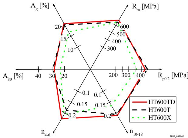
Figure 22. Comparison between the mechanical properties of the DP grade HT600X and the TRIP grades HT600T and HT600TD.
