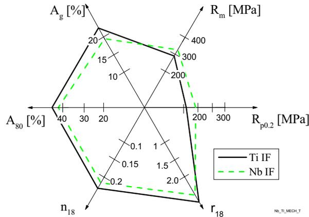
Figure 1. Comparison of the mechanical properties in transversal direction of a standard Ti-IF grade and a Nb-IF grade.
