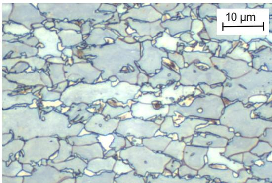
Figure 10. Typical microstructure of a DP grade.
