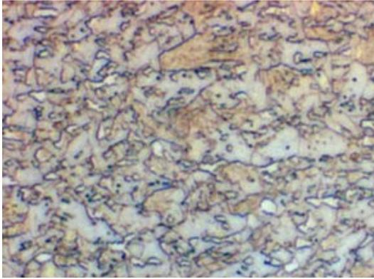
Figure 16. Typical microstructure of a PM thin sheet steel grade (HT800C).
