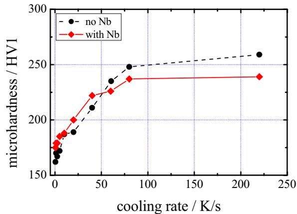
Figure 26. Microhardness as a function of the cooling rate for DP 600 alloys with and without Nb after annealing at 850 °C / 60 s.
