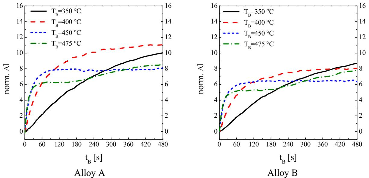
Figure 32. Influence of the isothermal holding temperature on the transformation behavior of the austenite in the bainitic range for alloys A and B ( $T_{IC} = 800^{\circ}\text{C}$ ,  $t_{IC} = 60\text{s}$ ,  $dT/dt = 70^{\circ}\text{K/s}$ ).
