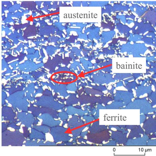
Figure 20. Microstructure of a TRIP thin sheet steel grade (HT700TD).
