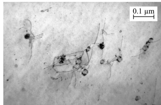
Small C and Nb rich (Ti,Nb)(C,N) particles
