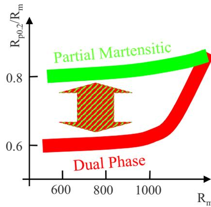
Figure 14. Yield ratio as a function of the tensile strength for DP and PM grades.
