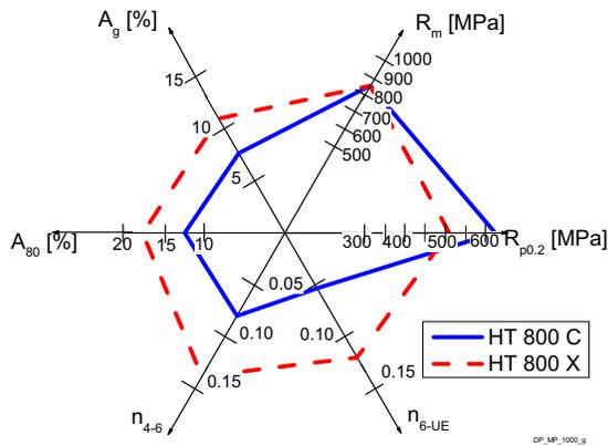
Figure 17. Comparison of the mechanical properties of the DP grade HT800X and the PM grade HT800C.
