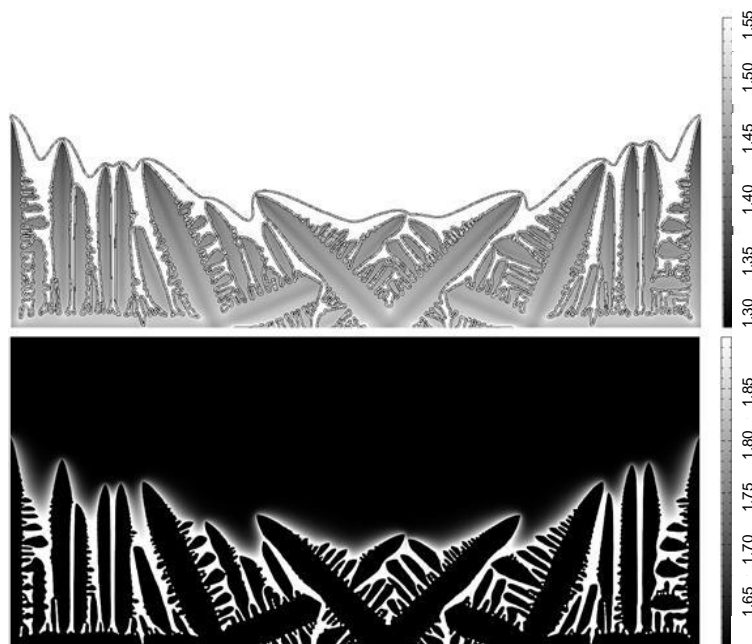
Figure 5. Manganese distribution (wt.%) within dendrites (top) and the liquid phase (bottom) obtained by Phase Field simulation of the solidification of a low-alloy steel.
