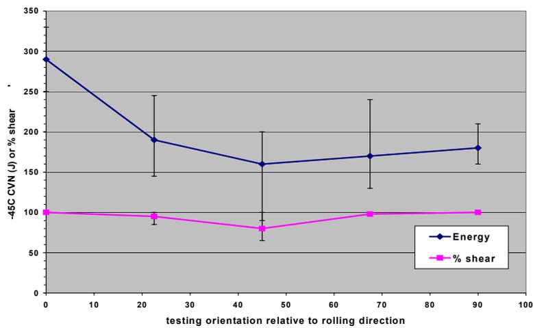
Figure 13. CVN energy as a function of testing direction 14.2mm-X70 MoNb<sup>6</sup>
