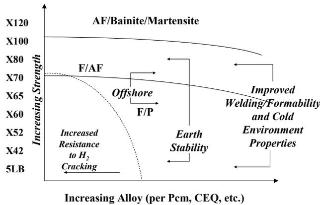
Fig. 3 Illustration of pipeline design attributes, increasing alloy (per Pcm, CEQ, etc) and API strength
