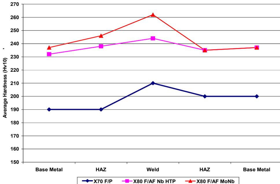
Figure 29. Average cross-weld hardness of recent API pipeline steels.
