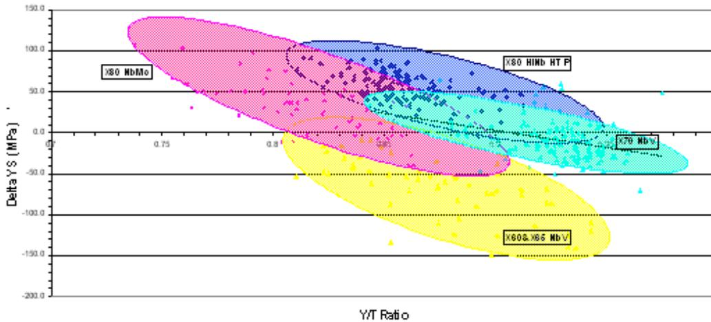
Figure 20. Dependence of plate-to-pipe strength change on skelp Y/T ratio
