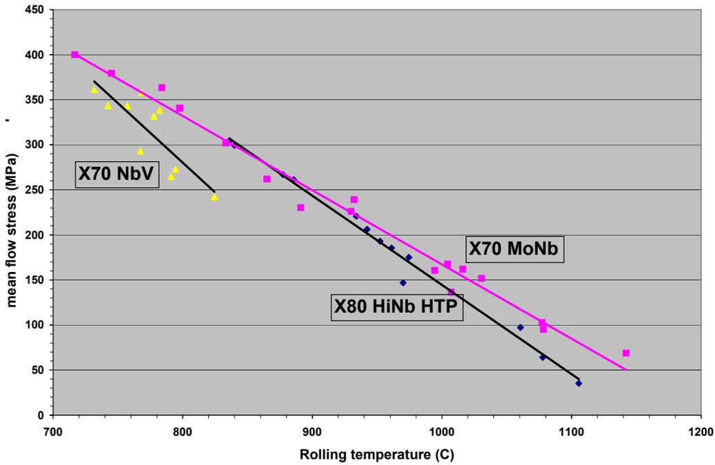
Fig. 23 Comparison of mean hot rolling flow stress - X70 and X80 steels
