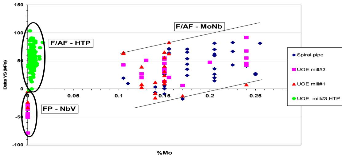
Figure 10. Dependence of plate-to-pipe YS change on Mo content – X65 – X80
