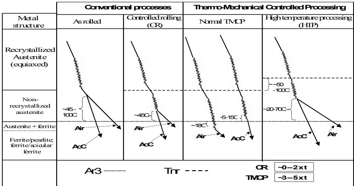
Figure 6. Schematics of rolling process thermo-mechanical paths for the production of API linepipe coil and plate
