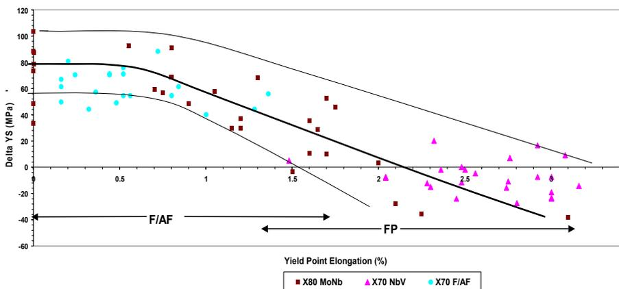
Fig. 16 Dependence of plate-to-pipe strength change on Luder's elongation X70 and X80,  $t/D \sim 0.9-1.2\%$
