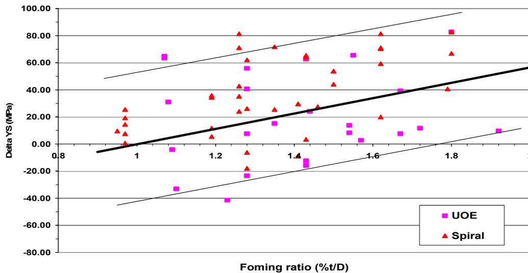
Figure 17. Strength change on pipe forming ratio
