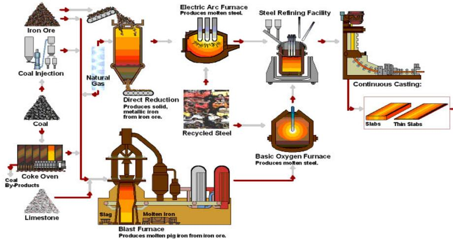
Figure 4. Schematic of the steelmaking process for API transmission linepipe grades
