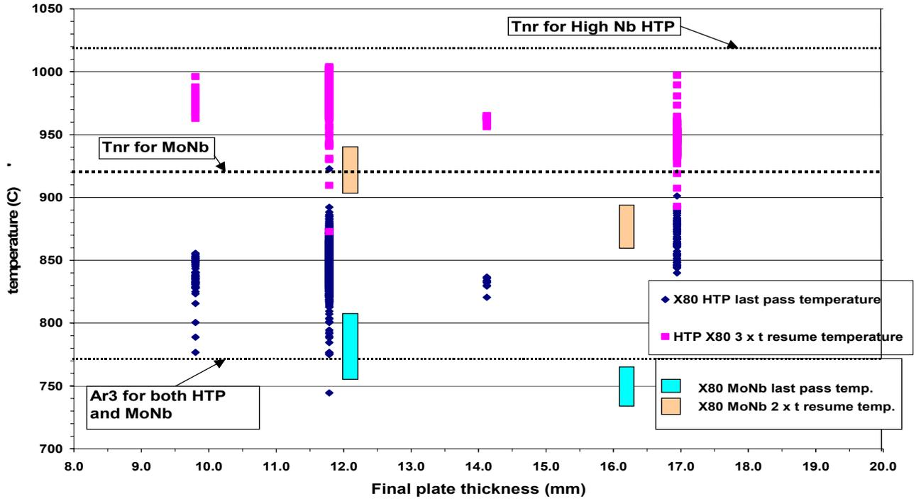
Fig. 22 Comparison of HTP vs. normal TMCP rolling temperature set points for X
