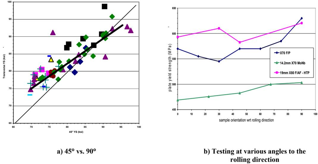
Figure 12. Illustration of skelp strength anisotropy – X80
