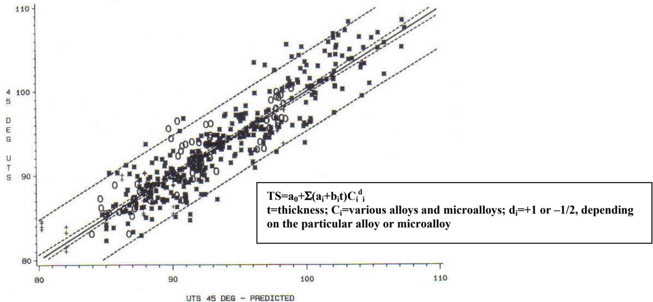
Figure 19. Tensile strength prediction model
