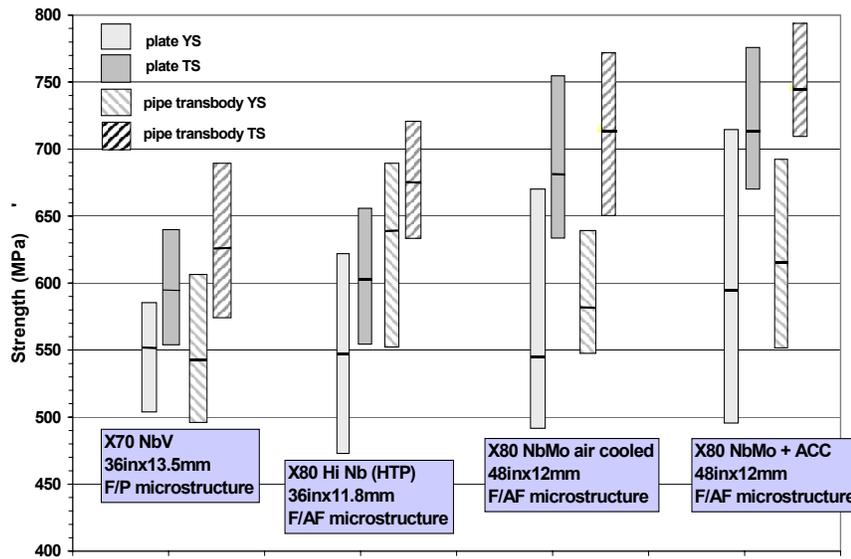
Fig. 24 Plate and pipe strength – recent North American X70 and X80 projects
