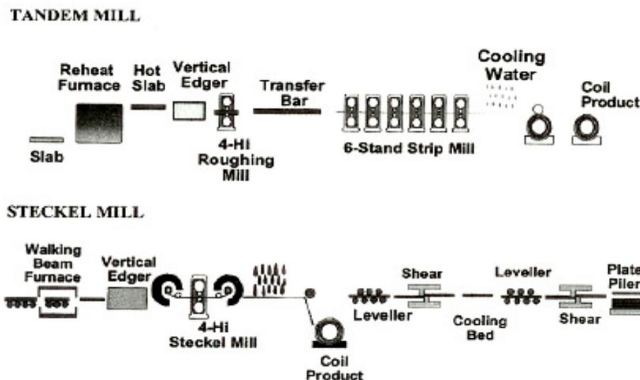
Fig. 5 Typical tandem (strip) and Steckel mill layouts
