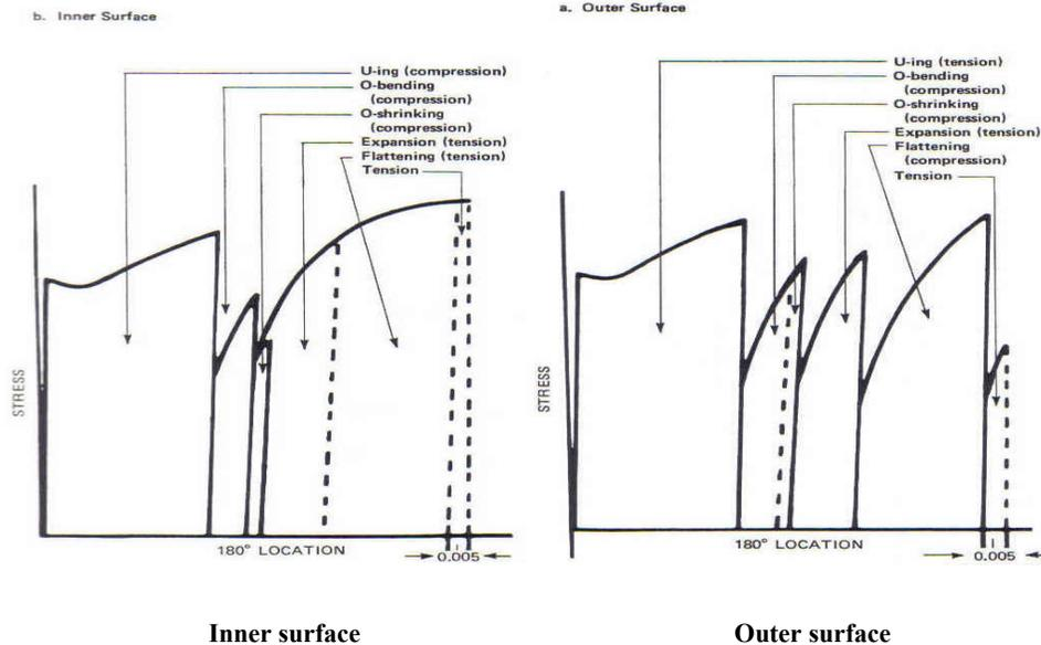
Figure 14. Inner and outer surface strain path in UOE pipe forming and testing
