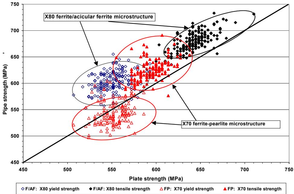
b) Recent X70 and X80 – illustrating the generally neutral or positive shift in tensile strength compared to yield strength
