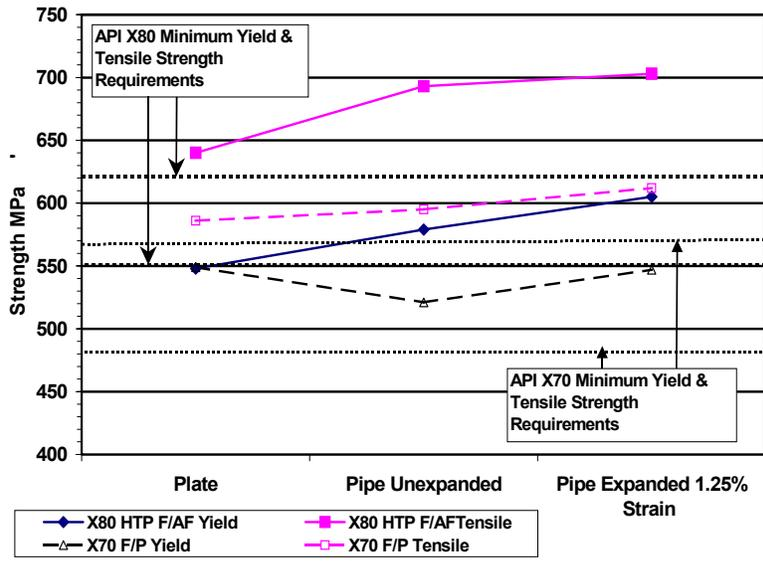
Figure 18. Strength change during pipeforming and cold expansion.
