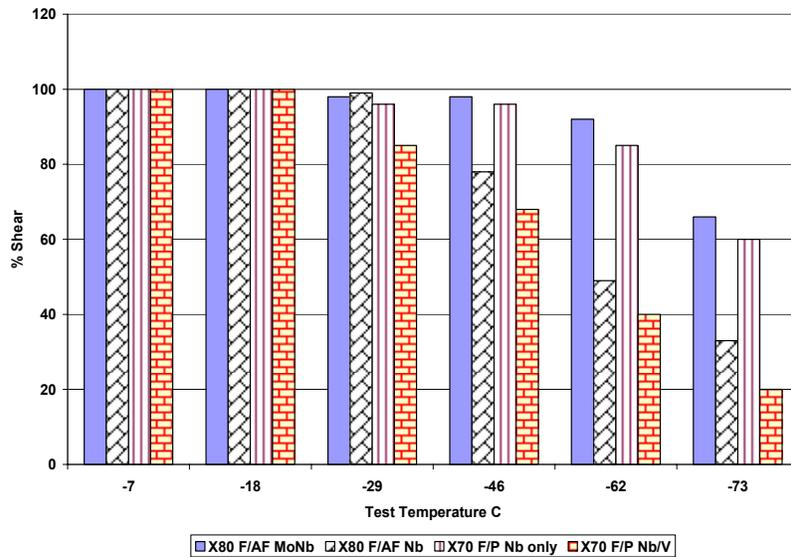
Figure 28. DWTT transition data for F/AF and F?P microstructures and alloying approaches
