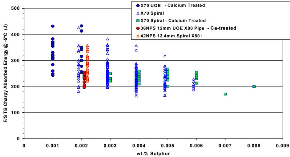
Figure 26. X80 Trans-body pipe notch toughness
