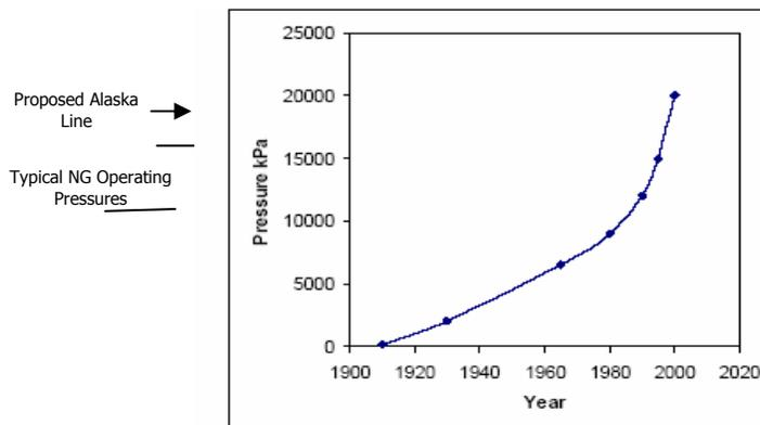
Figure 2. Increase in North American natural gas operating pressures
