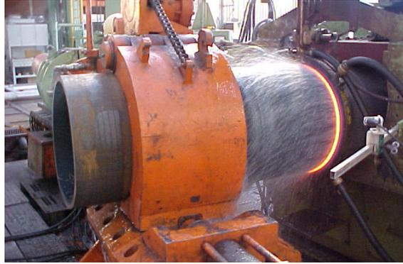
Figure 1 - The 20in. X80 bending process. Notice that, just after the heating coil, the pipe is water cooled.
