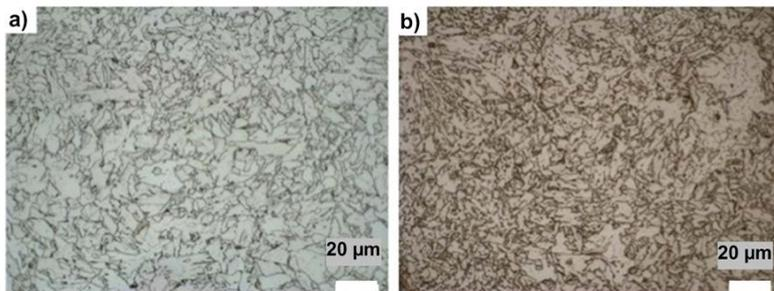
Figure 10. Optical micrographs of (a) Steel A and (b) Steel B after multi-pass weld HAZ thermal cycle predominantly showing polygonal ferrite grains.
