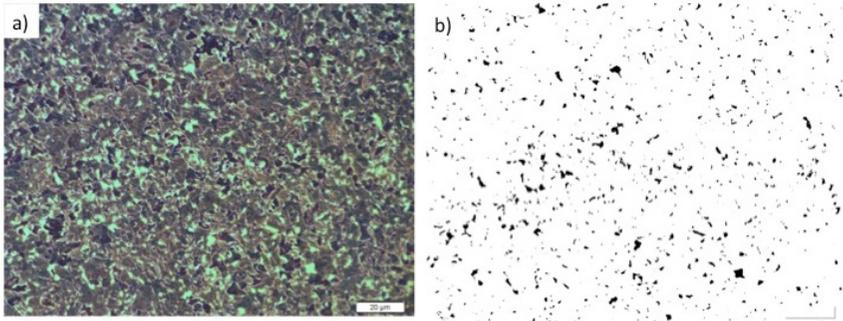
Figure 8. (a) Microstructure of Steel A after ICRHAZ thermal cycle when etched with Le Pera's etchant showing bright regions (MA constituents) and darker (ferritic) regions and (b) Image analysis of Figure 8(a); Bright MA constituents are isolated and shown as dark regions.
