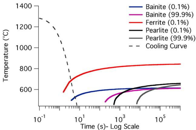
Figure 3. CCT diagram for Steel A generated from JMatPro®, predicting the formation of a mixed bainitic + martensitic microstructure along with some ferrite when subjected to a thermal cycle shown in Figure 2.
