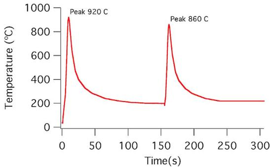
Figure 5. Thermal cycle for the generation of ICRHAZ microstructures in Steel A and Steel A1.
