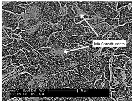
Figure 9. SEM image of ICRHAZ microstructure of Steel A showing MA constituents present at ferrite grain boundaries.
