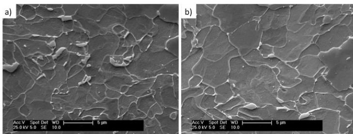
Figure 11. SEM images of microstructures of (a) Steel A and (b) Steel B after multi-pass weld HAZ thermal cycles showing polygonal ferrite grain size 6-10  $\mu\text{m}$ .
