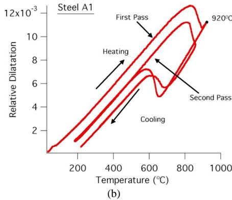
Figure 7. Dilatometry with reference to temperature of (a) Steel A and (b) Steel A1 for the two-pass weld HAZ treatment showing complete austenitization after 1<sup>st</sup> pass ( $> Ac_3$ ) and incomplete austenitization ( $Ac_1 < 860$  °C  $< Ac_3$ ) in second pass.
