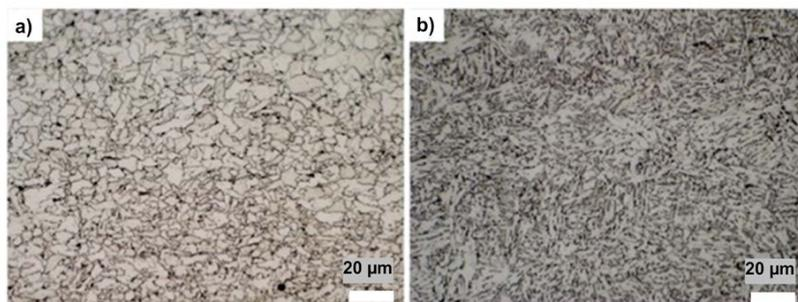
Figure 1. (a) As-rolled microstructure of Steel A showing polygonal ferrite microstructure, (b) As-rolled microstructure of Steel B showing Acicular/Widmanstätten type grains.
