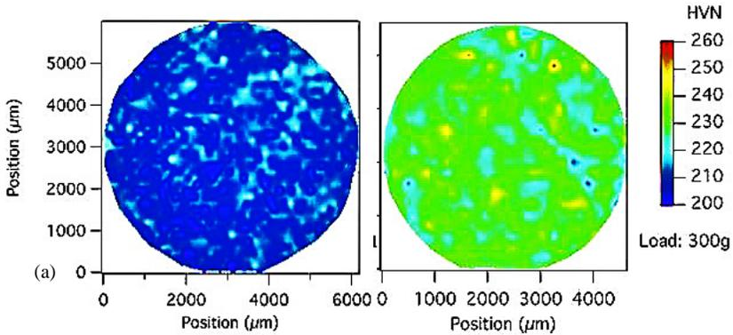
Figure 12. Hardness maps generated from the cross sections of simulated multipass weld HAZ Gleeble samples of (a) Steel A and (b) Steel B.
