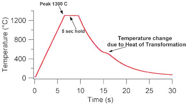
Figure 2. Temperature vs. time graph showing thermal cycle used for obtaining a bainitic/martensitic microstructure in Steel A.
