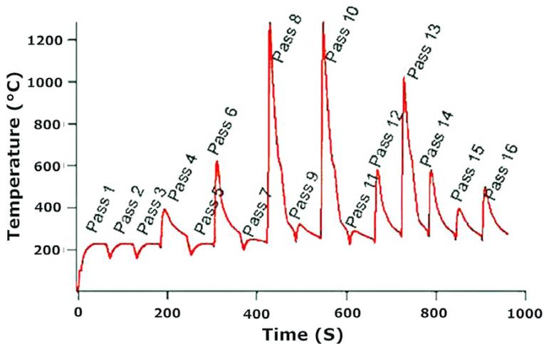
Figure 6. Generated thermal cycle for multi pass HAZ using an FEA model for peak temperature and Rosenthal-type cooling curves.
