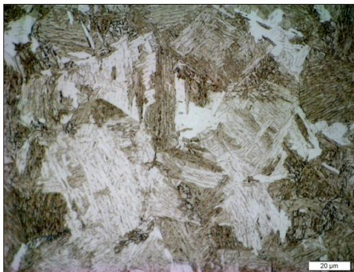
Figure 4. Microstructure of Steel A after the heat treatment (Figure 2); Steel A with this microstructure is now referred to as Steel A1.
