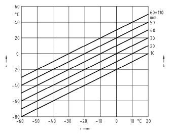
Figure B.4-3 — Design reference temperature and impact test temperature post weld heat treated (PWHT) condition, for 310 N/mm<sup>2</sup> <  $R_e \le 460$  N/mm<sup>2</sup> : 27 J
