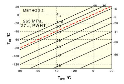
Figure 12a. New nomogram for conventional steel grades with strength level 265 MPa, dashed line allows use of thickness up to 110 mm if  $T_{KV}$  = 40 J at  $T_{R}$ .
