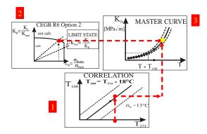
Figure 7. Principal derivation of limit state of fracture with fracture mechanics methods.
