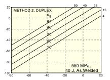
Figure 10b. Nomogram for austenitic ferritic  $\text{Re} \leq 550 \text{ MPa}.$
