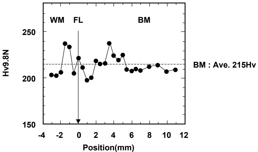
Figure 12. Typical hardness distribution of the weld joints.
