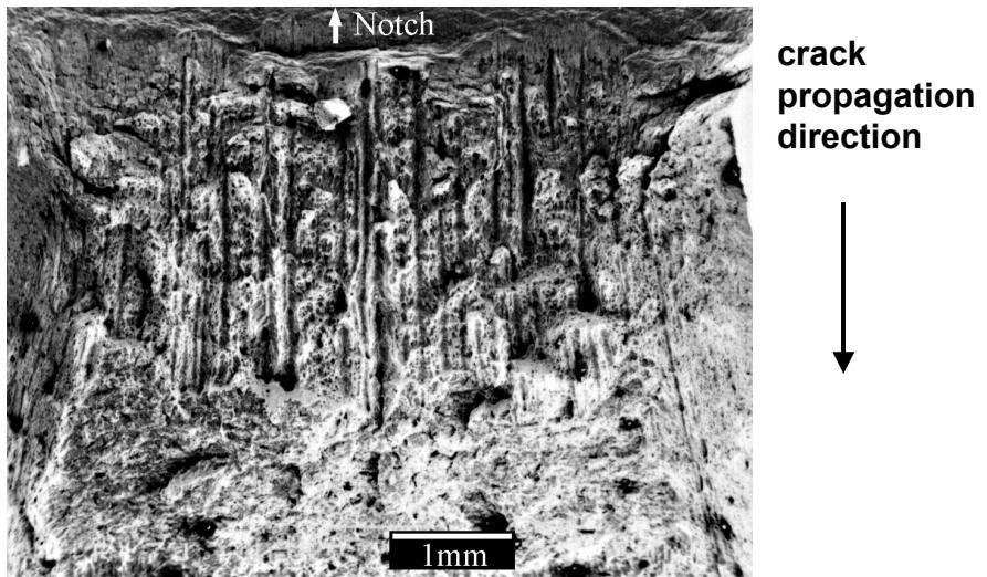
Figure 6. Observation of fractured surface of the specimen containing sulfur content of 72 ppm.
