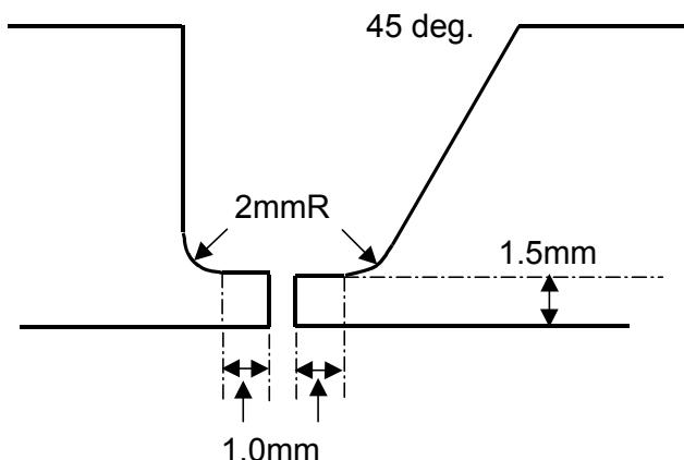
Figure 10. Schematic illustration of edge preparation for welding.
