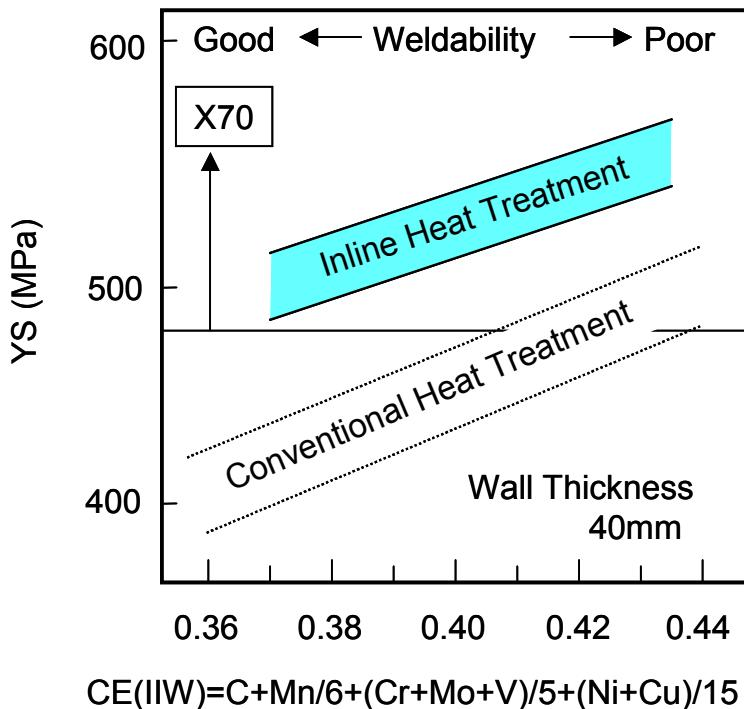
Figure 4. The difference of strength between inline and offline heat treatment
