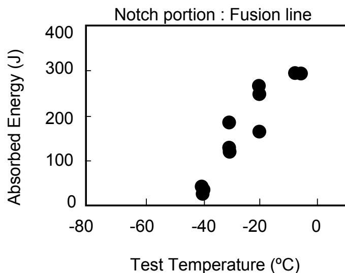
Figure 13. Charpy absorbed energy transition curve of the weld joints.
