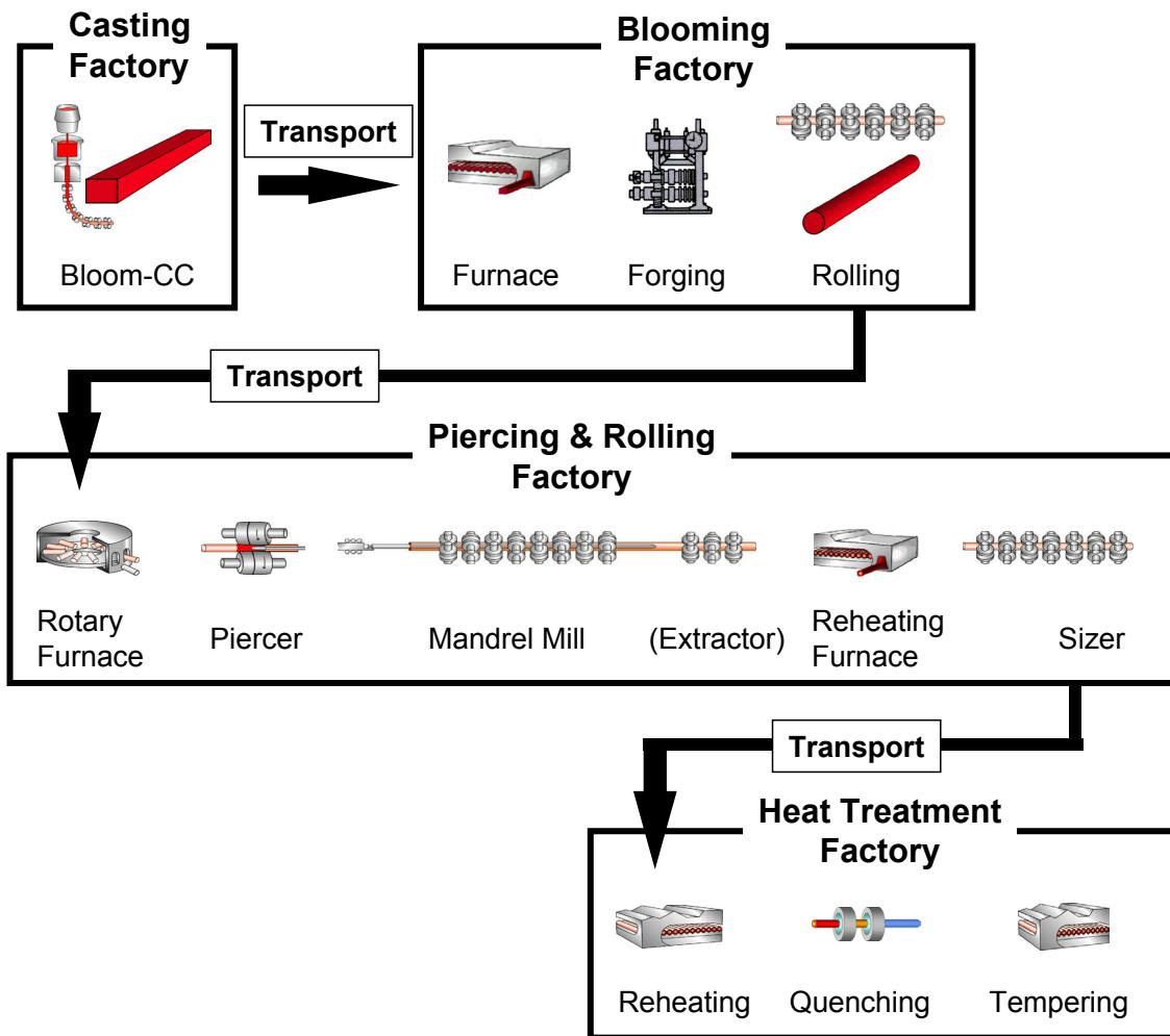
Figure 2. Schematic illustration of conventional production line for seamless pipe.
