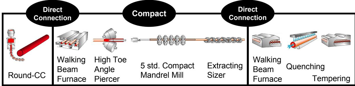
Figure 1. Schematic illustration of the newly constructed medium-size mill and inline heat treatment facilities.
