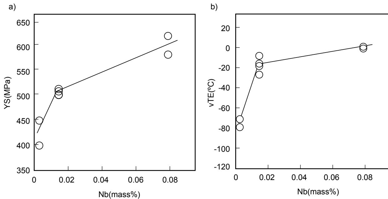
Figure 8. Effect of the niobium addition on yield strength and toughness for inline heat treatment;
