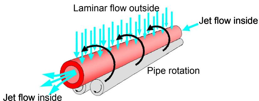
Figure 3. Schematic illustration of the inline quenching device.
