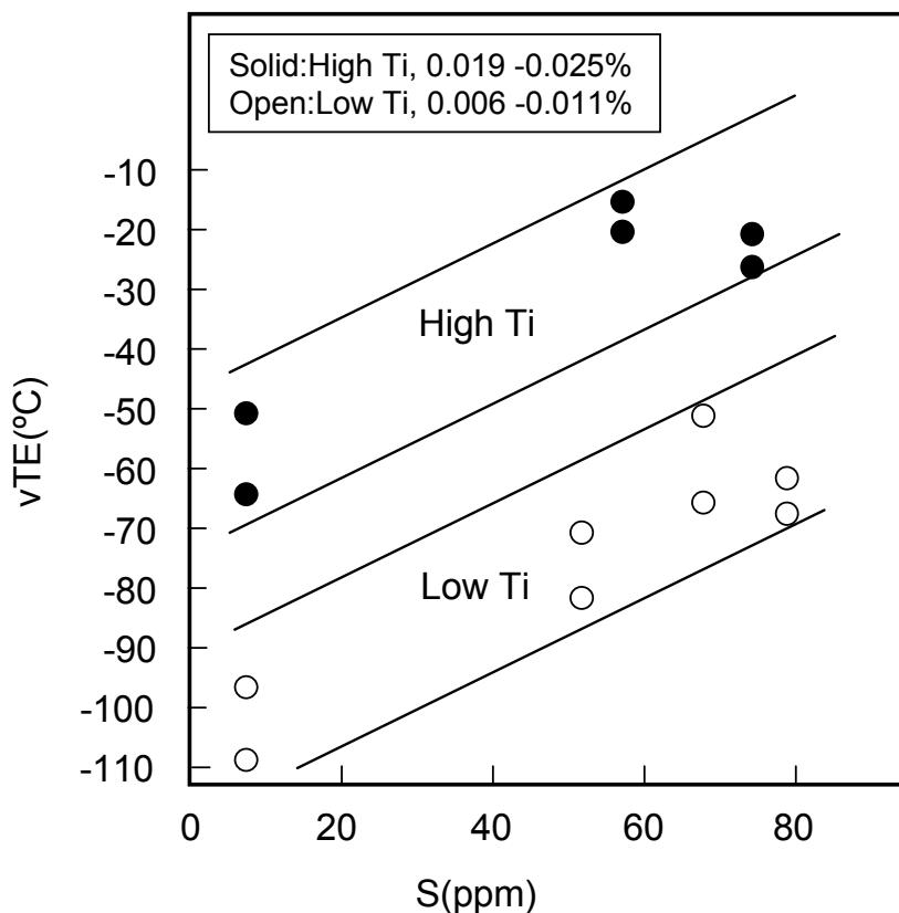
Figure 5. Influence of sulfur and titanium content in steel on toughness.
