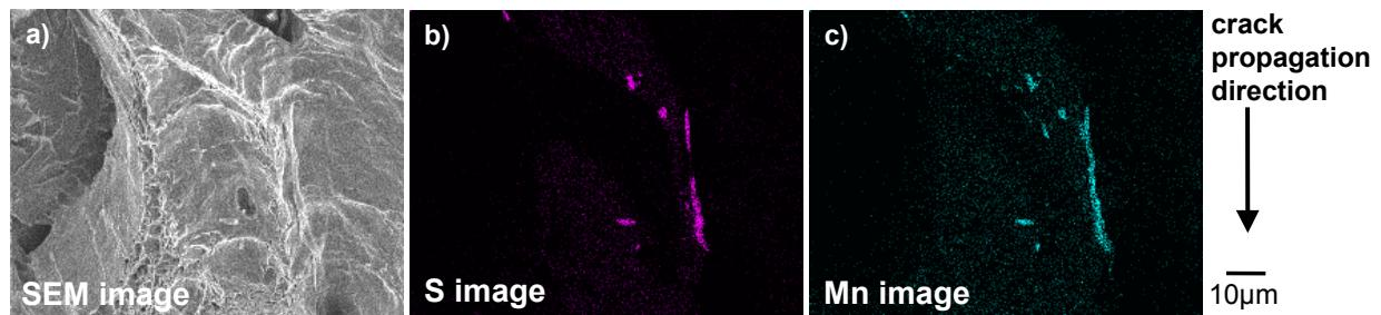
Figure 7. Observation of fractured surface of the specimen containing sulfur content of 72 ppm using EDS. a):SEM image b):sulfur image C):manganese image
