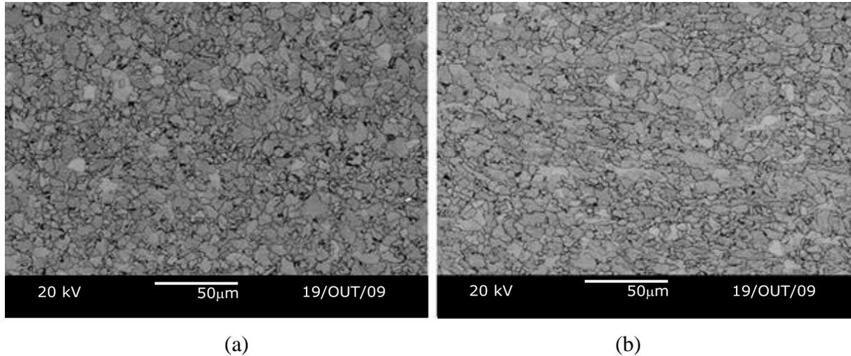
Figure 4. HAZ microstructures; (a) subcritical zone and (b) intercritical zone.
