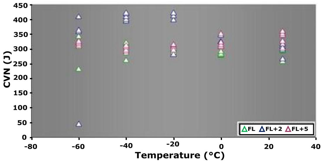
Figure15. Charpy test results from girth weld using low heat input – X70MS.
