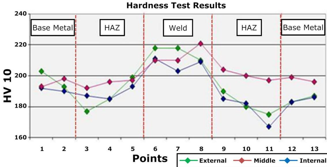
Figure 5. Hardness test results - longitudinal joint.
