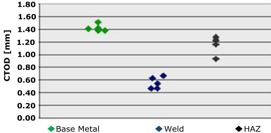
Figure 8. CTOD test results at 0 °C.
