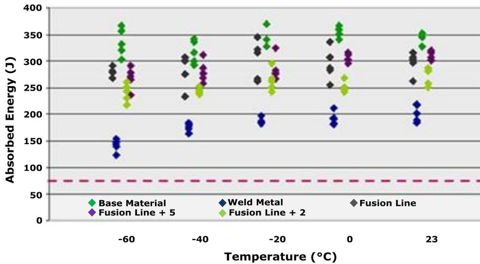
Figure 6. Charpy V-notch test results.
