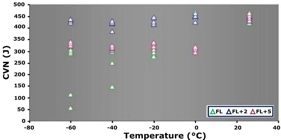
Figure 14. Charpy test results from girth weld using high heat input – X70MS.
