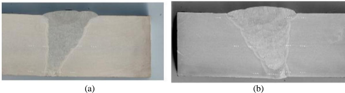
Figure 11. Macro sections; (a) Low heat input (Magnification: x0.7) and (b) High heat input (Magnification: x0.7).
