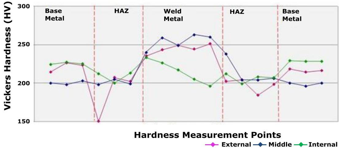
Figure 12. Hardness results using low heat input.
