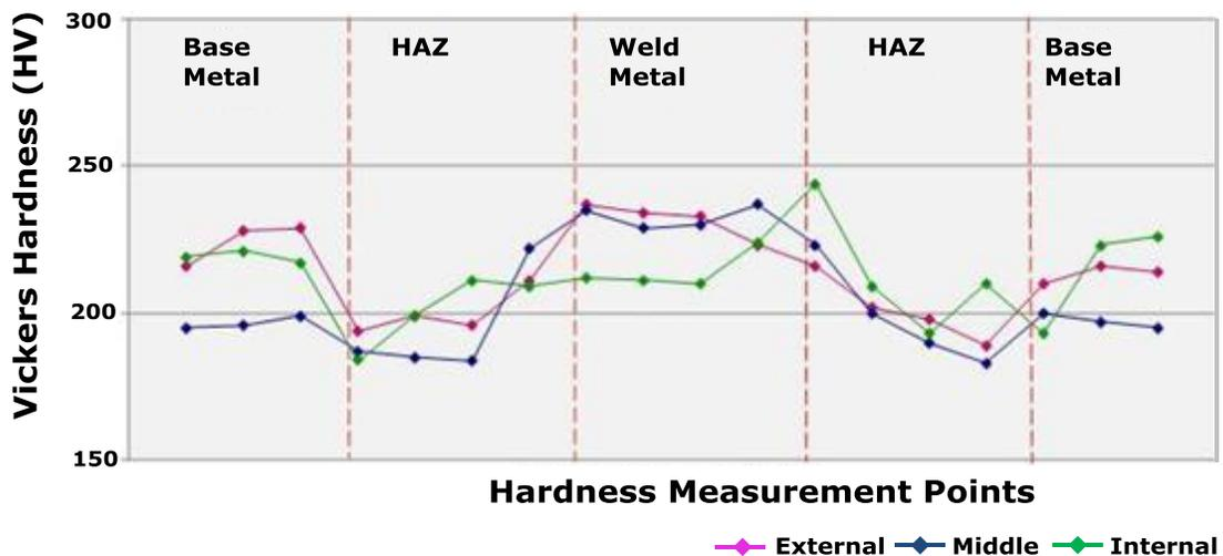
Figure 13. Hardness results using high heat input.
