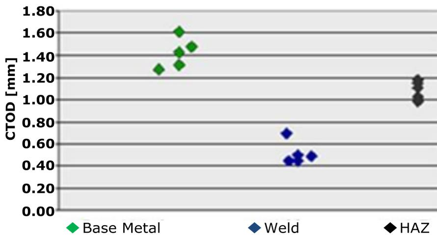
Figure 9. CTOD test results at -20 °C.
