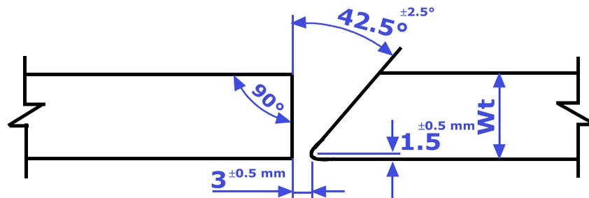
Figure 10. Diagram of bevel design.
