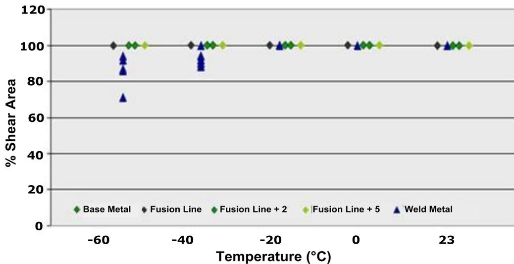
Figure 7. Shear area results from Charpy V-notch tests.
