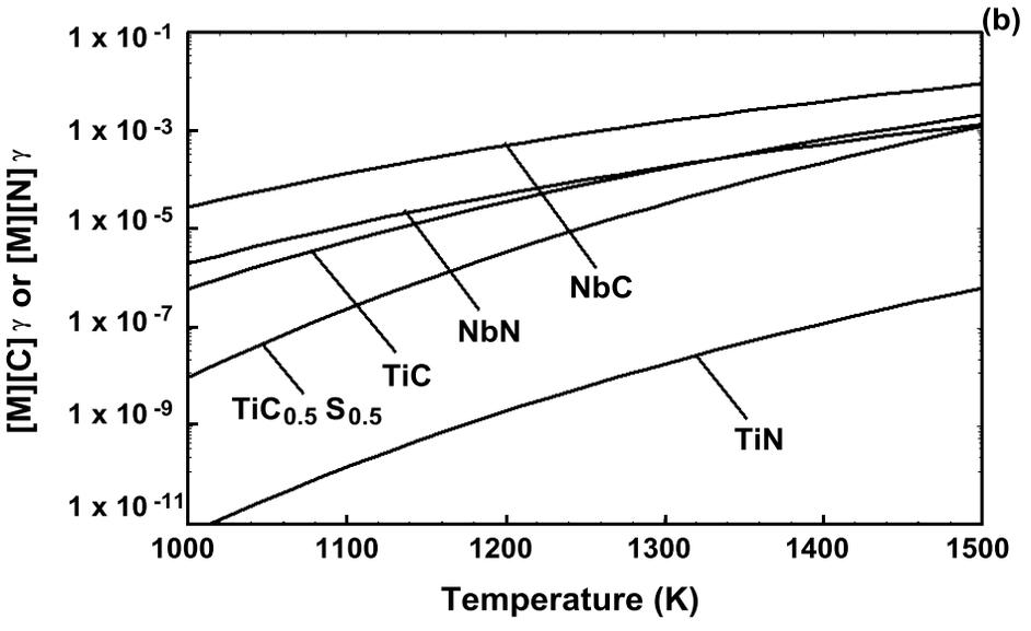
Figure 1. Oxides, carbides and nitrides formed at different temperatures; (a) Chemical driving force of compounds at high temperature, (b) Solubility of carbides and nitrides of Nb, Ti in austenite (S: 0.003wt.%) [4].
