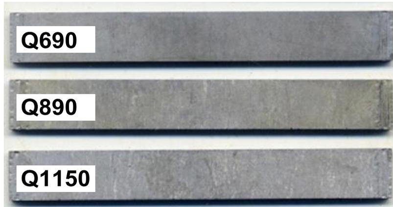
Figure 10. Specimens after four-point bending test 360 h.
