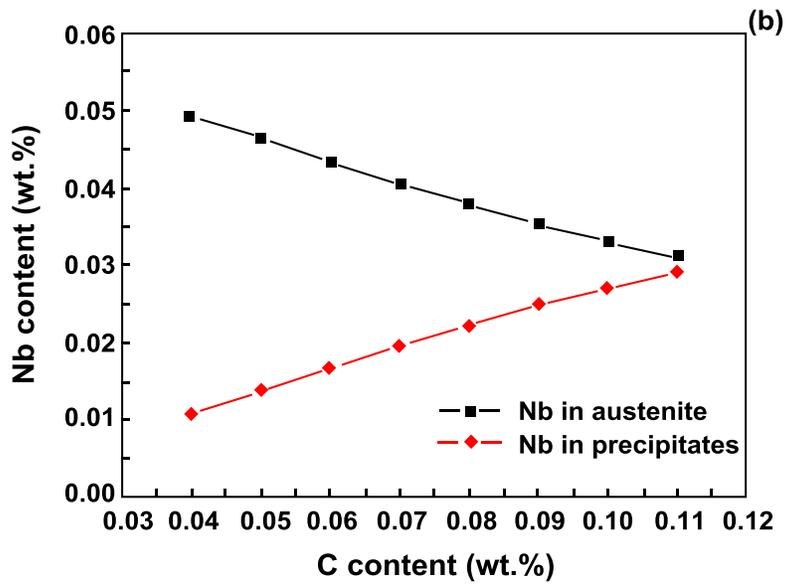
Figure 2. Nb contents in austenite and precipitates at different Nb total contents and C contents (austenized at 1200 °C); (a) Nb in austenite and precipitates at different Nb total content (0.11%C-0.03%V-0.02%Ti-0.0040%N-x%Nb), (b) Nb in austenite and precipitates at different carbon contents (0.06%Nb-0.03%V-0.02%Ti-0.0040%N-x%C) [5].
