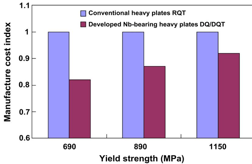
Figure 12. Comparison of manufacturing costs of conventional heavy plates (RQT) and developed Nb-bearing heavy plates (DQ/DQT).
