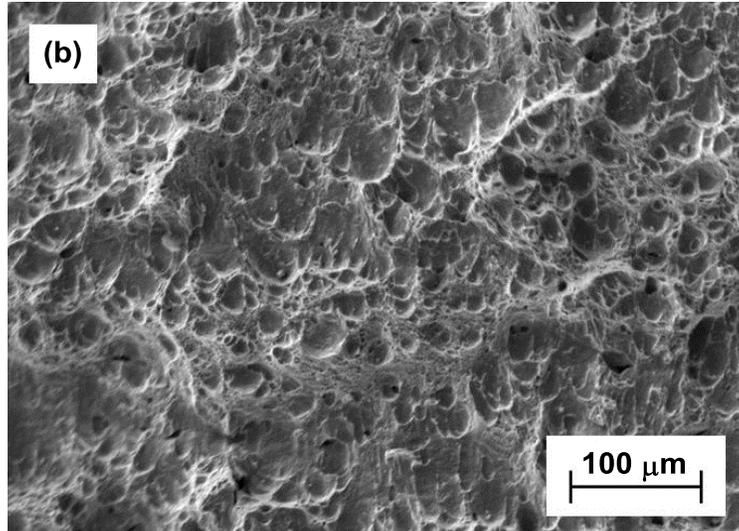
Figure 8. Instrumented impact results of steel plate (690 MPa) produced by DQ with cooling rate of 20 °C/s and tempered at 630 °C; (a) displacement - load curves, (b) fracture morphology [9].
