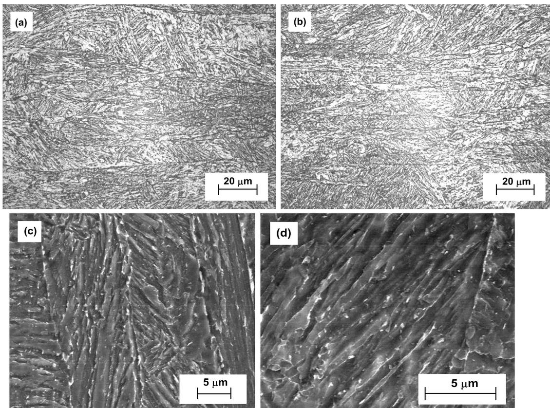
Figure 3. Microstructure of steel plates with minimum yield strength of 690 MPa produced by DQ with;
