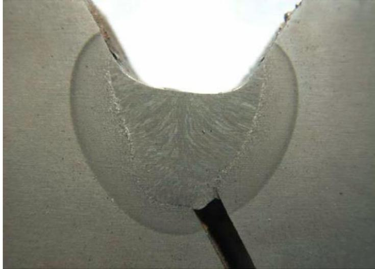
Figure 11. Section of Oblique Y type groove welding crack sample (preheating 150 °C).
