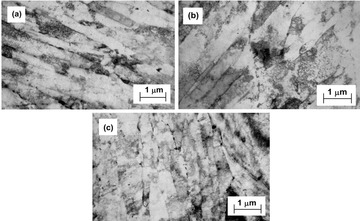
Figure 4. TEM micrographs of steel plates with yield strength 690 MPa produced by direct quenching (cooling rate 20 °C/s) followed by tempering at different temperatures; (a) 610 °C, (b) 630 °C, (c) 650 °C [9].
