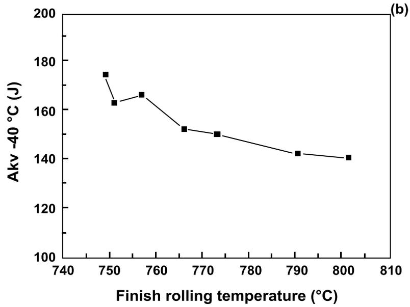
Figure 7. Effect of finish rolling temperature on; (a) tensile strength, (b) -40 °C Charpy V-notch impact energy of Q890CF.
