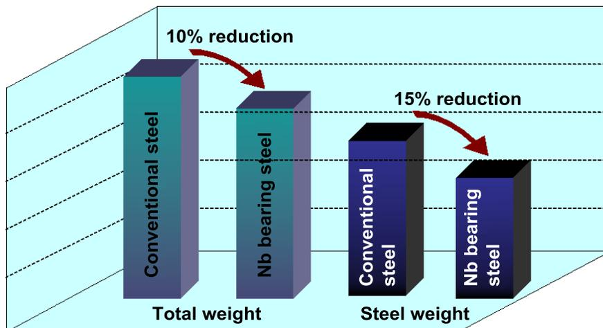
Figure 13. Total and steel weight reduction of mine hydraulic support ZFY18000/28/53D through replacing conventional steel by developed Nb-bearing steel heavy plates.
