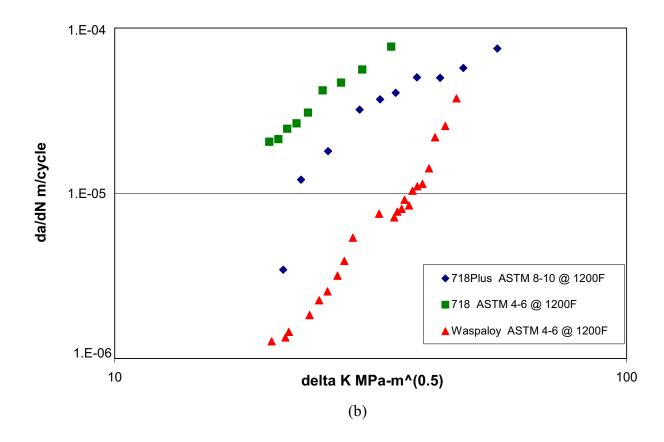
Figure 5. Fatigue Crack Growth Rate of Allvac<sup>®</sup> 718Plus<sup>™</sup> Alloy, 718 and Waspaloy at no hold time (a) and 100 second hold time (b).
