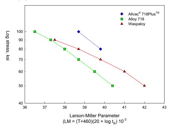
Figure 1. Larson-Miller Stress Rupture Life Comparison
