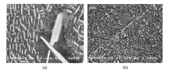
Figure 4. Microstructure of (a) Alloy 718 and (b) Allvac<sup>®</sup> 718Plus<sup>™</sup> after 350 Hours of Thermal Exposure at 1400°F. (Original magnification 20,000x).
