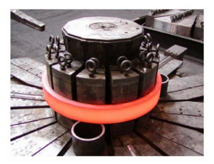
Figure 6. Seamless Rolled Ring of Allvac<sup>®</sup> 718Plus<sup>™</sup> Alloy (Courtesy of Firth Rixson Viking)
