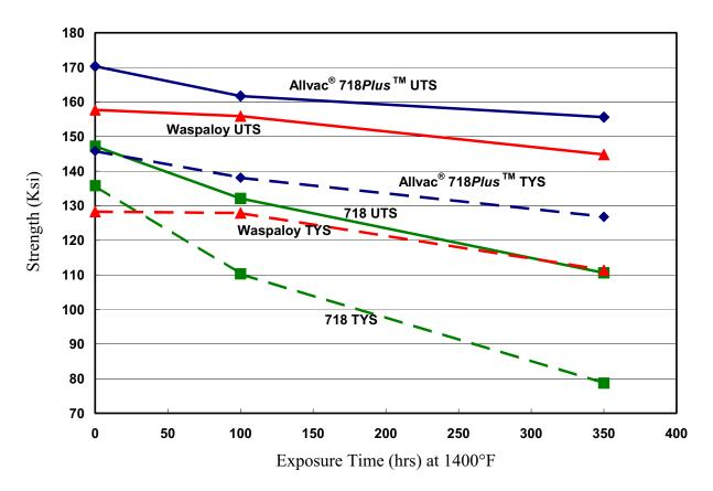
Figure 2. Effect of Thermal Exposure on Ultimate Tensile and Yield Strength at 1300°F
