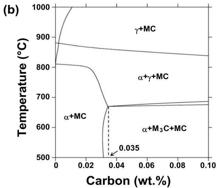
Figure 4. Phase diagram calculated using Thermo-calc (TCFE6 database);
