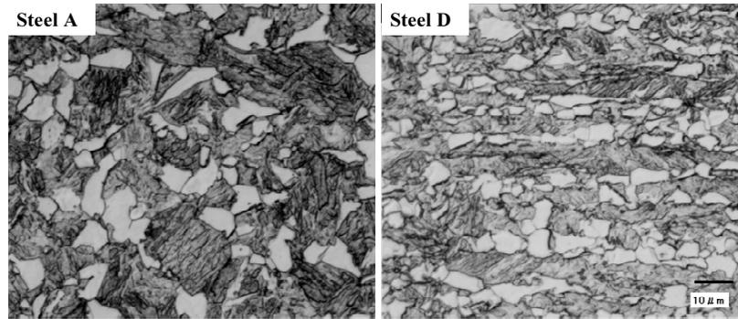
Figure 6. Effect of Nb on optical micrographs water quenched from 750°C.
