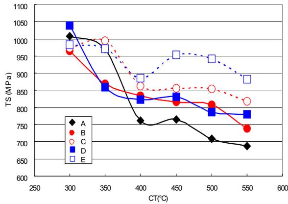
Figure 1. Effect of CT and alloying elements on TS.
