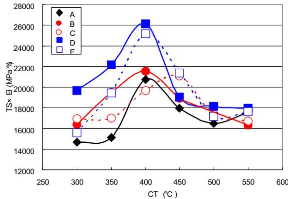
Figure 3. Effect of CT and alloying elements on TS and El balance expressed by TSxEl.
