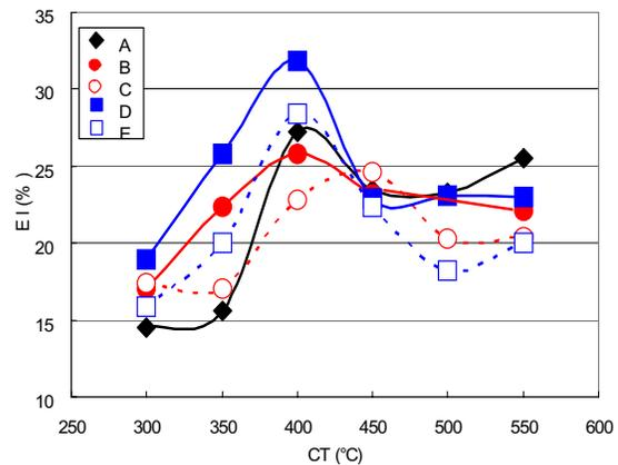
Figure 2. Effect of CT and alloying elements on El.
