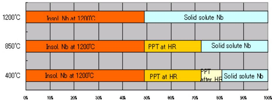
Figure 7. State of Nb in each stage of hot rolling process by chemical analysis.
