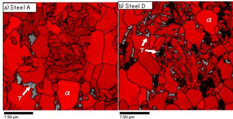
Figure 5. Effect of Nb addition on  $\gamma$  distribution observed by EBSD. ( $\gamma$ -phase is indicated by white and  $\alpha$ -phase is indicated by gray.)
