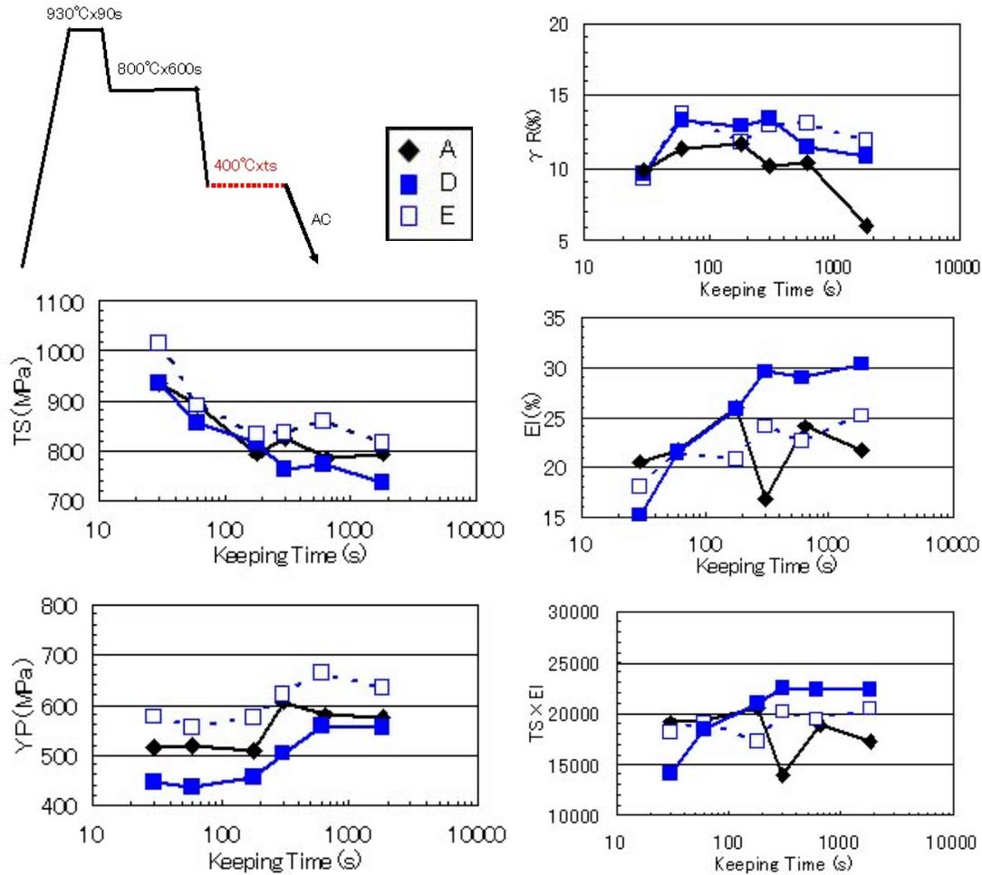
Figure 8. Effect of maintaining time at 400°C on TS, YP, EI, TS-EI balance (TSxEl) and volume fraction of retained austenite ( $\gamma_R$ ).
