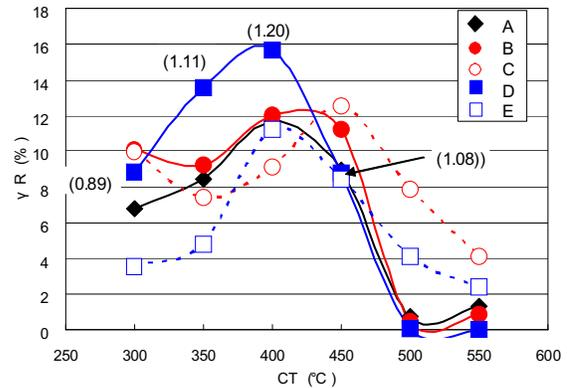
Figure 4. Effect of CT on volume fraction of retained austenite ( $\gamma$ R) and carbon concentration in retained austenite of steel D expressed in parenthesis.
