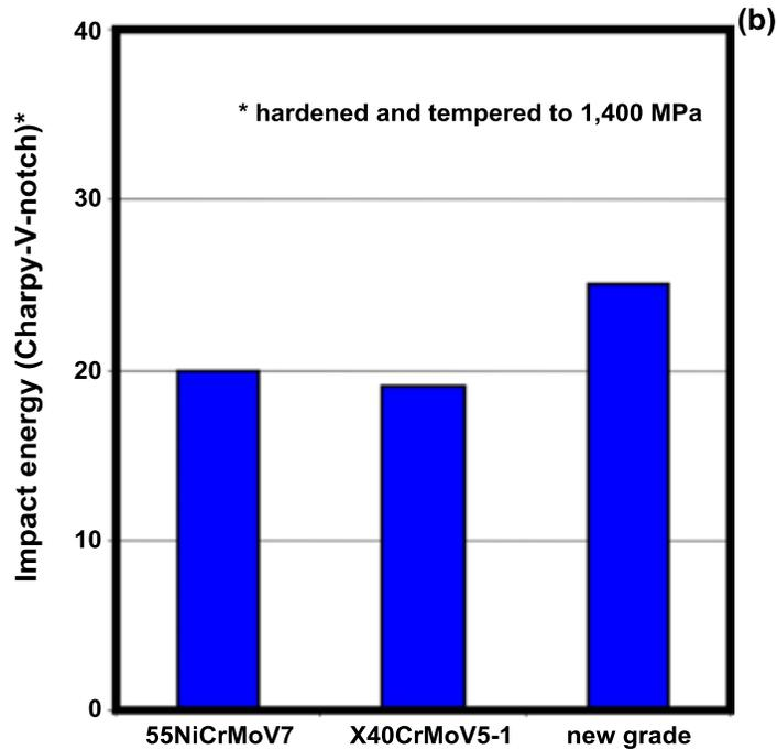
Figure 8. Yield strength and toughness of a new Nb microalloyed hot work steel in comparison to classical grades; (a) Yield strength, (b) Charpy toughness [12].
