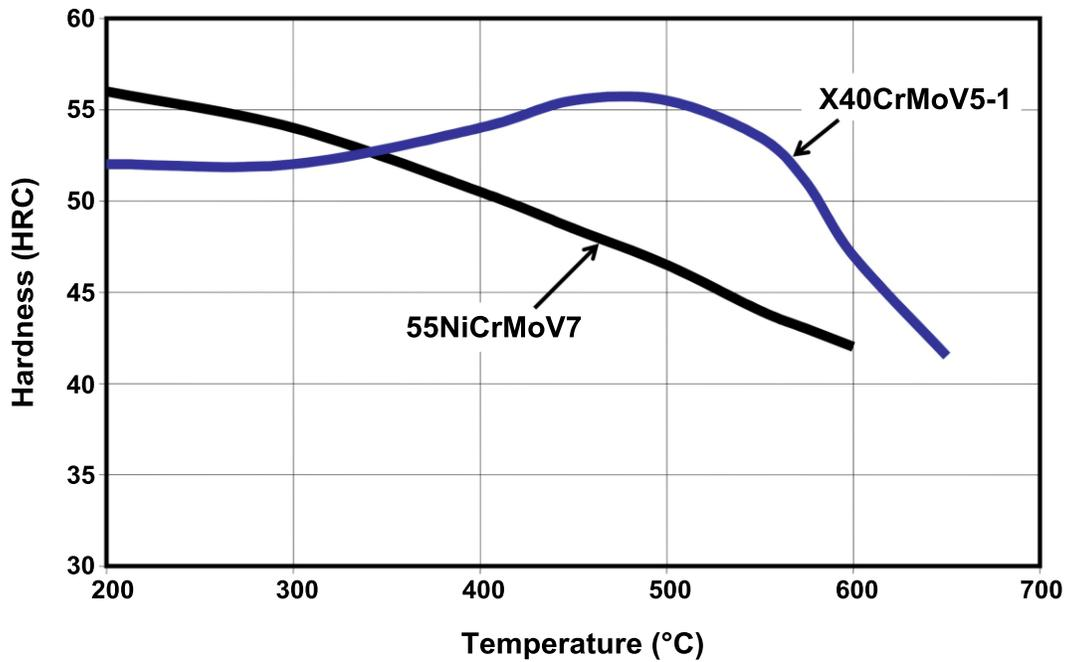
Figure 5. Tempering diagram of the hot work steels 55NiCrMoV7 and X40CrMoV5-1.
