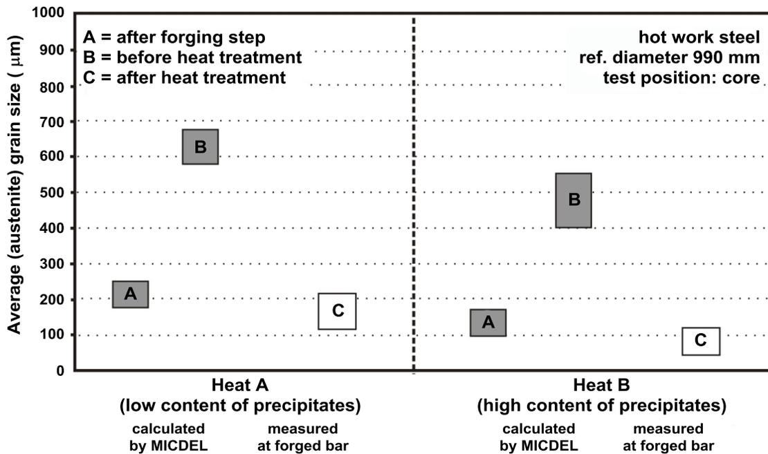
Figure 7. Calculated and measured grain sizes of a forged hot work steel block with different amount of precipitates [10].
