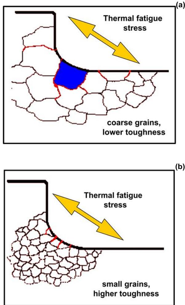
Figure 6. Effect of material toughness and grain size on thermal cracking of tools [6].
