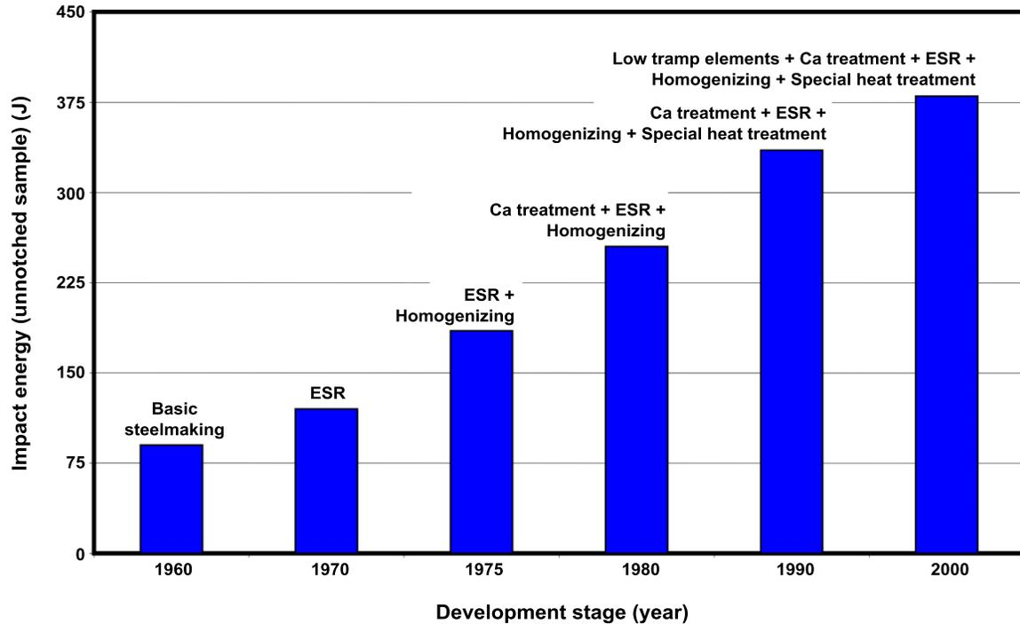
Figure 4. Measures in production of hot work steels to fulfill highest material toughness requirements [4].
