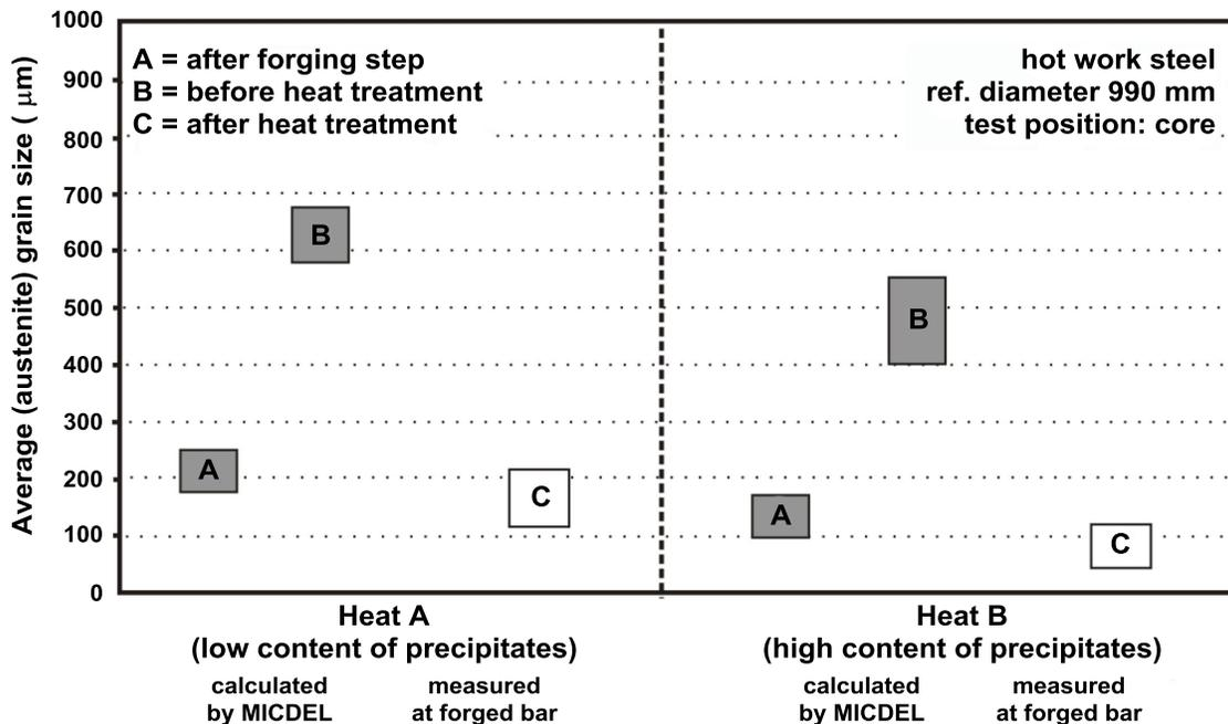
Figure 7. Calculated and measured grain sizes of a forged hot work steel block with different amount of precipitates [10].
