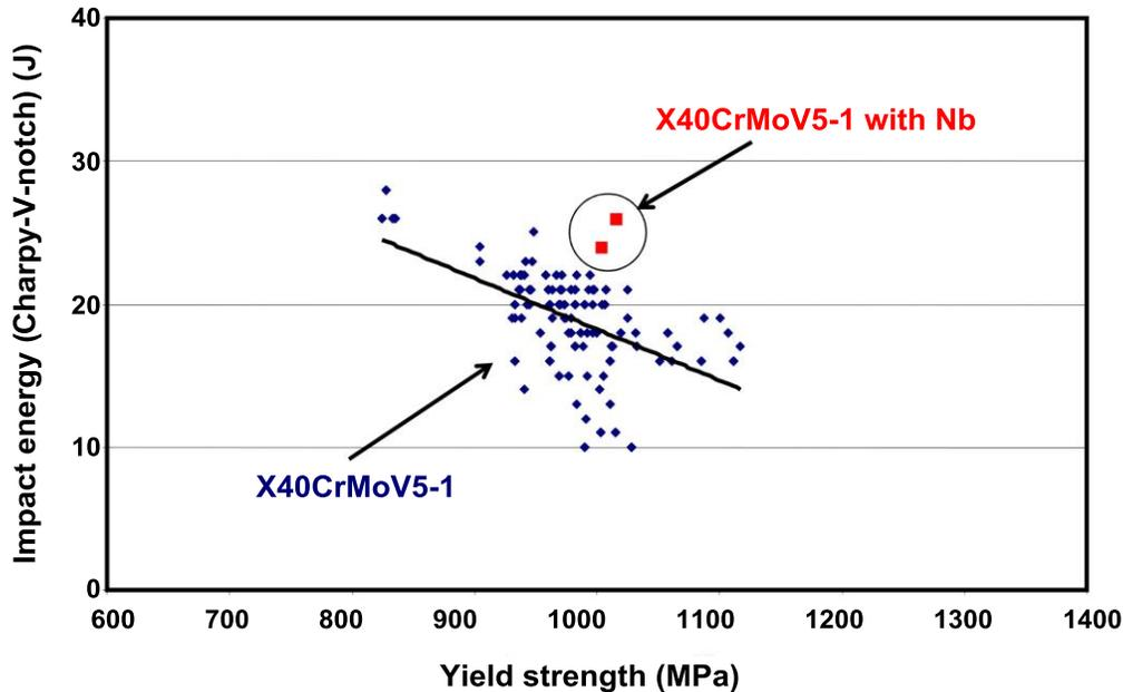
Figure 9. Results of mechanical testing steel bars in X40CrMoV5-1 for mandrels, toughness versus yield strength, in comparison with results for a Nb modified heat of the same grade.
