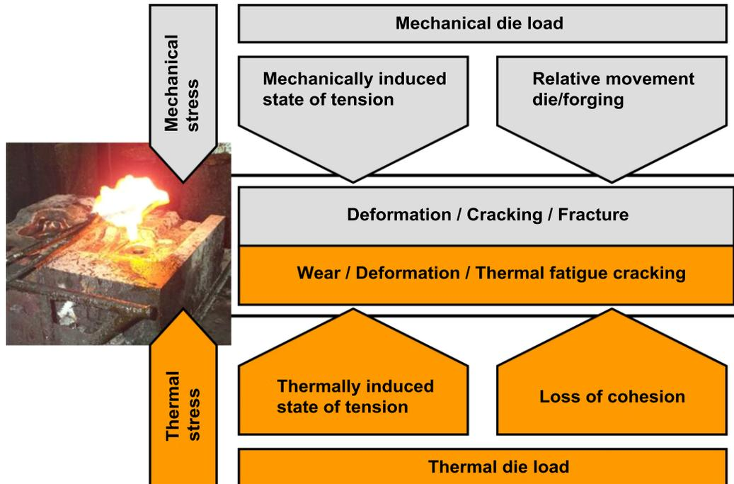
Figure 2. Load condition of a forging tool [2].
