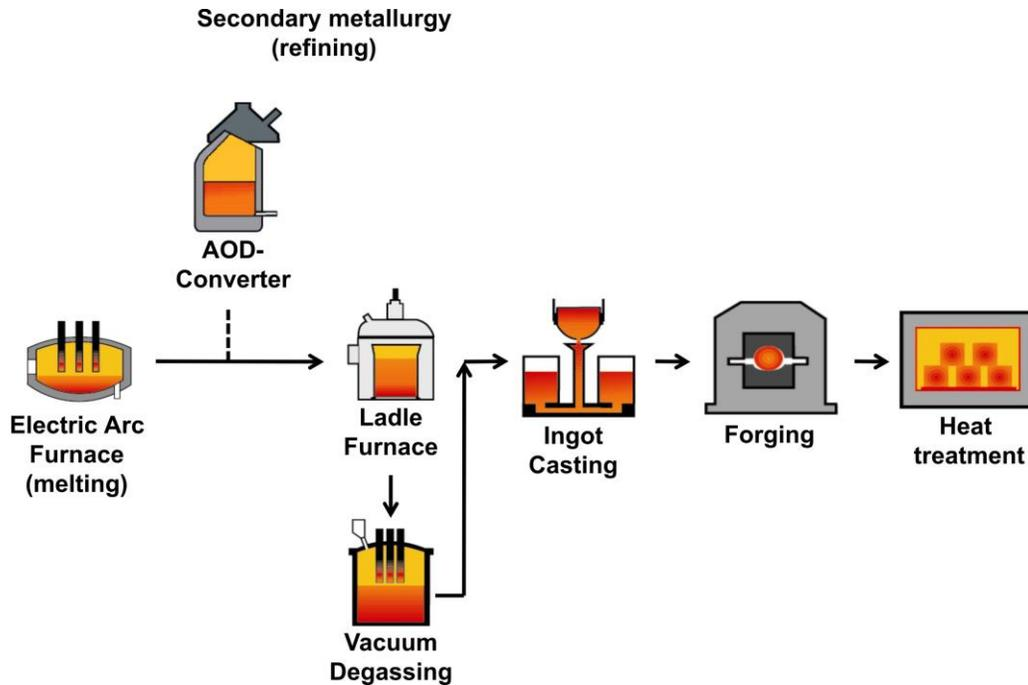
Figure 3. Process route for manufacturing forged tool steels.
