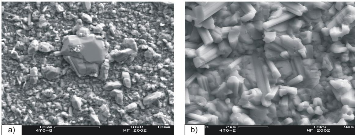
Figure 3: Top view scanning electron micrographs of nitride-2 coatings deposited onto a) Ti-45-8 and b) Ti-48-2-2 substrates. Specimens were isothermally oxidized in air at  $750^\circ\text{C}$  for 2200 h and 2000 h, respectively.
