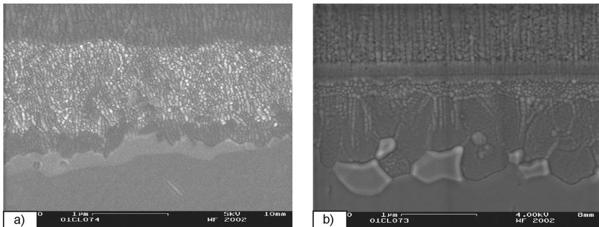
Figure 8. Scanning electron micrographs of Ti-45-8 (a) and Ti-48-2-2 (b) specimens coated with nitride-1, which were oxidized 3000 h at 750°C, showing the fine grained nitride layer of the transition zone.
