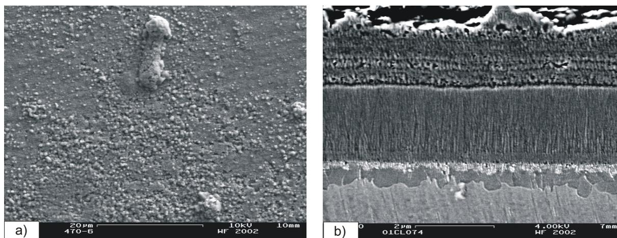
Figure 6: Scanning electron micrograph of a Ti-45-8 specimen coated with nitride-1, which was oxidized 3000 h at 750°C, showing a top view of the oxide scale (a) and a cross section through the oxide scale, nitride coating and substrate (b).
