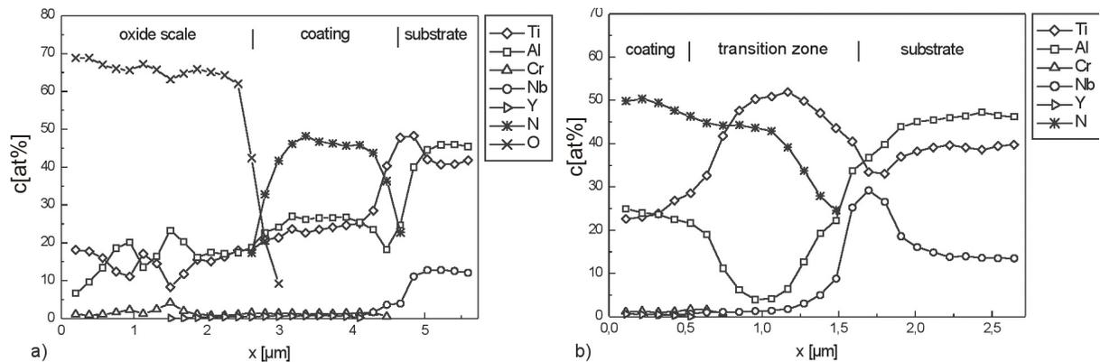
Figure 7: EDX analysis of Ti-45-8 specimen coated with nitride-1, which was oxidized 3000 h at 750°C, showing the concentration profiles across oxide scale, coating and substrate (a) as well as across the transition zone between nitride coating and substrate (b).
