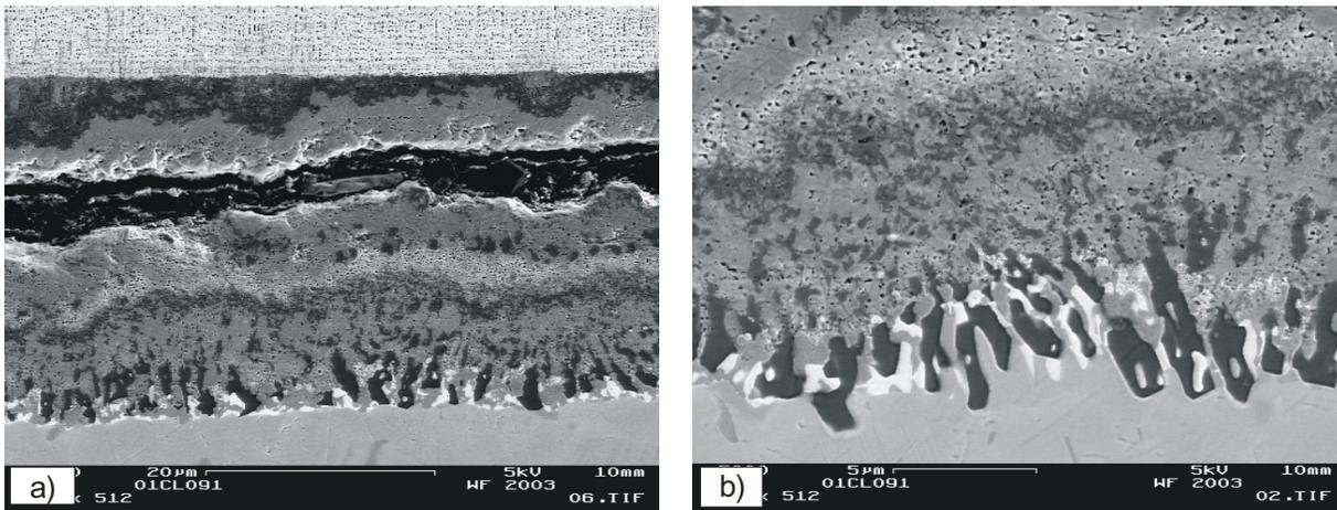
Figure 14: SEM micrograph of a specimen after 1000 1-h cycles at 900°C, showing the oxide scale (a) and the oxide/substrate interface (b).
