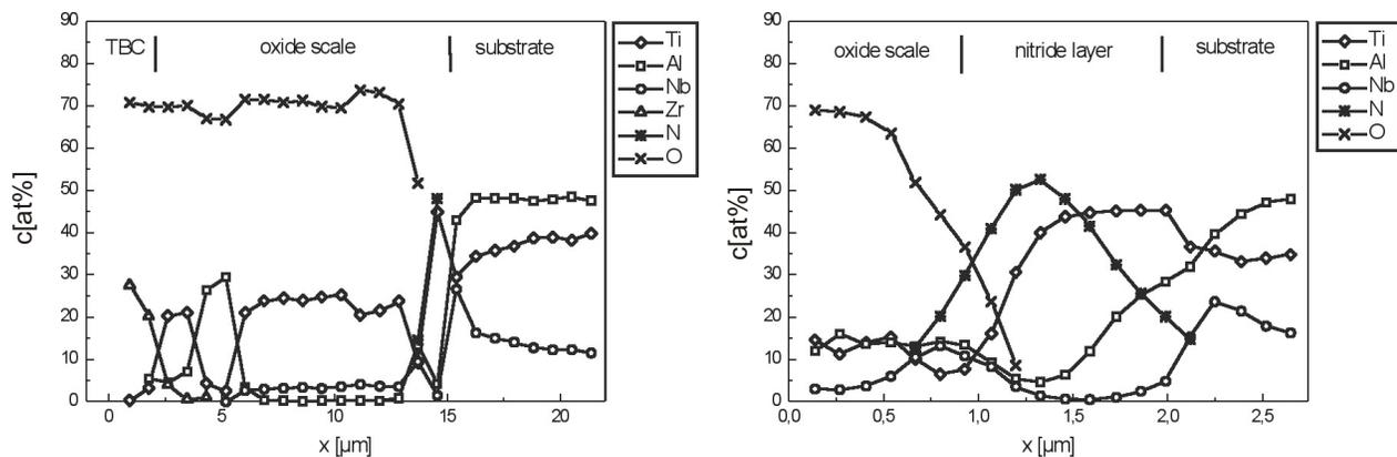
Figure 13: EDS analysis of a specimen after 1000 1-h cycles at 850°C, showing elemental profiles across the oxide scale (a) and the oxide/substrate interface (b).
