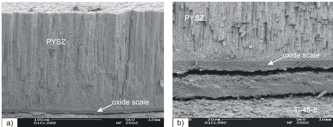
Figure 11: Typical failure location of an EB-PVD thermal barrier coating on Ti-45-8 after 250 1-h cycles at 950°C.
