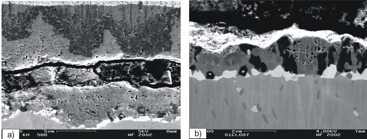
Figure 12: SEM micrograph of a specimen after 1000 1-h cycles at 850°C, showing the oxide scale (a) and the oxide/substrate interface (b).
