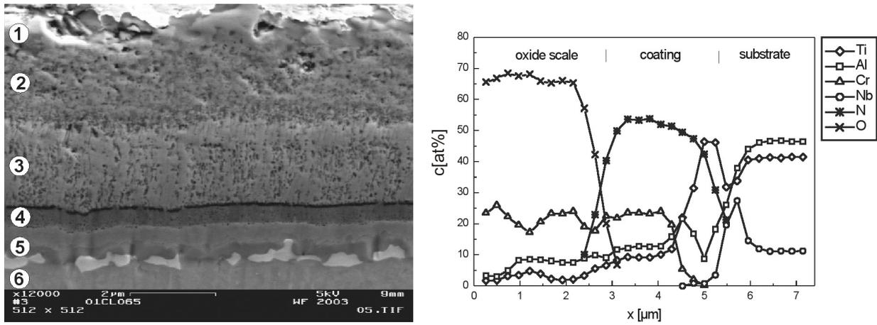
Figure 4: Scanning electron micrograph and EDX analysis of a Ti-45-8 specimen coated with nitride-2 which was oxidized for 2200 h at 750°C, showing a cross section view and the elemental profiles of the oxide scale (dense (1) and porous (2) part), nitride coating (3), base layer (4) and substrate (6). Clearly a transition zone (5) forms between the coating and the substrate.
