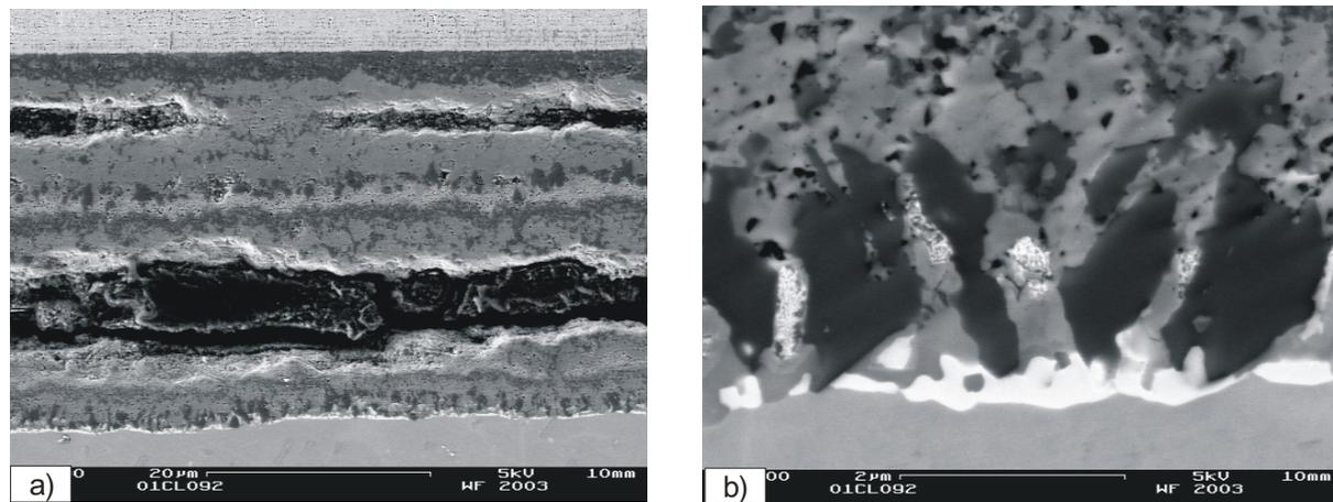
Figure 15: SEM micrograph of a specimen after 250 1-h cycles at 950°C, showing the oxide scale (a) and the oxide/substrate interface (b).
