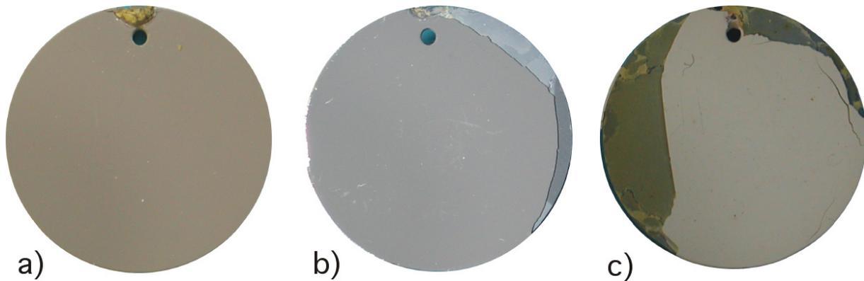
Figure 10: Photographs of TBC-2 specimens after cyclic oxidation. a) 850°C/1000h, b) 900°C/1000h, and 950°C/250h.
