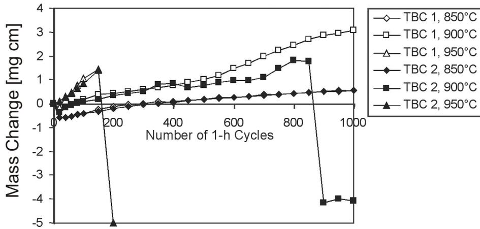
Figure 9: Performance of two different types of EB-PVD thermal barrier coatings on gamma titanium aluminide alloy Ti-45-8 between 850 and 950°C.
