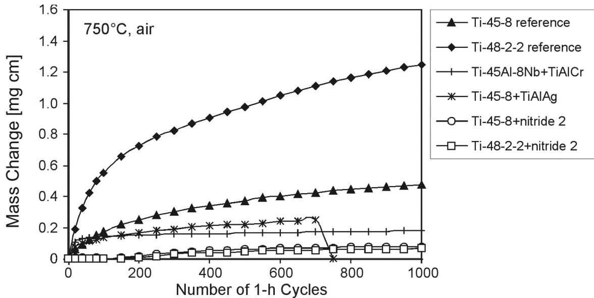
Figure 2: Cyclic oxidation behavior of reference and coated gamma titanium aluminide alloys Ti-48-2-2 and Ti-45-8.
