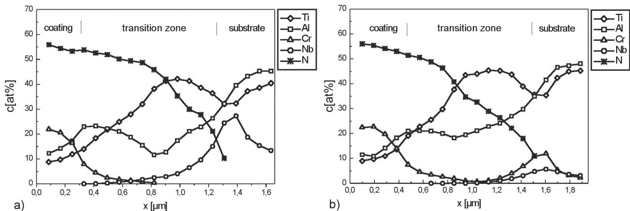
Figure 5: EDX analysis of Ti-45-8 (a) and a Ti-48-2-2 (b) specimens coated with nitride-2, which were oxidized at 750° C for 2200 h and 2000 h, respectively, showing elemental profiles across the transition zone between coating and substrate.
