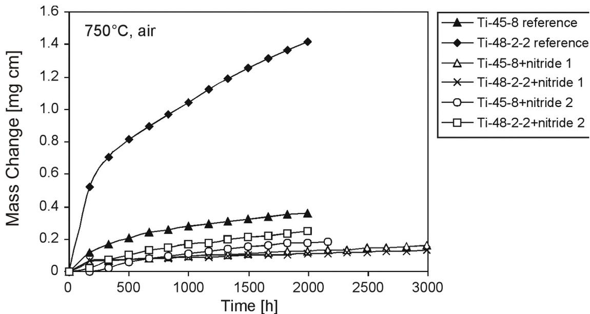
Figure 1: Quasi-isothermal oxidation behavior of reference and coated gamma titanium aluminide alloys.
