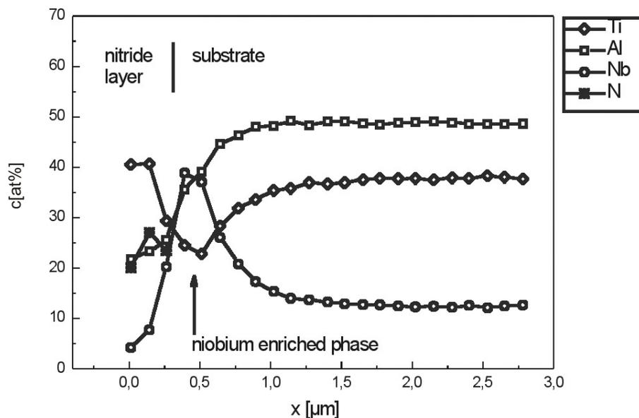
Figure 16: EDS analysis of a specimen after 250 1-h cycles at 950°C, showing transition between nitride layer and substrate.
