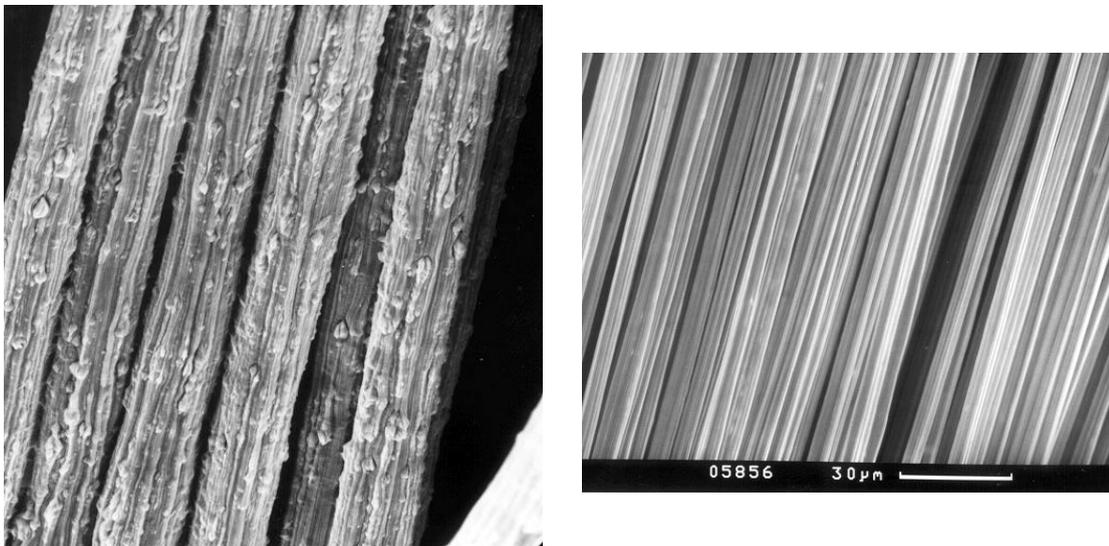
Figure 3: Quality of NbTi filaments. Left: Filaments without Nb barrier with hard intermetallic particles. Right: Improved filament quality by applying Nb barriers around each filament.
