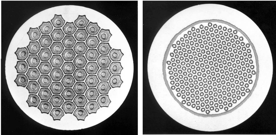
Figure 5: Examples of  $\text{Nb}_3\text{Sn}$  multifilamentary conductors. Left: Internal Sn conductor. Each bundle consists of a Sn source and a filamentary area surrounded by a diffusion barrier. The total array is imbedded in a Cu matrix. Right: Bronze route conductor, consisting of a number of filament bundles imbedded in a bronze matrix surrounded by a diffusion barrier and Cu stabilizer outside of the barrier.
