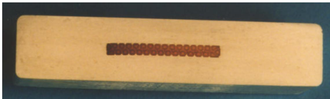
Figure 11: Superconducting cable for the ATLAS detector consisting of 38 strands with 1.3 mm diameter, co-extruded with ultra-pure Al, outer dimension 57 x 12 mm<sup>2</sup>, critical current 60 kA at 5T and 4.2K.
