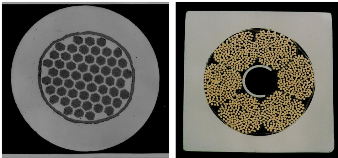
Figure 9: Conductor of ITER. Left: Basic Nb<sub>3</sub>Sn strand (0.8 mm diameter). Right: CiCC with central cooling channel and special steel conduit (50 x 50 mm<sup>2</sup>).
