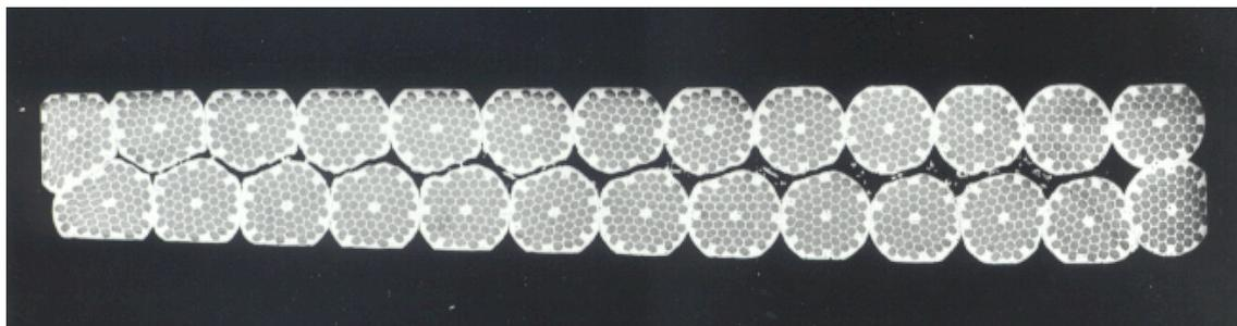
Figure 10: Superconducting cable for the LHC dipoles consisting of 26 strands with 1.06 mm diameter and 8670 filaments with 7 $\mu\text{m}$  diameter (Fig. 2, right).
