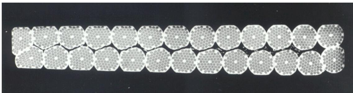
Figure 10: Superconducting cable for the LHC dipoles consisting of 26 strands with 1.06 mm diameter and 8670 filaments with 7 $\mu\text{m}$  diameter (Fig. 2, right).
