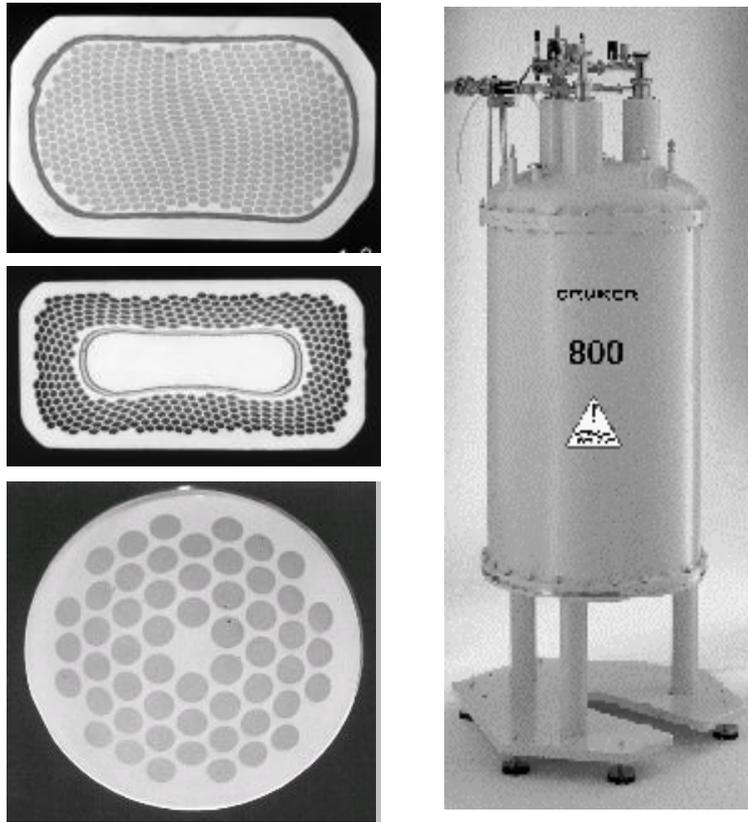
Figure 7: Nuclear Magnetic Resonance. Left: Typical superconductors for NMR magnets (From bottom to top NbTi standard conductor, Nb<sub>3</sub>Sn with internal Cu stabilization and with external Cu stabilization). Right: NMR Magnet cryostat.
