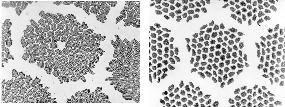
Figure 4: Cross sectional view of the filamentary area of bronze route  $Nb_3Sn$  conductors after reaction heat treatment. The reacted  $Nb_3Sn$  layer and the unreacted Nb core can clearly be distinguished (filament diameter about 4  $\mu m$ ). Left: Due to the growth of the filament area during reaction there is an intergrowth of the filaments within one bundle. Right: Intergrowth of filament avoided by large filament spacing.
