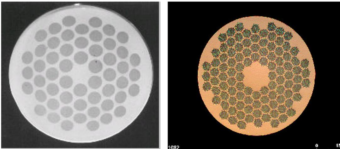
Figure 2: Examples of NbTi/Cu multifilamentary conductors. Left: Standard conductor with 54 filaments. Right: Fine filament conductor with 8670 filaments produced by a two stage bundling process.
