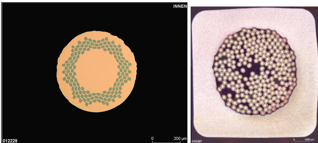
Figure 8: Conductor of W7X. Left: Basic NbTi strand (0.57 mm diameter) Right: CiCC with Al-alloy conduit (16 x 16 mm<sup>2</sup>).
