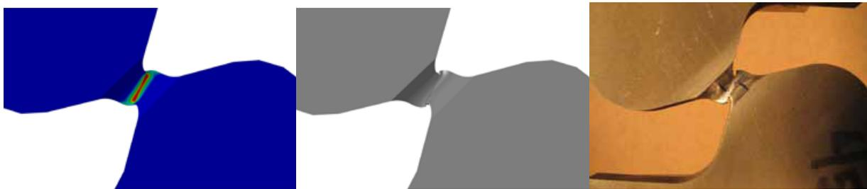
Figure 5. FEA and Physical Specimen Failure Comparison
