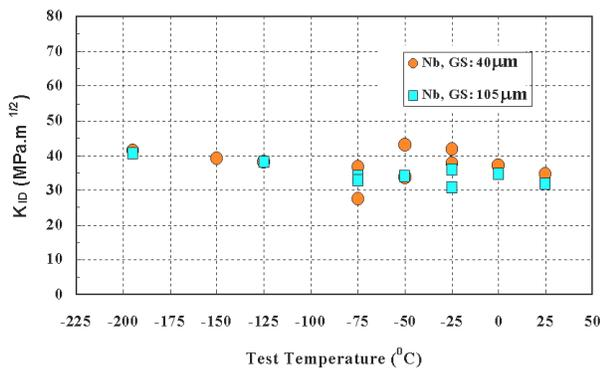
Figure 8. Grain size and test temperature effects on dynamic fracture toughness,  $K_{ID}$ , of Nb [24].
