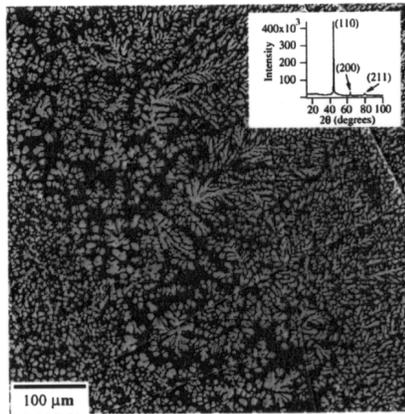
Figure 17. Bulk metallic glass composite containing a Nb-Ti-Zr crystalline phase designed to impart enhanced ductility and toughness [4,6-8].
