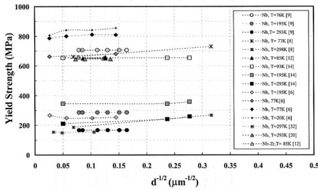
Figure 1. Effects of changes in grain size on yield strength of polycrystalline Nb and Nb alloys [5,13].
