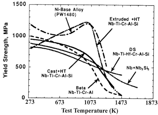
Figure 5. Effects of test temperature on strength of monolithic Nb alloys and Nb Silicide composites [18-21].
