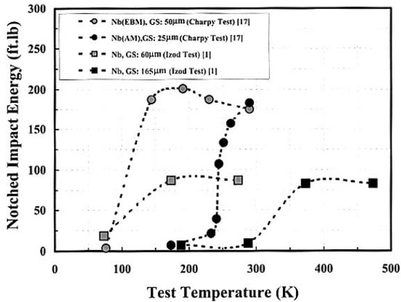
Figure 6. Effects of changes in grain size and processing conditions on impact energy and DBTT of Nb [12].
