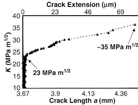
Fig. 12. Typical R curve of Nb silicide, showing an initiation toughness of  $23 \text{ MPa m}^{1/2}$  and a peak toughness of  $\sim 35 \text{ MPa m}^{1/2}$ . Similar behavior was observed in investment-cast Nb silicide [3].
