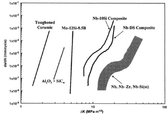
Figure 16. Comparison of fatigue behavior of some high temperature materials [25-30].
