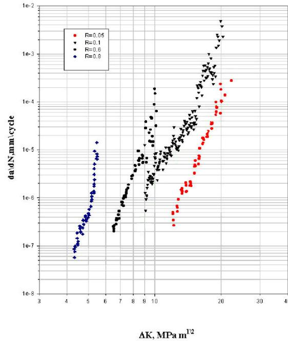
Figure 14. Effects of changes in stress ratio on fatigue of Nb-10 a/o Si composites.
