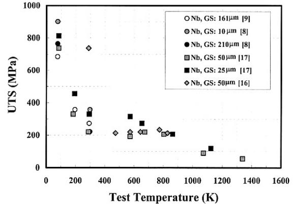
Figure 4. Effects of changes in test temperature on UTS of polycrystalline Nb and Nb alloys [22].
