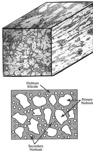
Figure 10. Typical microstructure of arc cast/extruded Nb-10 a/o Si alloy [9, 16].
