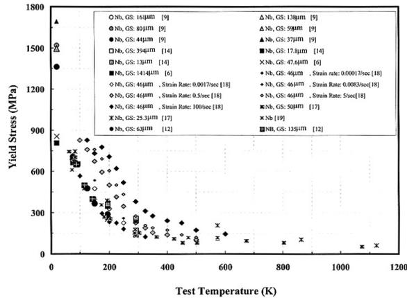
Figure 3. Effects of changes in test temperature on yield stress of Nb and Nb alloys [5,13].
