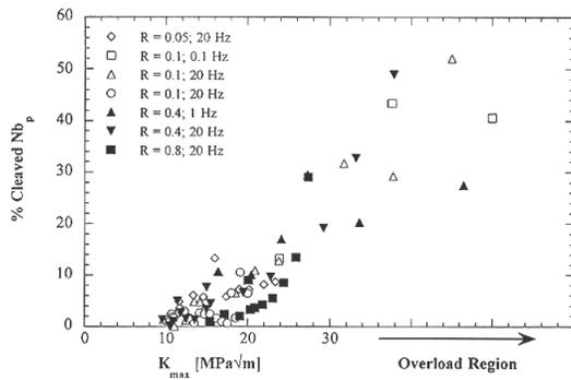
Figure 15. Quantitative fractography results showing an increase in amount of cleaved primary Nb with increasing  $K_{max}$  in Nb-10 a/o Si composites.
