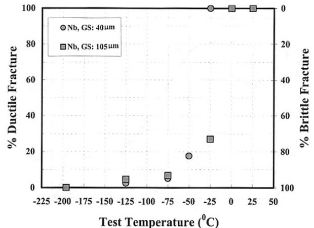
Figure 7. Effects of changes in grain size on DBTT and fracture surface appearance of Nb [22].
