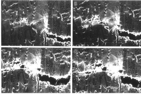
Figure 11. In-situ fracture experiment showing crack impingement on tough Nb in Nb-10 a/o Si composite increasing load from A-D [16,32].
