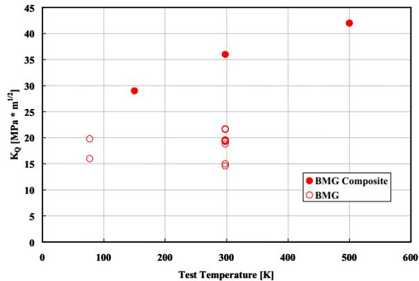
Figure 18. Effects of changes in test temperature on fracture toughness of a bulk metallic glass and bulk metallic glass composite containing a Nb-Ti-Zr crystalline phase [5].
