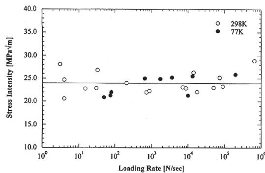
Figure 13. Effects of changes in loading rate and test temperature on toughness of Nb-10 a/o Si composite [16].
