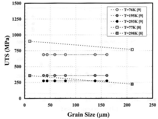
Figure 2. Effects of changes in grain size on UTS of polycrystalline Nb and Nb alloys [5,13].
