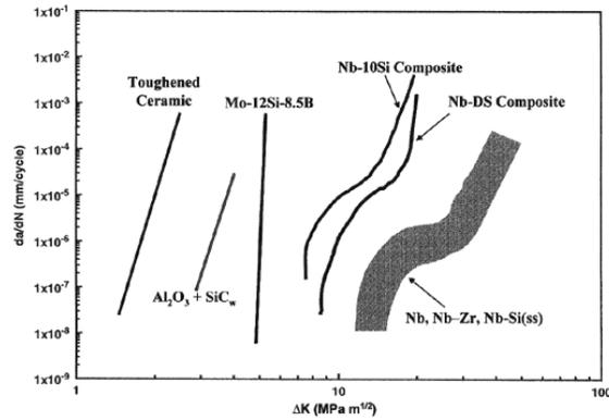
Figure 16. Comparison of fatigue behavior of some high temperature materials [25-30].
