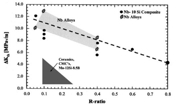
Figure 9. Summary of effects of changes in stress ratio on fatigue threshold of a variety of high temperature materials [3,13,25-30] tested at 298K.
