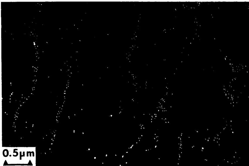
Figure 31 - Strain-induced precipitation of NbCN in austenite in a steel containing .09 percent C - .07 percent Nb. Specimen reheated at 1250 C, rolled 25 percent and held at 950 C, and air cooled to RT. Centered dark field electron micrograph using a (111) NbC reflection. After Santella (69).
