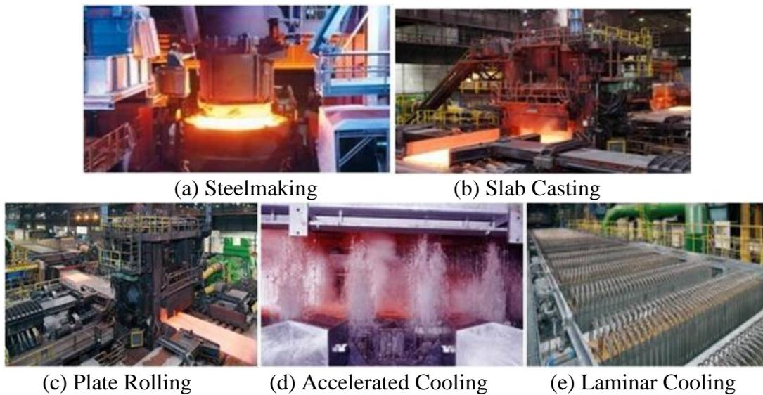
Figure 2. (a – e) Steelmaking, Casting, Rolling and Cooling Facilities at voestalpine.
