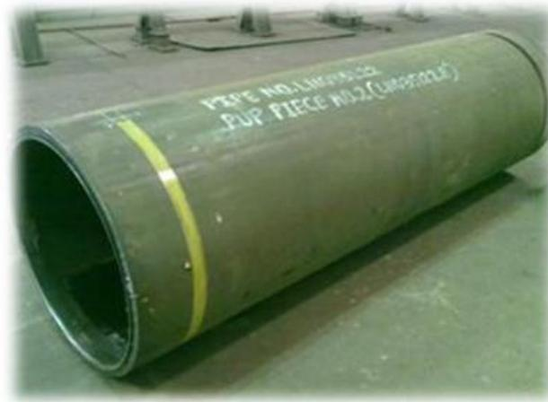
Figure 1. Thick wall sour service pipe.
