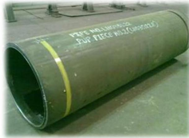
Figure 1. Thick wall sour service pipe.
