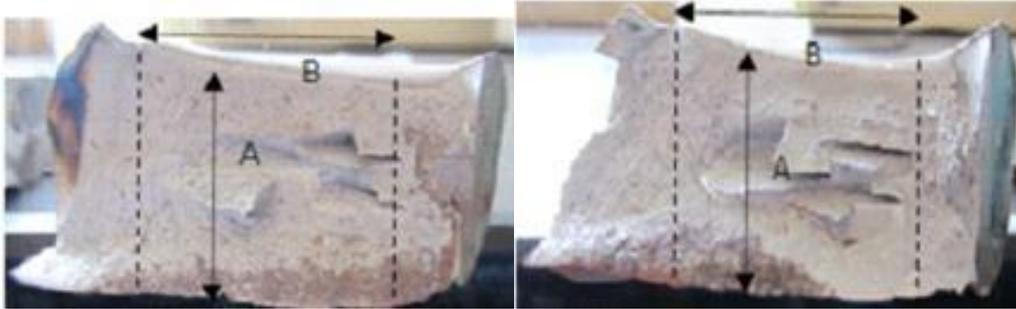
Figure 9. DWTT Shear area in pipe at -17 °C (Reduced size).
