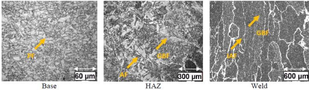
Figure 12. Microstructure variation from base metal to HAZ to the weld.
