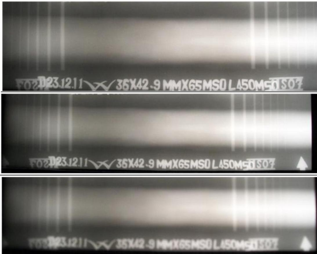
Figure 8. Photographs of real time radiography of weld seam.
