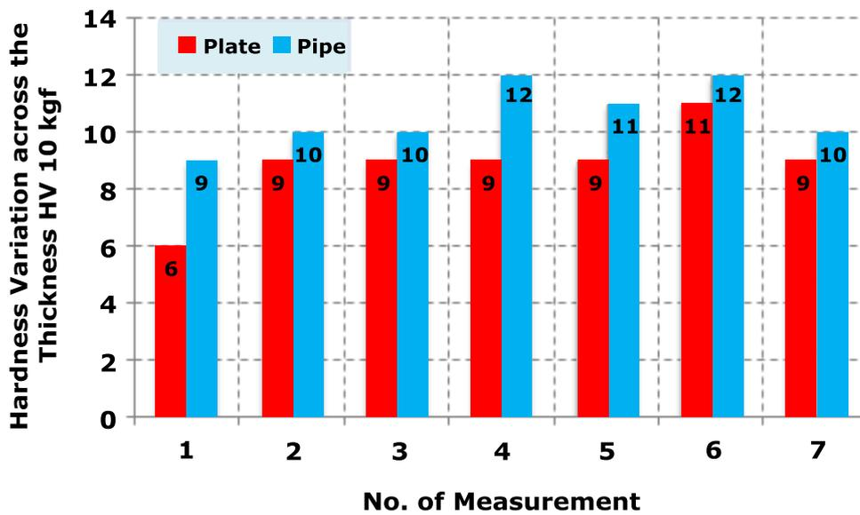
Figure 13. Hardness variation across the thickness in plate and pipe (base material).
