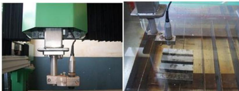
Figure 18. Immersion ultrasonic testing setup from GE Energy Inspection Technologies.
