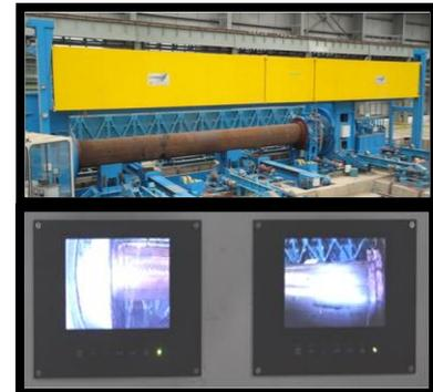
(l) Hydrostatic Testing
