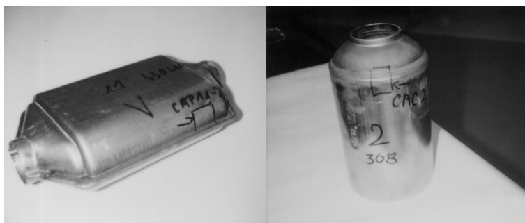
Figure 13. Fillet welds on Faurecia catalysts: (a) straight weld on an AISI 409 racetrack type catalytic converter can; (b) circular weld on an AISI 441 cylindrical catalytic converter can.
