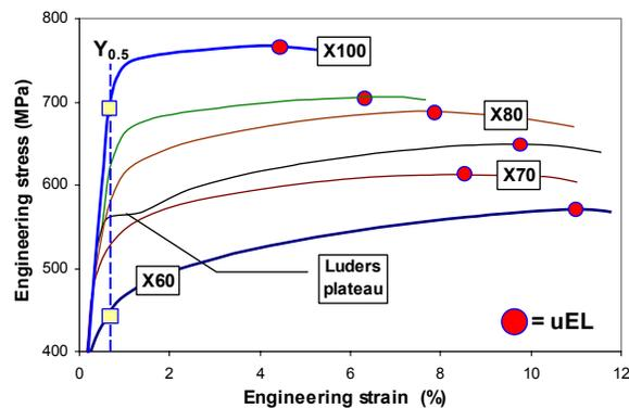
**Figure 4. Effect of steel grade (X60 – X100) on stress strain response and uniform elongation, uEL.**
