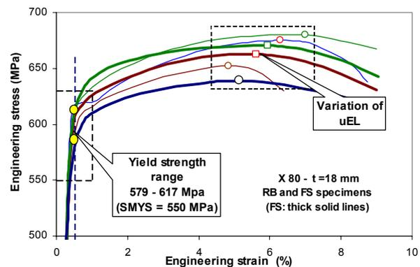
**Figure 5. Effect of specimen geometry and sampling location on tensile stress-strain behaviour of grade X80 pipe [50]**
