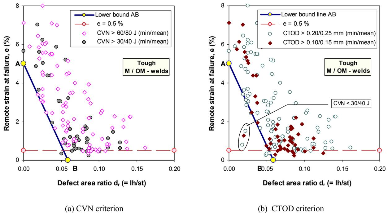
Figure 2. Variation of overall remote strain,  $e$ , with defect area ratio,  $d_r$ , in overmatched welds as a function of CVN or CTOD toughness (see insert to the plots).
