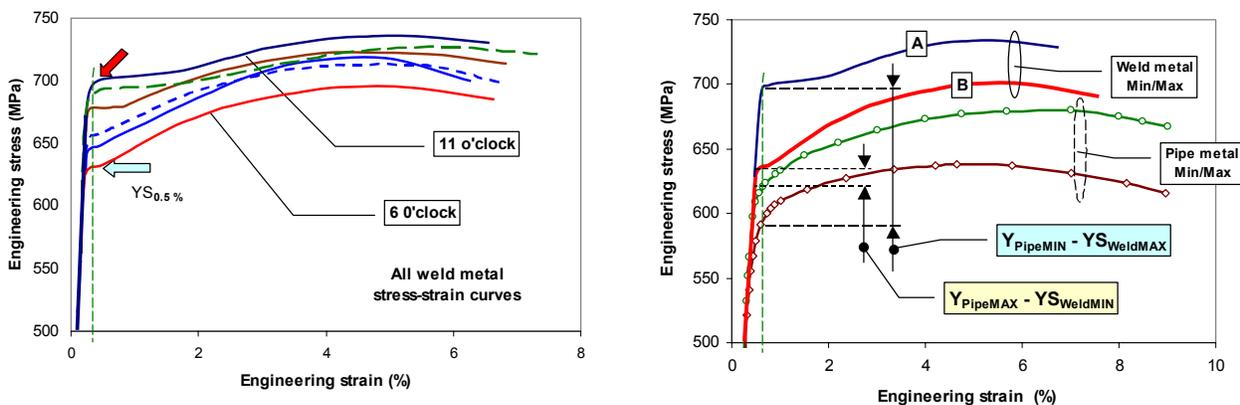
(a) – Weld metal stress-strain curves
