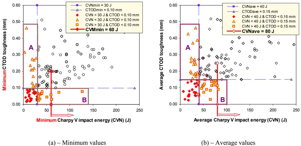
Figure 3. Variation of Charpy V Notch impact energy and CTOD properties of the girth weld metals at wide plate test temperature.
