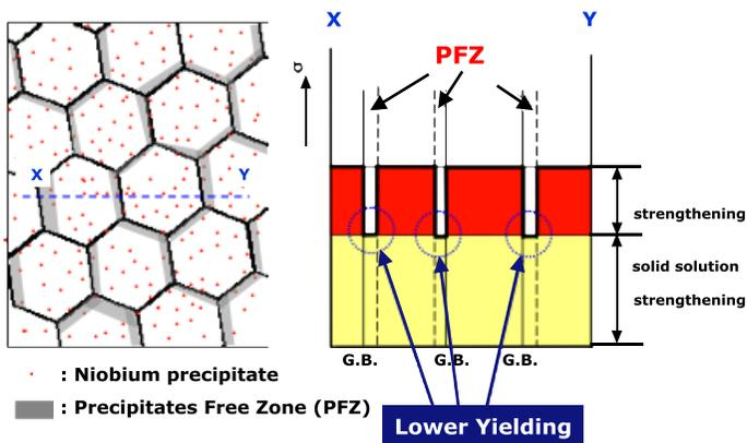
Figure 5. Mechanism of providing low yield strength.
