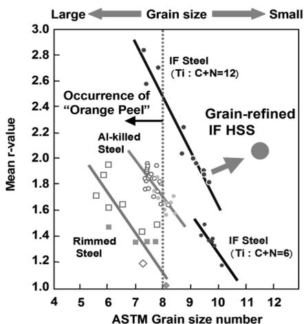
Figure 2. Correlation between ASTM grain size number and mean r-values of cold-rolled steel sheets.
