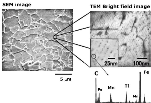
Figure 8. Typical microstructure of 780 MPa class hot-strip, hardened by nano-scale interphase precipitates.
