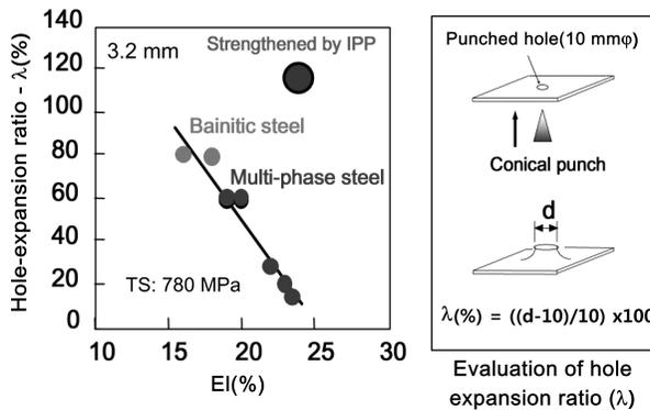
Figure 7. Outstanding EI- λ balance of hot-band strengthened by interphase precipitation (IPP).
