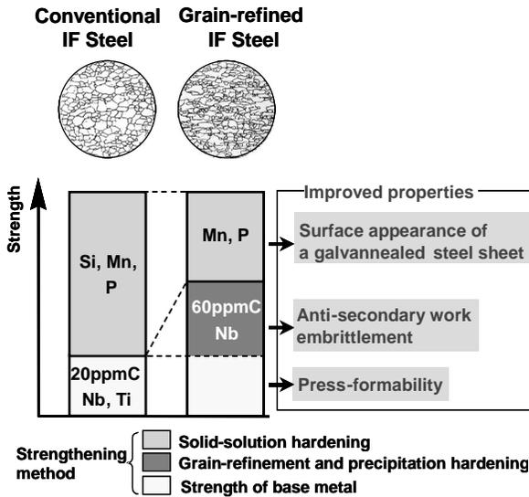
Figure 1. Schematic diagram showing the metallurgical concept of the newly developed steel compared to the conventional IF steel.
