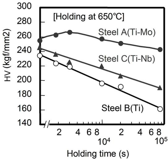
Figure 11. Softening behavior of three types of steels after isothermal holding at 650 °C.
