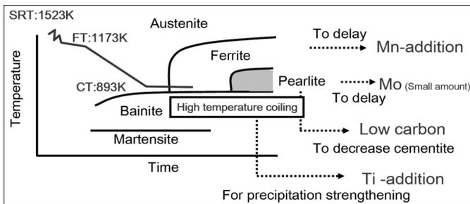
Figure 6. Schematic CCT diagram of alloy design and on-line microstructure control.
