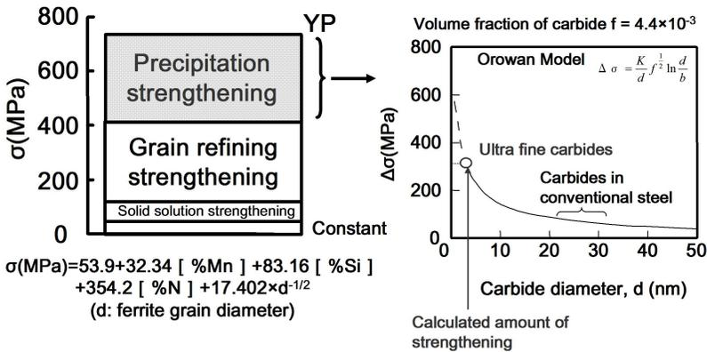
Figure 10. Strengthening of ferrite matrix by nano size fine carbides.
