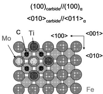
Figure 9. Lattice structure of precipitates and crystallographic relationship with ferrite matrix.
