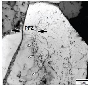
Figure 4. TEM micrograph of specimen deformed with 0.5% tensile strain [18].
