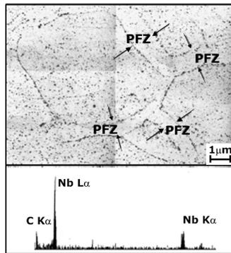
Figure 3. TEM image from replica and EDS spectra of precipitates, observed in the annealed sheet of 390 MPa grade of grain-refined IF HSS [10].
