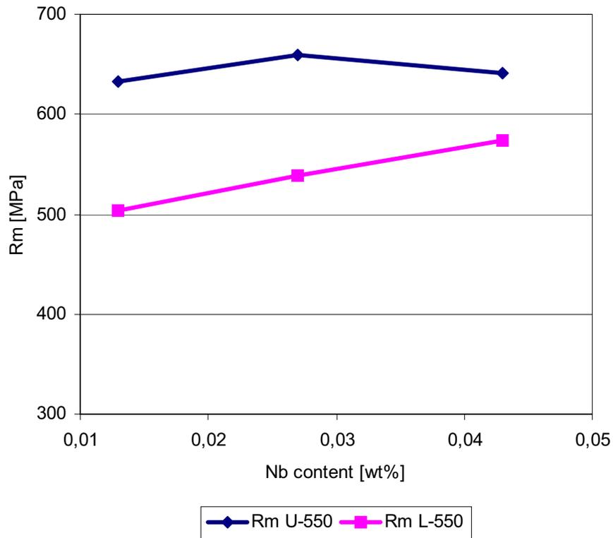
Figure 18. Tensile strength  $R_m$  vs. Nb content, for UFC and laminar cooling down to 550°C coiling temperature.
