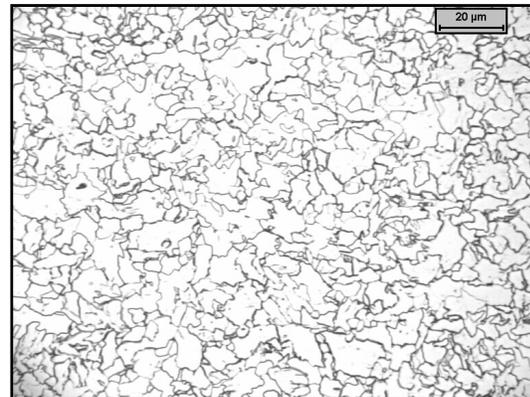
Figure 37. Microstructure of Alloy K after ultra fast cooling down to a coiling temperature of  $650^{\circ}\text{C}$ .
