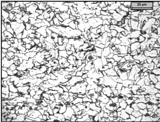
Figure 21. Microstructure of Alloy F after laminar cooling down to a coiling temperature of 550°C.
