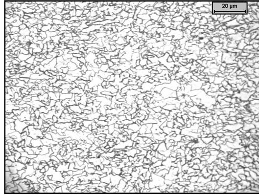
Figure 39. Microstructure of Alloy L after ultra fast cooling down to a coiling temperature of 650°C.
