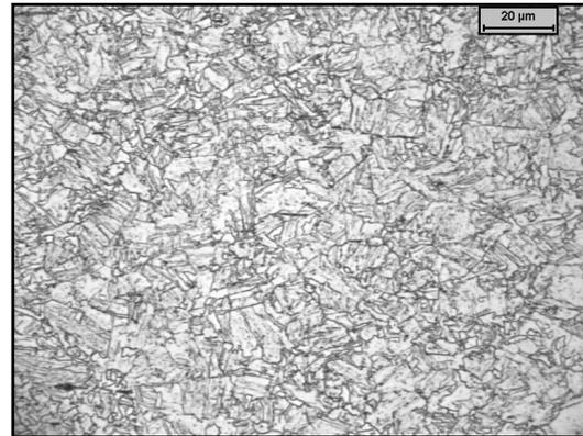
Figure 22. Microstructure of Alloy F after ultra fast cooling down to a coiling temperature of 550°C.
