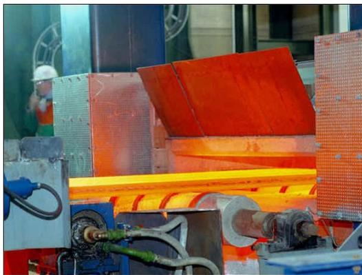
Figure 4. The entry to the tunnel furnace.
