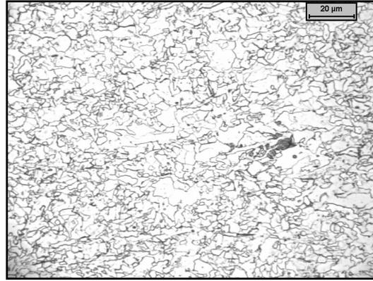
Figure 32. Microstructure of Alloy H after ultra fast cooling down to a coiling temperature of 650°C.
