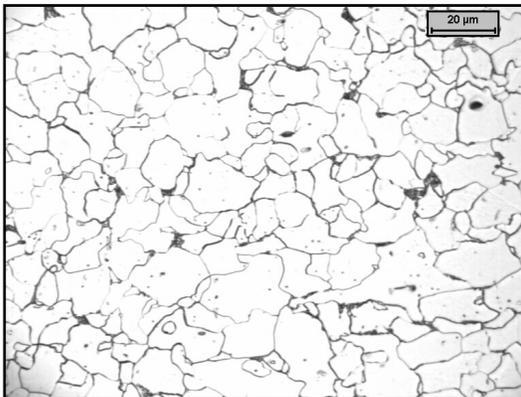
Figure 36. Microstructure of Alloy K after laminar cooling down to a coiling temperature of  $650^{\circ}\text{C}$ .
