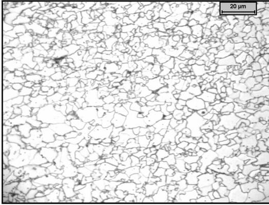
Figure 38. Microstructure of Alloy L after laminar cooling down to a coiling temperature of 650°C.
