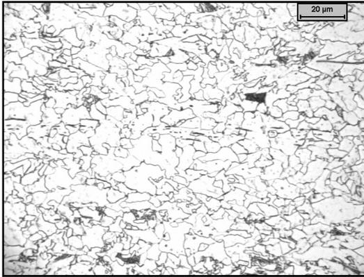
Figure 27. Microstructure of Alloy G after laminar cooling down to a coiling temperature of 650°C.
