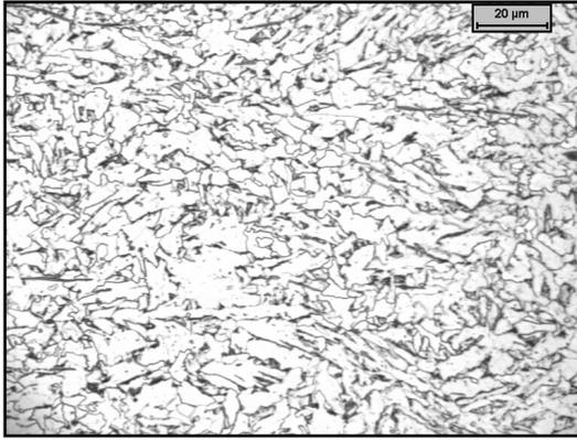
Figure 25. Microstructure of Alloy G after laminar cooling down to a coiling temperature of 550°C.
