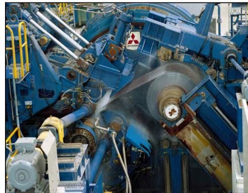
Figure 9. The Carrousel coiler.
