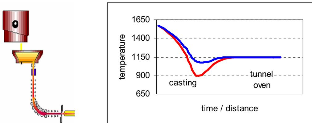
Figure 11. Casting section of the DSP and typical temperature profiles of the continuous slab, in the case of normal operation (blue curve) and in the case of reduced casting speed (red curve).
