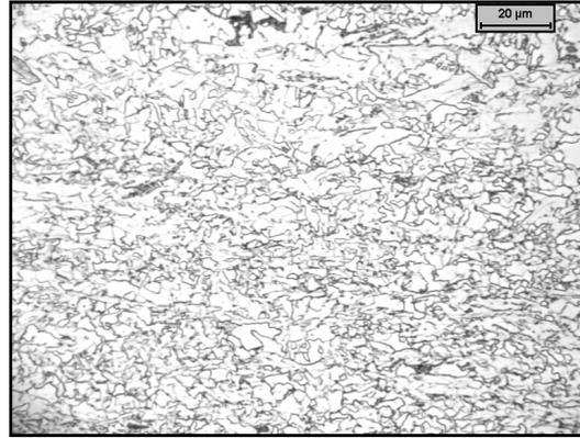
Figure 45. Microstructure of Alloy O after ultra fast cooling down to a coiling temperature of 650°C.
