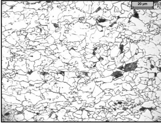
Figure 44. Microstructure of Alloy O after laminar cooling down to a coiling temperature of 650°C.
