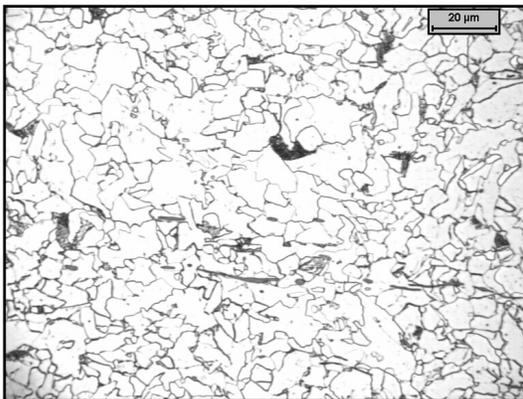
Figure 23. Microstructure of Alloy F after laminar cooling down to a coiling temperature of 650°C.
