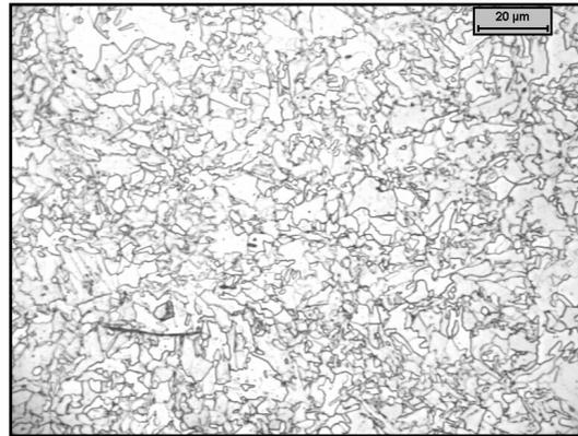
Figure 43. Microstructure of Alloy N after ultra fast cooling down to a coiling temperature of 650°C.
