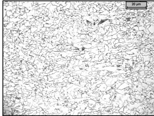
Figure 28. Microstructure of Alloy G after ultra fast cooling down to a coiling temperature of 650°C.
