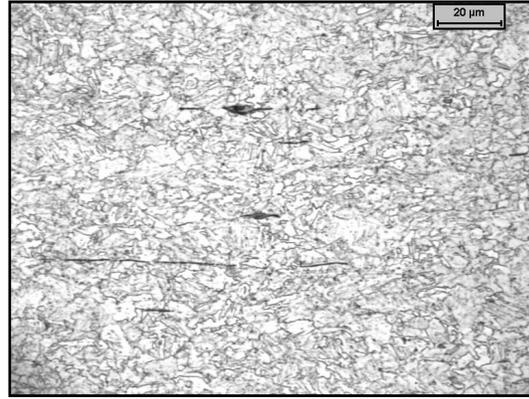
Figure 26. Microstructure of Alloy G after ultra fast cooling down to a coiling temperature of 550°C.
