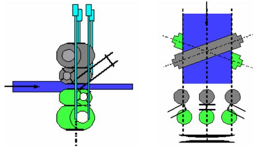
Figure 7. The principle of pair crossing.
