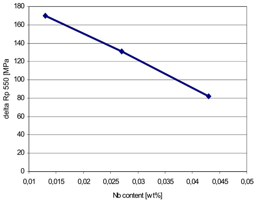
Figure 19. Yield stress gain  $\Delta R_p$  of UFC vs. Nb content at 550°C coiling temperature.
