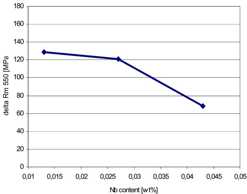
Figure 20. Tensile strength gain  $\Delta R_m$  of UFC vs. Nb content at 550°C coiling temperature.
