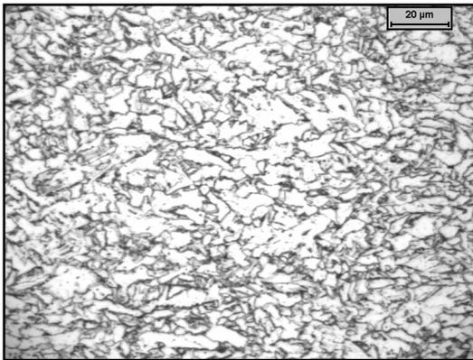
Figure 29. Microstructure of Alloy H after laminar cooling down to a coiling temperature of 550°C.
