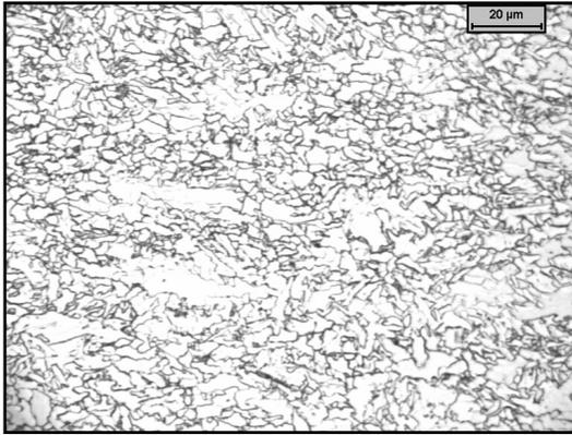
Figure 40. Microstructure of Alloy M after laminar cooling down to a coiling temperature of 650°C.
