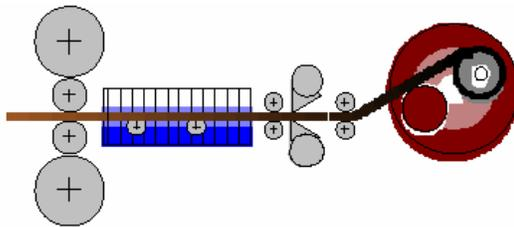
Figure 8. Schematic of ultra fast cooling table, flying shear and carousel coiler.
