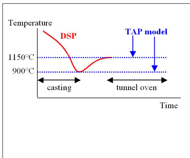
Figure 12. Schematic Representation of Time and Temperature for the TAP model. The red line indicates a typical time-temperature profile for DSP slabs cast at reduced speed.
