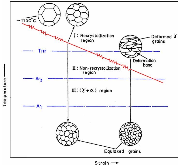
Figure 10. Schematic of the effect of  $T_{NR}$  on microstructures during hot rolling.
