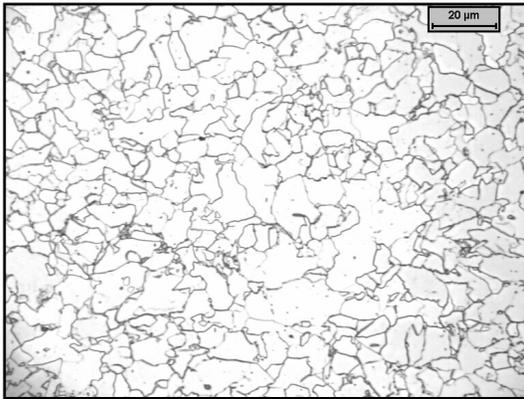
Figure 42. Microstructure of Alloy N after laminar cooling down to a coiling temperature of 650°C.
