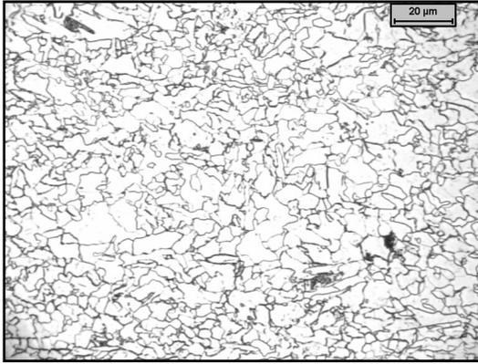
Figure 31. Microstructure of Alloy H after laminar cooling down to a coiling temperature of 650°C.
