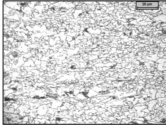
Figure 41. Microstructure of Alloy M after ultra fast cooling down to a coiling temperature of 650°C.
