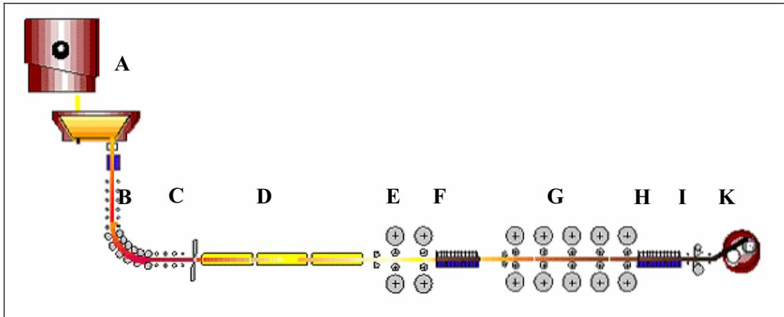
Figure 1. Schematic drawing of the DSP process, starting with the casting section (A), bending to horizontal (B), crop shear (C), tunnel oven (D), roughing stands (E), intermediate cooling (F), finishing stands (G), ultra fast cooling table (H), flying shear (I) and carousel coiler (K).
