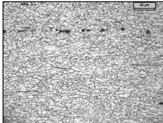
Figure 30. Microstructure of Alloy H after ultra fast cooling down to a coiling temperature of 550°C.
