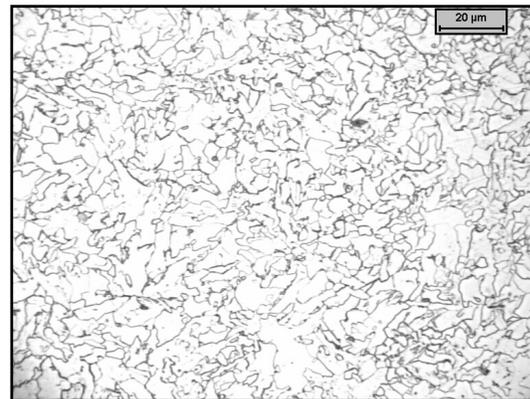
Figure 24. Microstructure of Alloy F after ultra fast cooling down to a coiling temperature of 650°C.
