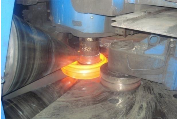
Figure 1: Ring-rolling of a contoured ring. (Frisa Aerospace SA de CV courtesy).
