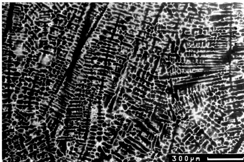
Figure 4: Columnar part of the structure (50X) of 1.4852.
