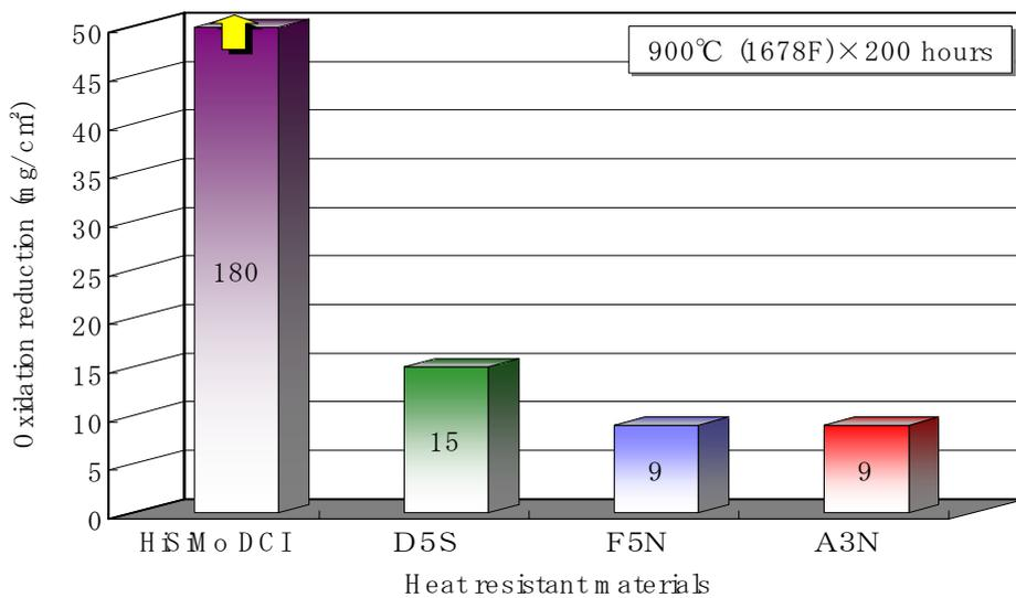
Figure 5: Comparison of oxidation reduction of each tested material as given in Table I.
