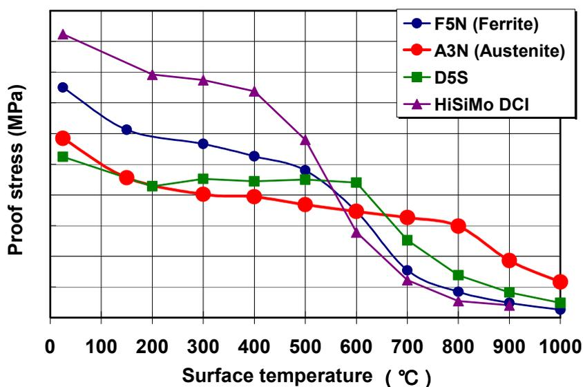
Figure 2: The proof stress (MPa) at temperature of the material given in Table I.
