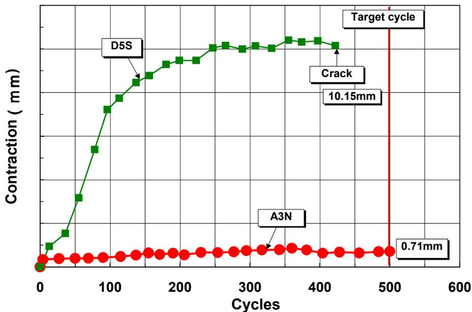
Figure 7: Difference of contractions of the exhaust manifolds made of D5S and A3N during the durability test at 900°C (1678°F).
