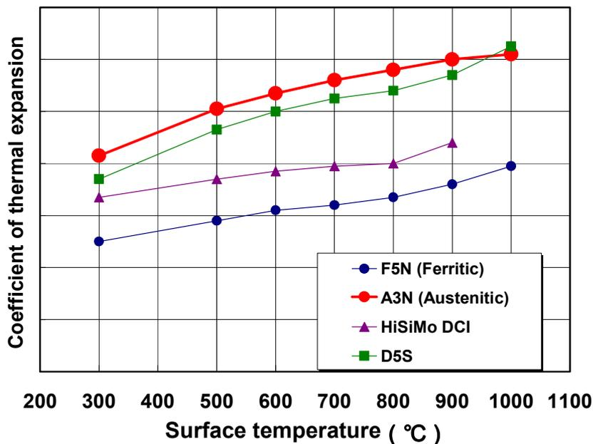
Figure3: Coefficient of thermal expansion of the materials given in Table I.
