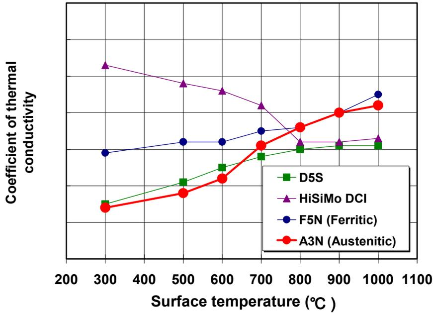
Figure 4: Coefficient of thermal conductivity of the materials given in Table I.
