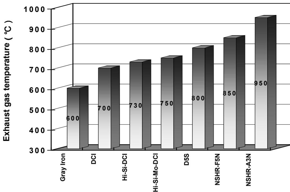
Figure 1: The development of heat resistance materials for high temperature exhaust gas systems.
