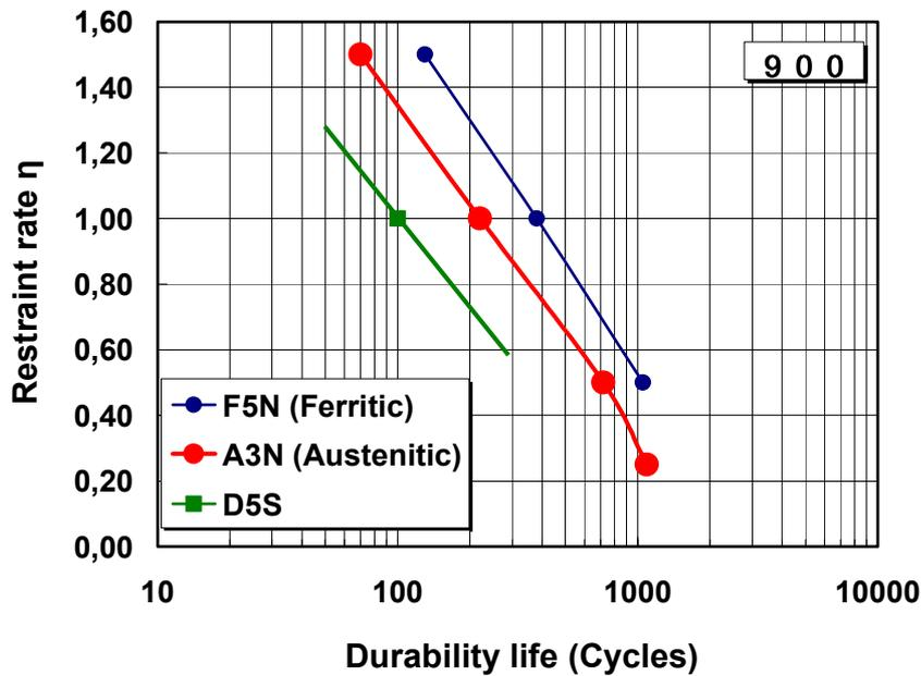
Figure 6: Thermal fatigue properties of 3 of the material tested at 900°C.
