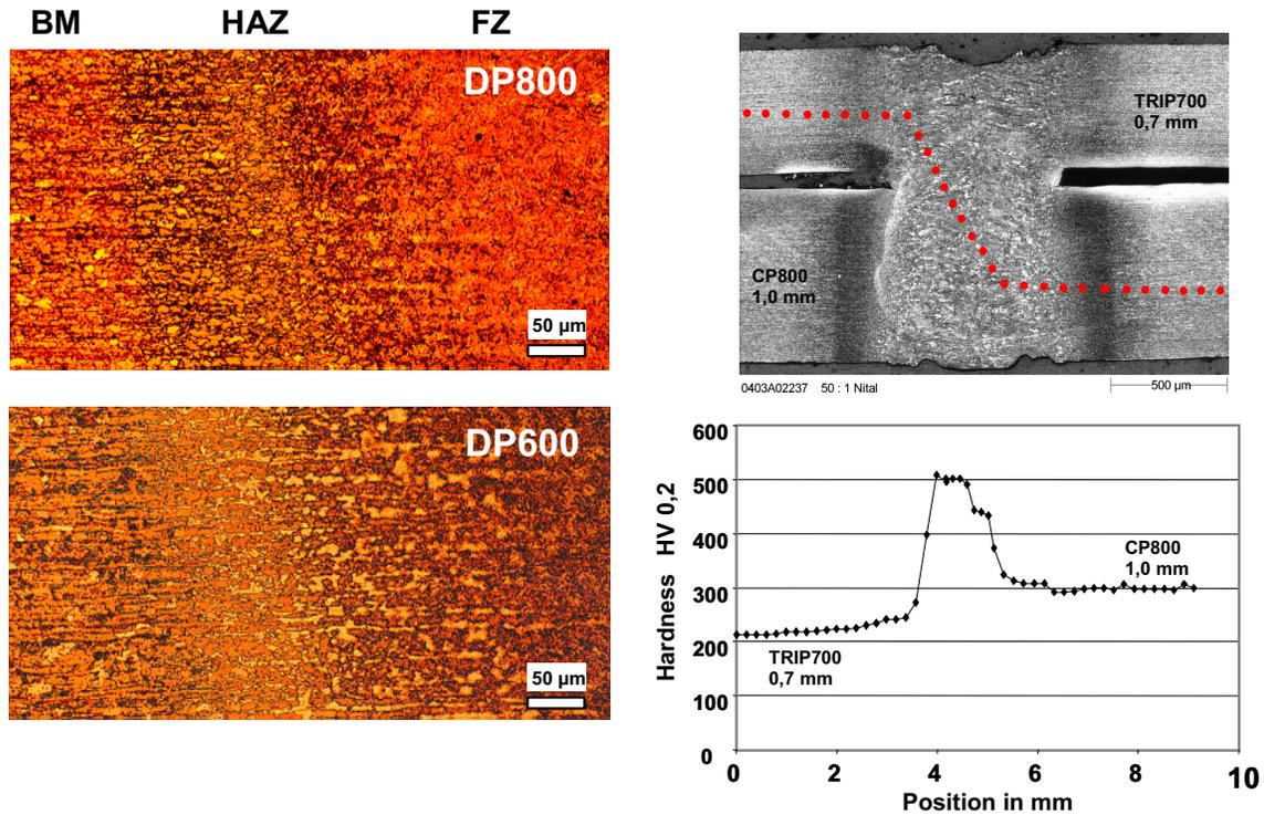
Figure 12. HAZ of laser welded dual phase steels (a) DP800 and (b) DP600; light phases are martensite, dark phases are tempered martensite. Laser overlap weld between TRIP700 and CP800 (c) and hardness scan across the overlap weld (d).
