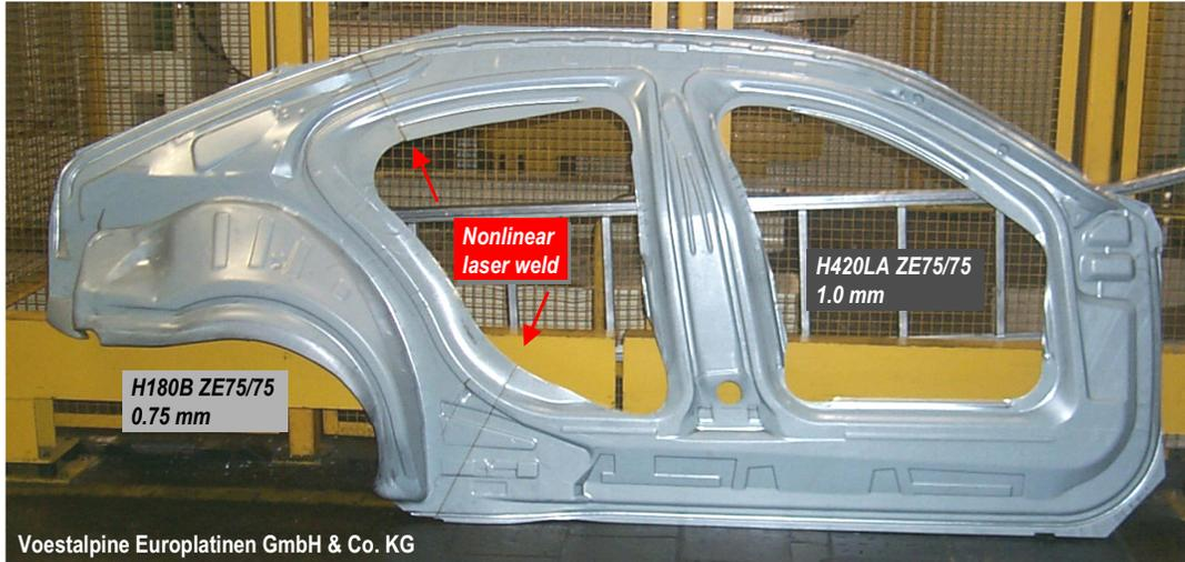
Figure 16. Example of an integrated body side inner panel of the BMW E65 (7-series) using a non-linear laser welded blank consisting of BH steel (YS: 180 MPa) and microalloyed high strength steel (YS: 420 MPa). Blanks are stamped as two per hit (LH & RH side) on a 9,500 t transfer press.
