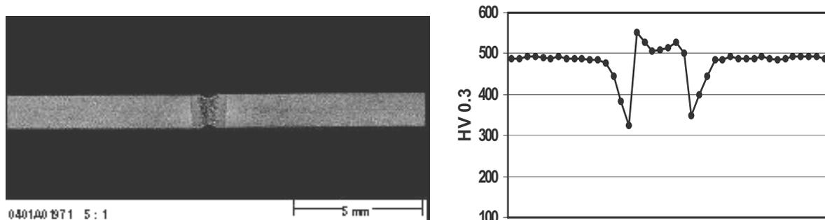
Figure 13. Hardness scan across a laser weld seam applied to hot forming steel (22MnB5) after quench hardening.
