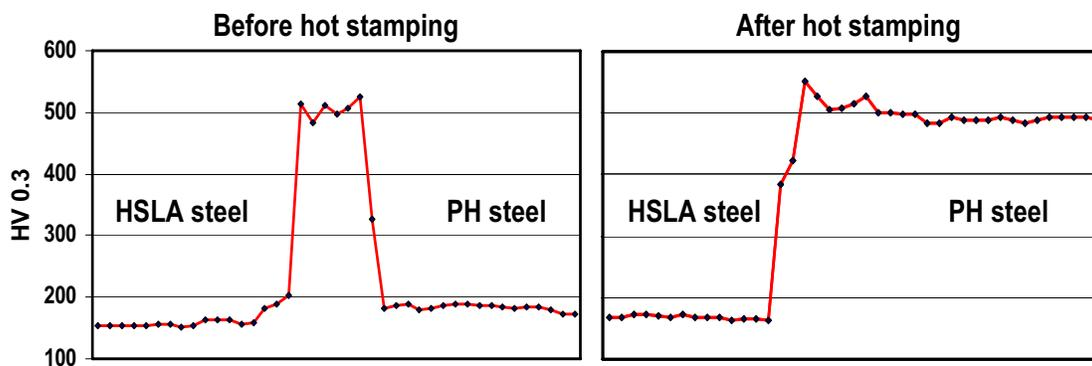
Figure 15. Hardness variation in a laser welded blank consisting of a low carbon HSLA and a press hardening steel before and after hot stamping.
