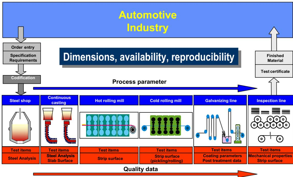
Figure 18. Process parameter and quality monitoring along the process chain for automotive flat steel products.
