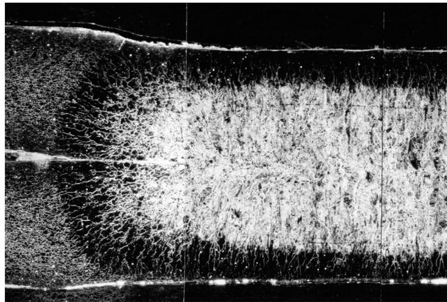
Figure 11. Ultra low carbon corner of the iron-carbon phase diagram indicating the region of effective  $\alpha$ -grain growth. Grain coarsening in the heat-affected zone of titanium stabilized IF mild steel after resistance spot welding.
