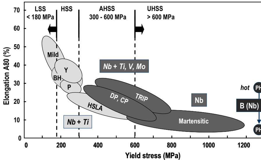
Figure 2. Stress-elongation diagram showing the different automotive steel families and typical microalloying elements contained.
