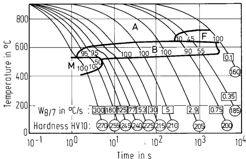
Figure 14. Transformation behavior for simulated HAZ (peak temperature 1350 °C) of HTP steel (0.03 %C, 0.10 %Nb, 1.75 %Mn).
