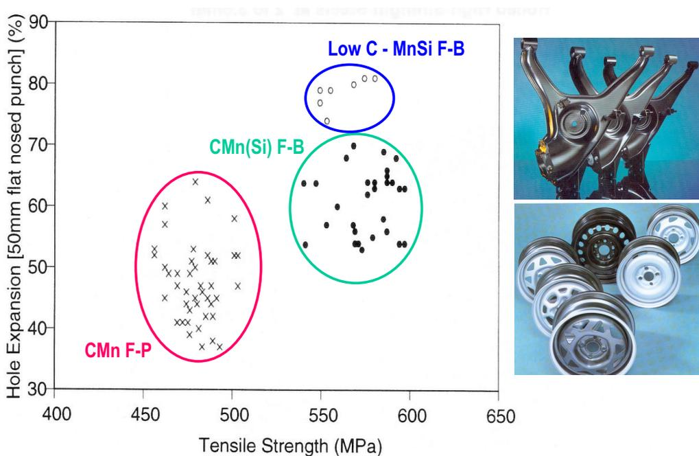
Figure 9. Relationship between hole expansion ratio and tensile strength for various steel types (F-P: ferritic-pearlitic, F-B: ferritic bainitic) and typical applications.
