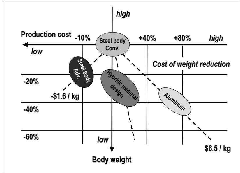
Figure 3. Impact of material concepts on the weight and cost balance of a car body.
