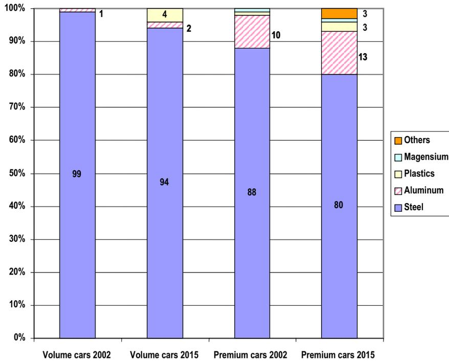
Figure 4. Evolution of material weight share in the body-in-white in volume and premium cars [5].
