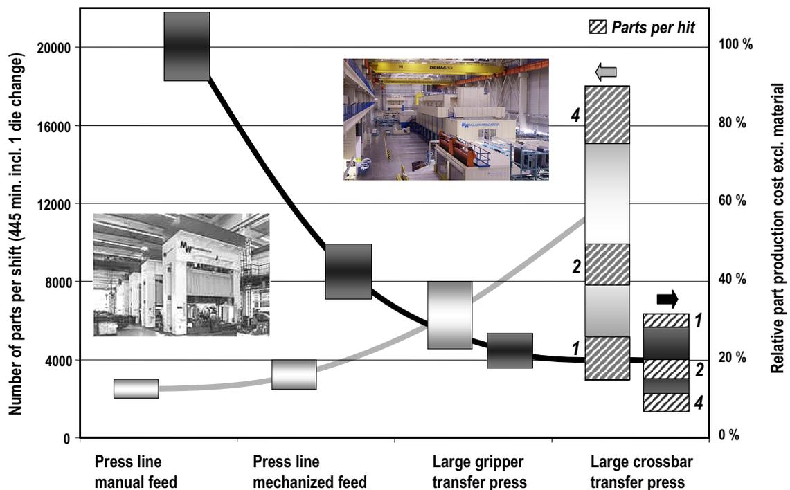
Figure 17. Performance and part production cost of different press line systems [39].
