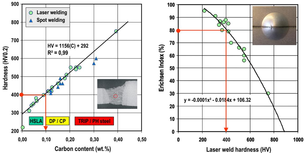
Figure 10. Relationship between carbon content and weld hardness in automotive steel after laser and resistance spot welding (left). Correlation between weld ductility and weld hardness after laser welding evaluated by Erichsen cup testing (right).
