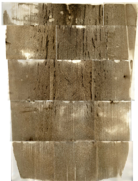
Figure 2. Sulphur-print of an ingot of the dimension 746x1089x1700mm [1].
