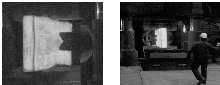
Figure 7. The forging operation.
