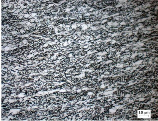
Figure 8. Optical microstructure of multi-phase X100 based on low molybdenum (0.275%) higher niobium (0.08%).
