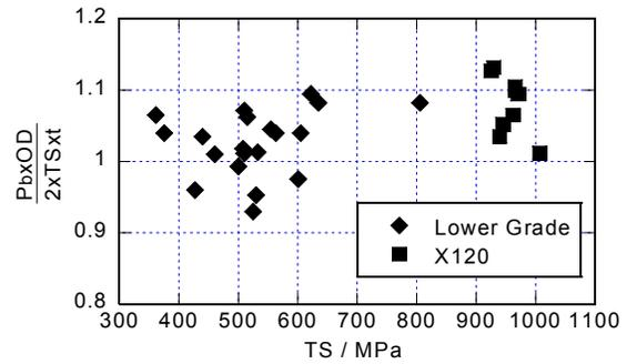
Figure 16. Normalized values of burst pressure as a function of TS.
