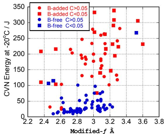
Figure 6. Effect of alloy system on relationship between  $\beta$ -value and CVN energy at -20°C of simulated HAZ.
