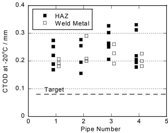
Figure 15. CTOD test results of seam weld centerline and HAZ (shallow notch, 36"OD-16mmWT)
