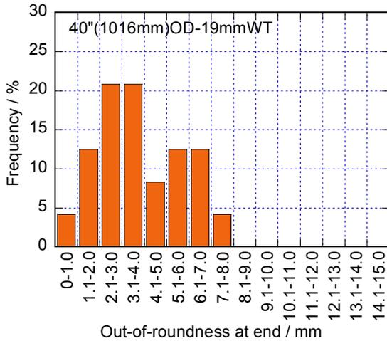
Figure 12. Out-of-roundness distribution of 40”OD-19mmWT pipe during trial production.
