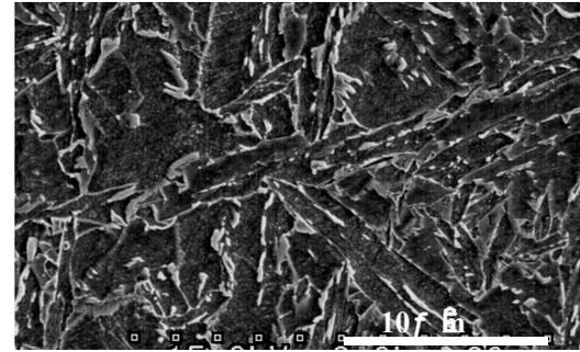
(B) Weld metal ( Degenerated Upper Bainite )
