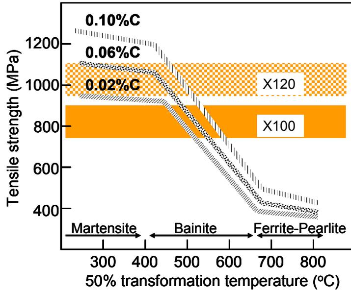
Figure 2. Schematic illustration showing the relationship between transformation temperature and tensile strength
