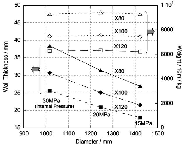
**Figure 1. Change of strength and weight by pipe strength (constant transportation volume)**
