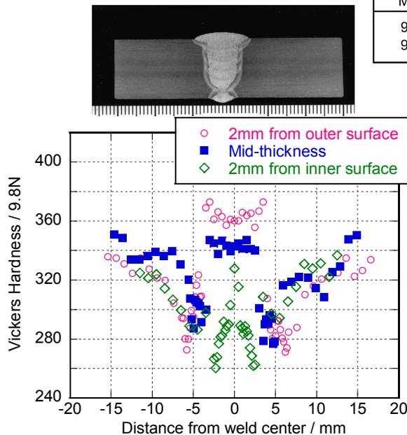
**Figure 17. Hardness distribution in girth weld.**
