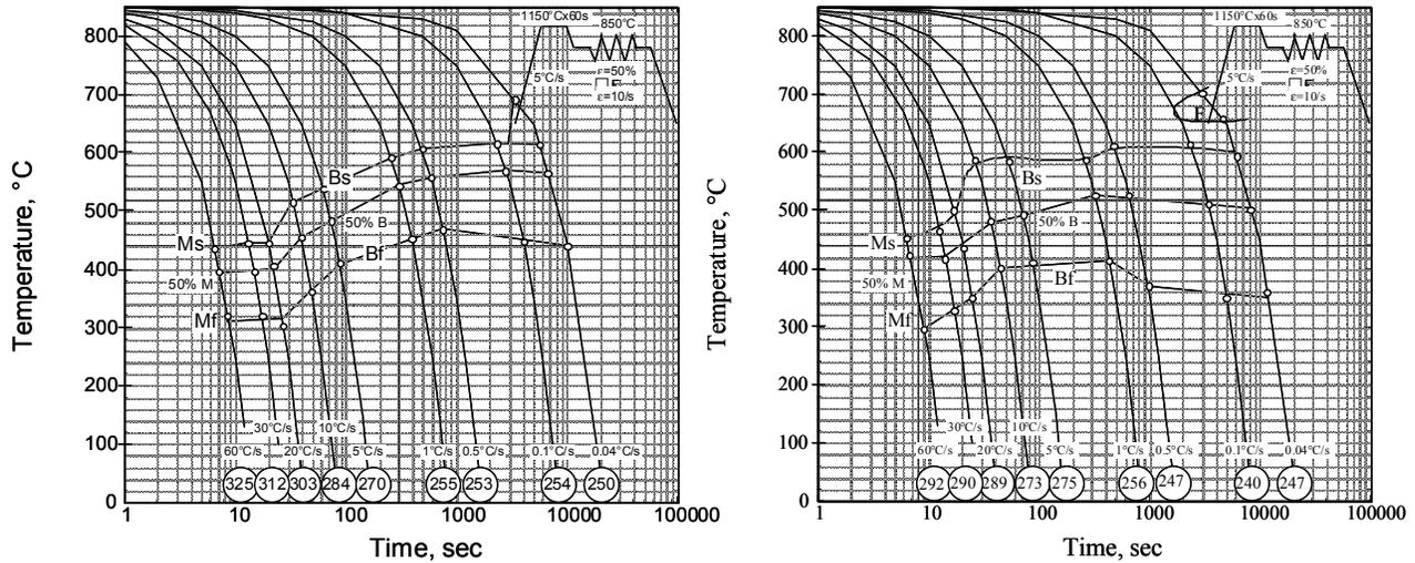
Fig. CCT diagram of LLY-3(0.035% C) steel.
