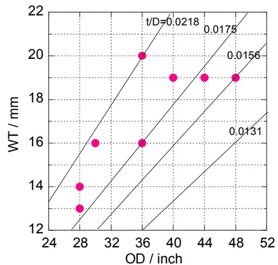
Figure 11. Sizes of pipes produced for testing.
