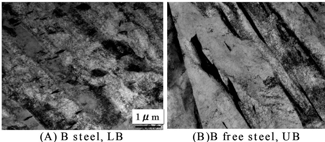
**Figure 7. Transmission electron micrographs of simulated HAZ microstructure**
