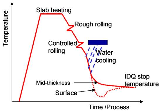
Figure 3. Interrupted direct quench (IDQ) process.
