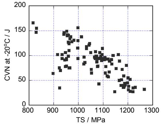
Figure 13. Balance between TS and CVN energy of weld metal produced by SAW.
