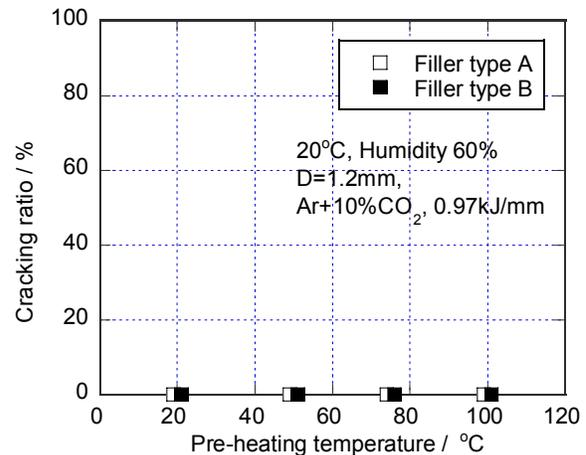
Figure 10. Results of y-groove weld cracking test. (TS of A =956MPa, TS of B = 993MPa)
