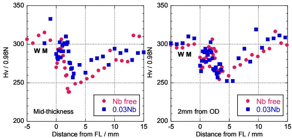
Figure 8. Effect of Nb on trans-weld hardness distribution
