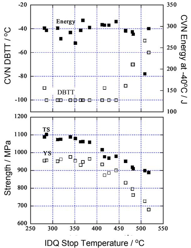
Figure 4. Effect of IDQ stop temperature on strength and toughness.
