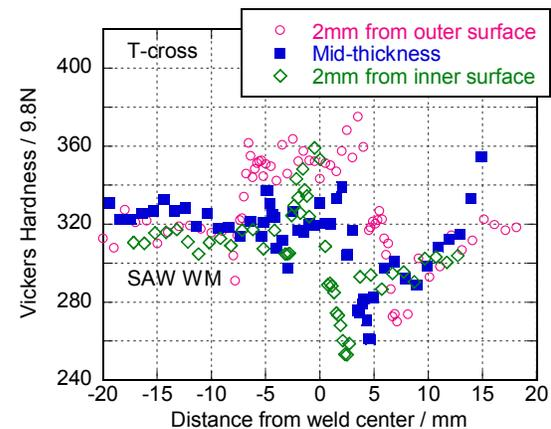
**Figure 18. Hardness distribution in T-cross.**
