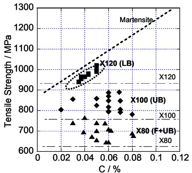
Figure 9. Effect of carbon on tensile strength for martensitic, X120, X100 and X80.
