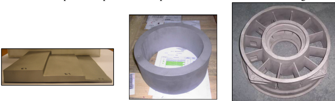
Figure 6: Stair shaped cast plates(left); hollow cylinders (centre); democast (right).
