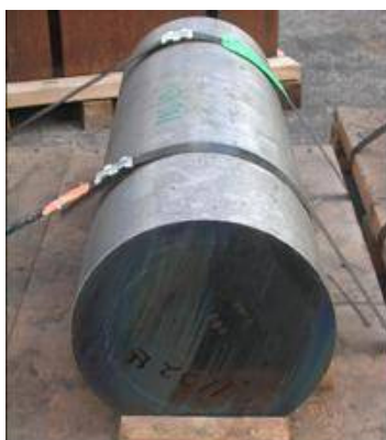
Figure 1: 304.8 mm billet used for production of forged rings at Forgital.
